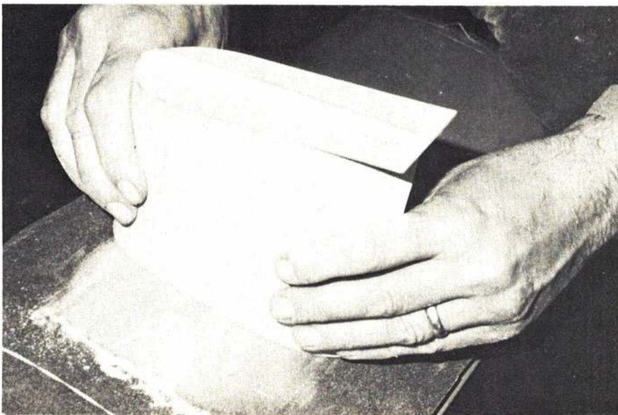
Above: Foam float is easy to make with a band-saw or hot wire. Plank it with balsa or fiberglass and epoxy. Below: Tip floats attach directly to wing bottom surface. Here sandpaper on the wing helps contour the float for a perfect fit.
