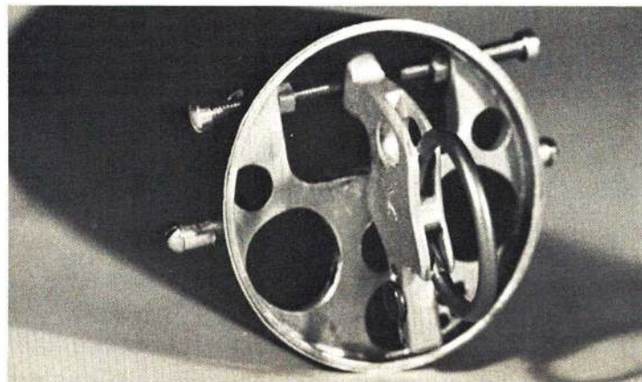
Above: The blades were computer designed! Plans give all stations of airfoil and shape. Left: Torque in the rubber twists a music wire shaft. That's the rubber anchor end with its two screw adjustments on top. During power burst, stabilator is tilted down slightly and more right rudder is applied.
