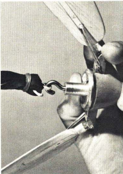
Left: All parts of the prop hub are machined, shaft turns on two ball bearings. Below: Front end uses popular Montreal-stop utilizing the lock-pin as a "waiting for air" safety device. Pushed in, the prop is locked so it is pulled just before launching into that perfect thermal.
