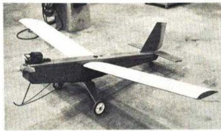
All-metal modified "Bikini" drone used in the WPAFB Project Teleplane weighs 45 lb. and is powered by a 4 1/4 hp McCullough ignition engine. Kraft dual-conversion radio tolerates the ignition noise with no problem.
