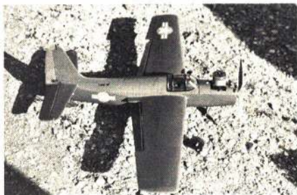
XBTF2-S Guardian by John Mangino seen at Arizona Regional meet is the particular version of this aircraft which had only one rudder. Note pushrod to the rudder for line tensioning. O.S. power.
