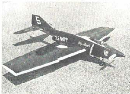
Overall view of Phantom shows mirror-like finish and built-in leading edge steps.
