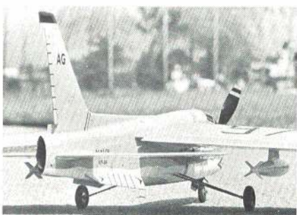
Rear view shows wing's anhedral, unusual ventral fins, drop tanks and rockets.
