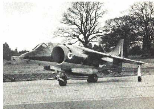
Huge air scoops feed the 19,200-lb. thrust Bristol Pegasus. Top is supersonic.
