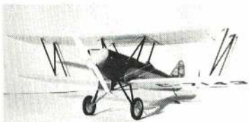
Shock-absorbing landing gear on Indoor Eagle Rock Bipe. Structure is nearly scale.
