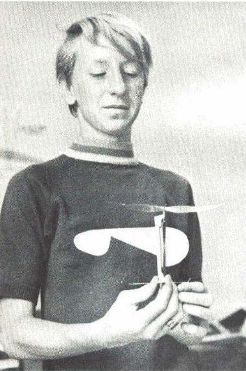
Using an extended Sleek Streak prop as a rotor, Marque Provart makes 10- to 15-second flights with this Minicopter.
