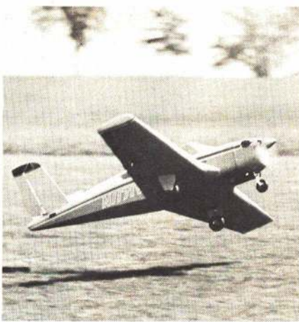
Left: Taking off in a snappy climbing turn is the V-tailed Bonanza. Below: Ready to taxi out, the Debonair responds to gently advancing throttle. Except for tip shapes, tail surfaces and rear window outlines, the two craft are basically similar.
