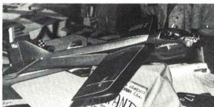
The Rampant by Jerry Worth uses tandem or bicycle landing gear with wing tip skids.
