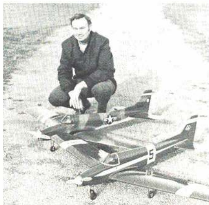
Plane on left has fiberglass fuselage, retracts, acrylic lacquer. Other, enamel; follows plans.
