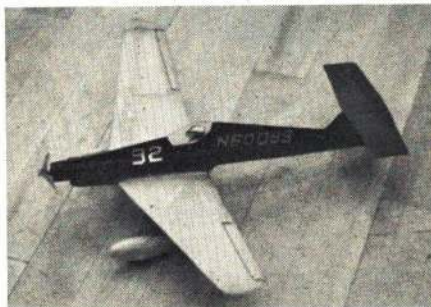
That's a round-the-pole speed model of the Rivets. Model is rubber-powered and did all of 18.7 mph for Rich Castle.
