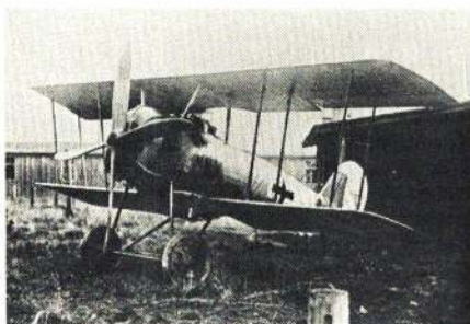
A production D.VIII abandoned by the Germans. Reportedly "pleasant to fly," double-bay construction gave greater rigidity.
