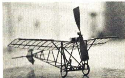
That's a round-the-pole speed model of the Rivets. Model is rubber-powered and did all of 18.7 mph for Rich Castle.
