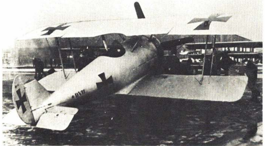
Predecessor to the D.VIII was this single bay strut D.VII entered in the January 1918 Fighter Competitions. (Builder's Note: Cross Patee began to phase out in late March 1918.)
