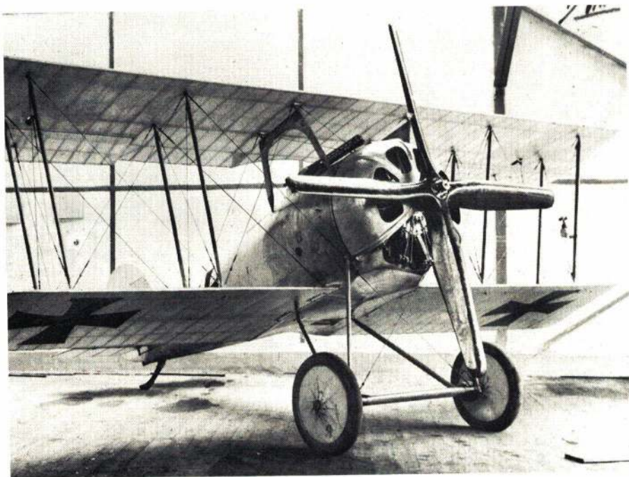
A brand new D.VIII in standard factory finish (aluminum dope). Type-tested in January 1918, production models carried a 160-h.p. Siemens-Halske, 11-cylinder, geared rotary. The propeller revolved at 900 rpm counter to the revolving (also at 900 rpm) crankcase and cylinders.
