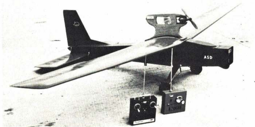
Air Force project "Praeire" aircraft. Designed for target marking, was preceded by feasibility demonstrations in Teleplane program.
