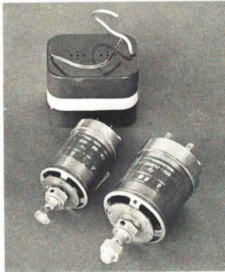
Above: Galler Industries takes a special wound slot-car type motor, gears it, and drives a 10-6 wood prop from a fairly small battery pack. It is a lightweight system and not complicated. Several accessories are available to operate the unit with RC or a timer. Right: From Astro-Flite comes this neat reworked high-performance motor for direct driving standard gas engine type props. Two sizes, smaller unit produces 1/10th hp at peak of battery charge—quite powerful! Larger motor gives 1/4th hp!
