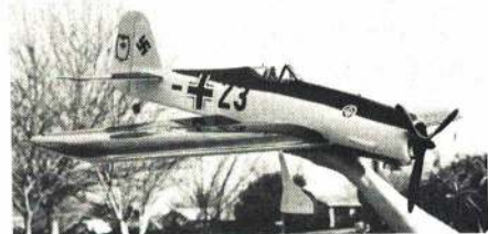
Semi-scale FW-190 by Mike Guthompson is ST 46-powered and spans 57 inches.
