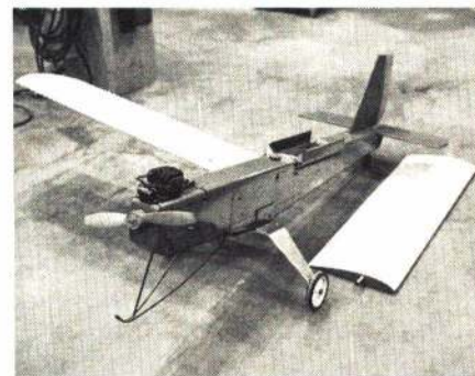
Above: "BOB" is a highly modified 11-ft. span bird used in early RPV experiments and for laser target marking tests. Left: Ross four-cylinder motor powers this heavy "Big Daddy" model. Below: Modified "Bikini" all-metal drone with 4.5 hp ignition motor is flown with Kraft dual-conversion radio. Flown at 44 lb.
