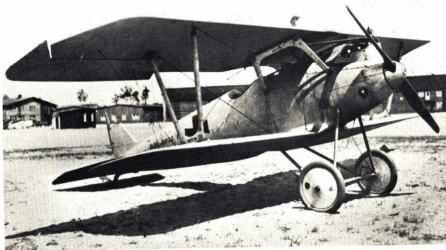
Pfalz D.IIIa (Serial 6033/17). The vertical fins of the Pfalz D.III and IIIa aircraft were integral to the fuselage. An inverted airfoil on the tailplane gave more rapid dive recovery. (Builder's Note: All struts carry aircraft serial number.)
