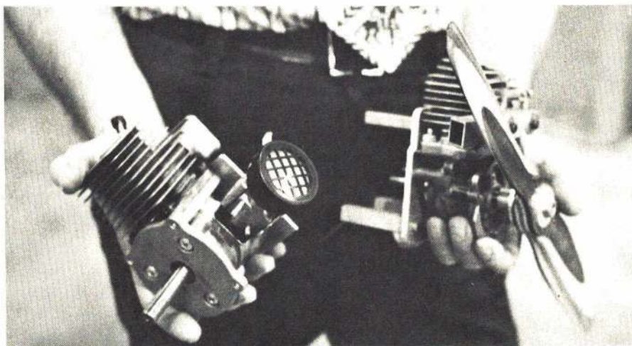
Above: Small industrial engines have been used. At left, a stripped-down O&R two cu. in. engine, and at right a 2.7 cu. in. engine. Right: Best power-to-weight engine is this 12 hp McCollough go-kart motor for use in the full-size 200-lb. "Eagle" RPV. Below: Modified "Bikini" drone servos are equipped with beefed up World Engines amplifier. Gives tremendous thrust and speed.
