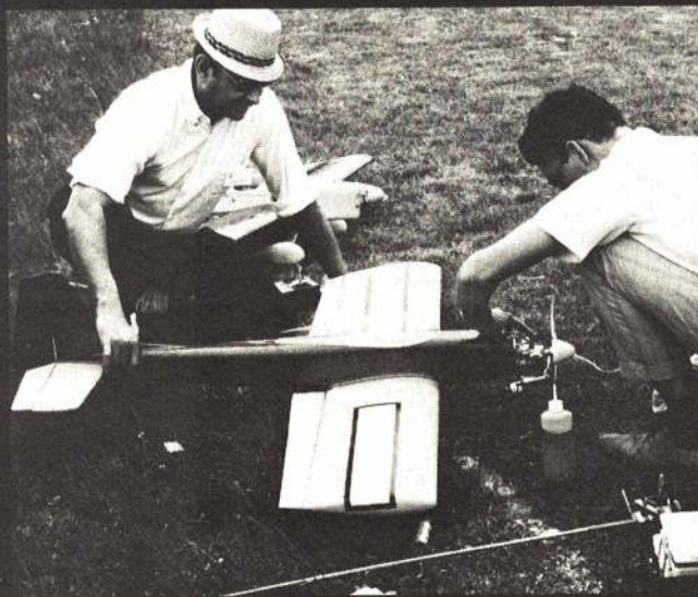
Ed Sweeney starts Kronk Twin-powered Kwik Fli which has reflex trailing edge flaps and ailerons. Not only do the flaps sharpen the plane's square maneuvers but also tamed the stall and significantly slowed the landings. Ailerons much smoother.
