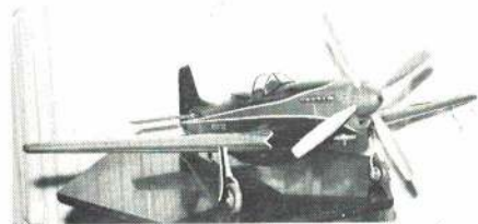
Jerry Farr's 1'-1" Mustang has working flaps, throttle, and K&B 35 power.
