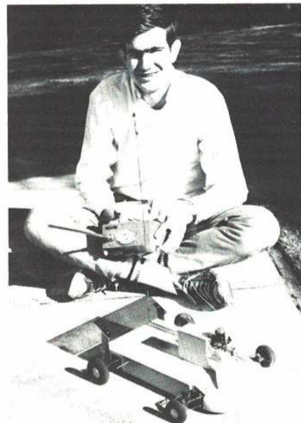
Steven Root tests RC gear on air car. Uses deflector for downforce, has full suspension.
