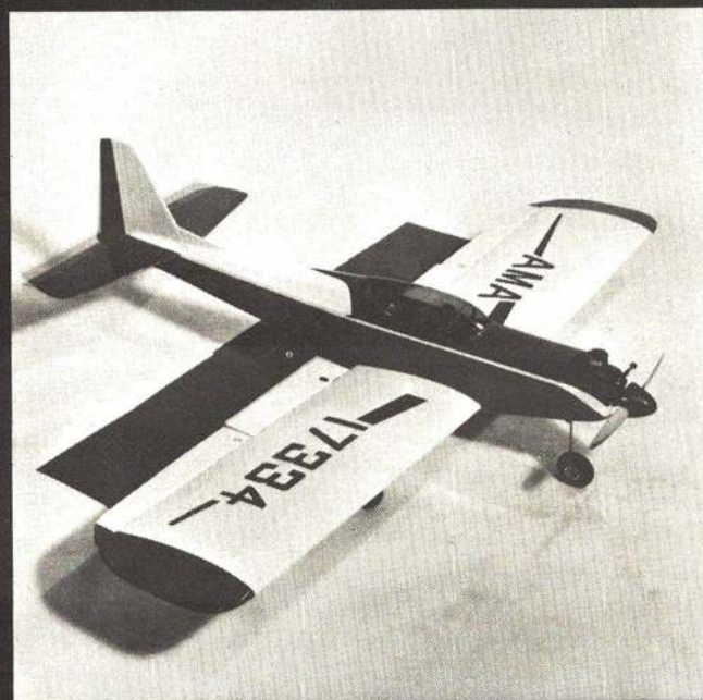
Ed Sweeney starts Kronk Twin-powered Kwik Fli which has reflex trailing edge flaps and ailerons. Not only do the flaps sharpen the plane's square maneuvers but also tamed the stall and significantly slowed the landings. Ailerons much smoother.
