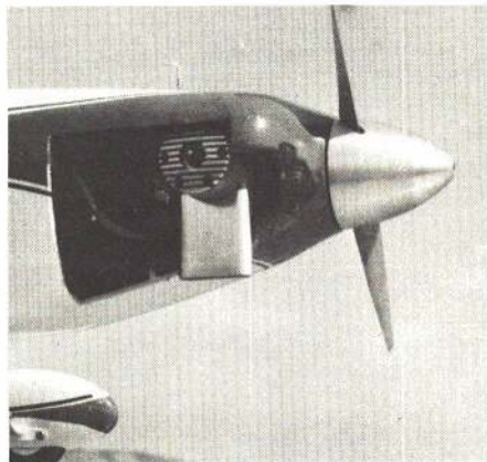
Not having cheek cowl, engine is lost in fuselage. Exhaust extension is essential.
