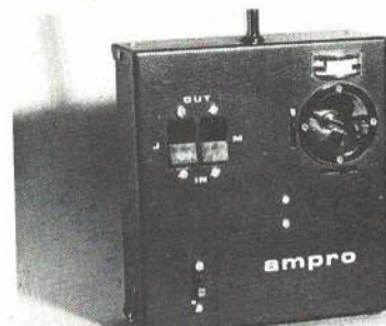
The AMPRO modification of a conventional 3-channel transmitter with rocker switches for main and jib sheets. See text for details.
