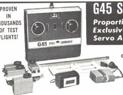
Equipment shown came out of a Testor's ready-to-fly RC Skyhawk. Range is excellent and magnetic actuator powerful enough for Capstan's big rudder. Small digital could be used, too.
