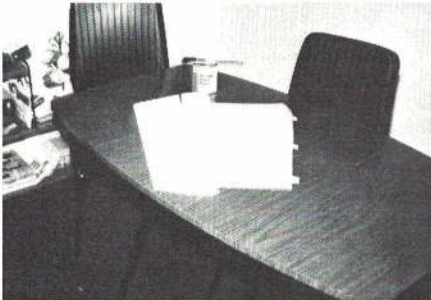
Mylar covering taped to table, contact cement is set.
