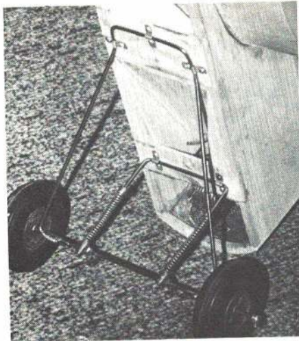
To help earn maximum landing points, Mark finds a simple shock absorbing gear useful.
