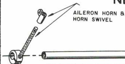
TORQUE TUBE TORQUE TUBE BEARING 2 REQ. ONE EACH END
