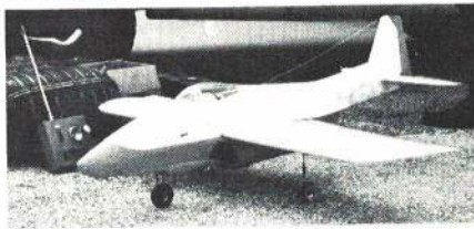
Pulse jet-powered, retract gear design by "Doc" Martin of Houston is not throttled but carves nice big maneuvers in the sky.
