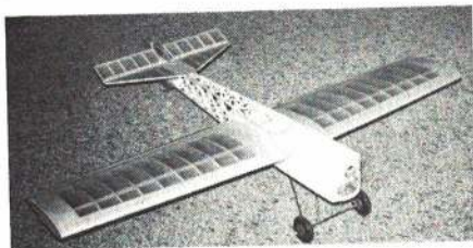
Mark Bauer's latest old-time stunt model now fitted with adjustable features a la Al Rabe and a ST 40.
