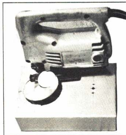
ABOVE: Cut out a hole for the milliammeter in a metal case (this one from Ace R/C). Three small holes are for slave servo, to indicate wind direction. BELOW: Two completed wind direction and velocity monitoring units. Larger unit houses a barometer, as well as an additional meter for a future project. This case is a discarded "exit" sign box.
