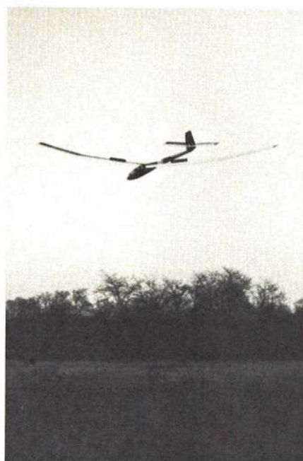
Spoilers deployed, the Astro-Jeff becomes a real target drone, capable of zeroing in on the landing spot.
