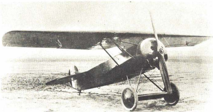
A D. VIII in American colors at McCook Field where it was evaluated by our Air Service. Built in Nov. 1918, the lightweight Fokker tipped the scales at 848 pounds, including its 331-pound Oberursel UR II engine. Gross takeoff weight was 1238 pounds, with 180-pound Lt. Leigh Wade aboard.
