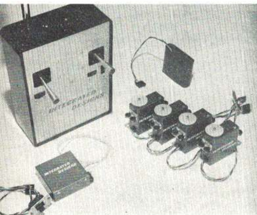
Integrated Designs uses IC throughout and will feature new KPS-11 servos. Low cost.
