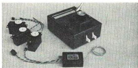
New Orbit RC car radio has exotic transmitter shape for easy use of steering, throttle, and shifting. Frequency changeable at the track by installing different crystals. PS-3 servos used, fast, accurate, and rugged. Note antenna angle.
