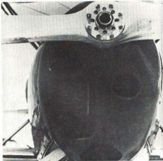
Scale buffs have plenty of intake holes to carve. Inverted engine puts thrust high for a good trim.
