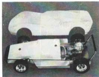
Sharp GT styled body of tough Cyclocac® brand snaps over the chrome plated steel chassis. * Borg-Warner Corporation
