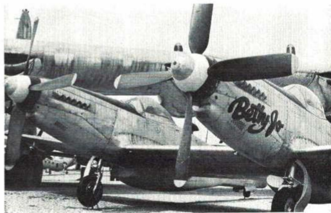
The rare "Twin Mustang" by North American. Not a mating of two Mustangs, F-82 is fully-engineered twin fighter. Only one pilot.
