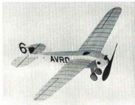
All balsa Avro 560 is ultra lightweight model. Great flyer but tricky on takeoff.
