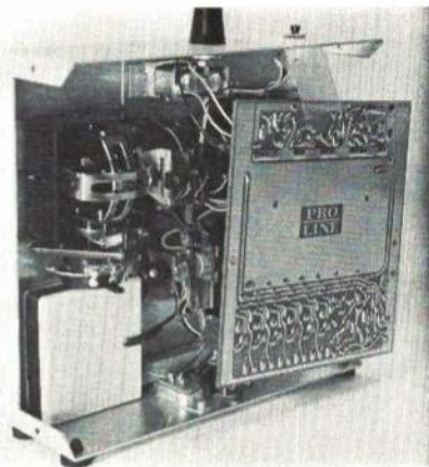
Transmitter uses Kraft-Hayes sticks and other fittings. Neat assembly is evident. PC board is plated and moisture-protected.
