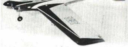
Small European-style stunter, Slicker from Indy RC, uses 15 to 40 engines. 425 sq. in.
