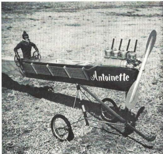
Intrepid aviator views one real, three fake cylinders (hiding fuel tank), and a real Fox 36RC. Landing gear prevents nose-overs.
