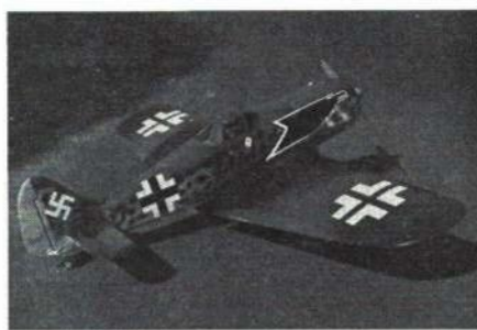
Model features (1) removable foam wing, (2) removable tail surfaces, (3) removable dural gear, (4) radial mounted engine, (5) muffler channelled down fuselage center, Continued on page 78
