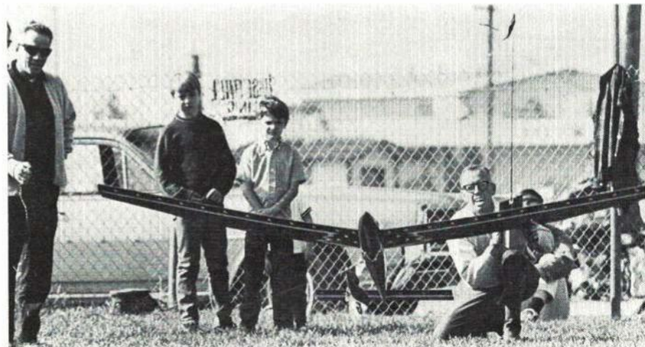
Yankee Wench ROG's while Le Gray rapidly gets hand back to the stick. ROG's are safer. Man at far left holds electric winch button. Cable runs to pulley across field.
