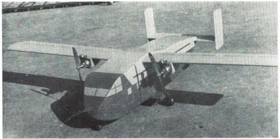
Inexpensive all-cardboard version of Skyvan (AAM Jan. 70) cut out of grocery boxes by W. A. Dahlgren is just as strong and light as balsa version. Uses two Cox or Testors 049's.
