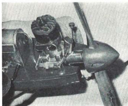
Fuel-line guide by Sal Calato prevents line from being melted by hot engine or exhaust.
