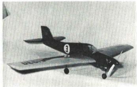
Avenger from Wing has beautiful fiberglass fuselage, foam wings. FAI or AMA versions.
