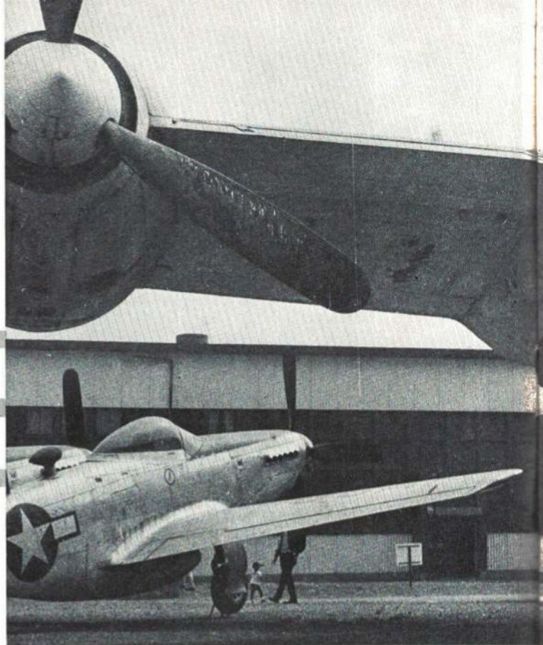
It was impossible to get all of the B-36 in picture frame! Six huge multi-row, "corn cob" radial air-cooled engines, plus four jets, powered the beast. It never fired a weapon or dropped a bomb in anger. Small jet in pix was carried internally as experiment.
