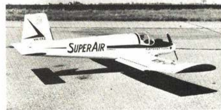
Rear quarter view shows off the simple lines. Flaps down for quick takeoff and steady slow flight when working.
