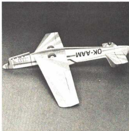
Colored tissue is used for striped patterns, a ballpoint pen draws the lines. The launcher dwarfs the model.
