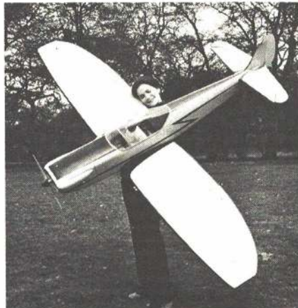
A 1/4 size C.A.P. 20 homebuilt by Lehman uses O.S. 80, weighs 14 lb. and spans 8'.
