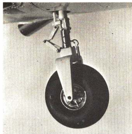
Carefully concealed is a stock Breiten nose gear. Fork built up with balsa, shim stock, and Epoxolite. Du-Bro wheel fits scale.
