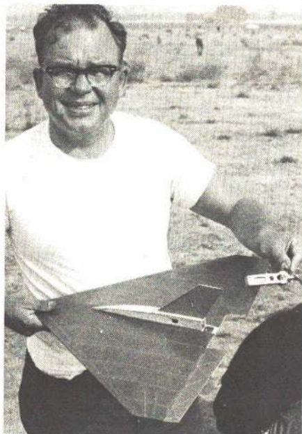
Walt Mooney's delta with removeable CO2 engine mount. Flies two planes with same engine.
