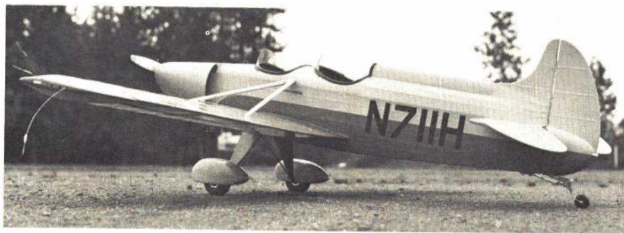
Top: How about that nifty scale tail-wheel? It's worth several scale points. Cockpit is simple—it needs the full pilot and instruments treatment if you can avoid weight buildup. Above: Symmetrical stunt airfoil is evident in this view of the model. What it costs in lost scale points is easily made up by optional maneuvers. Ailerons and rudder are fixed for flight unless you fly it RC.
