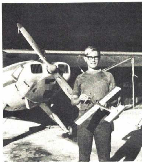
Above: Author is also learning to fly a Cessna 140. Below: Wings in most control line planes don't use dihedral. This model also gets by without real airfoil shape, but it sure flies easily.
