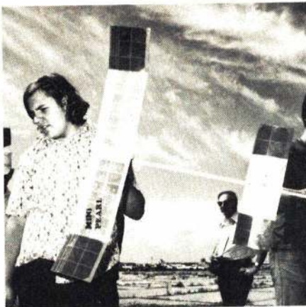
Fuse snug in insulated hole of Ed Taylor's Mini Pearl FF fuselage, above, serves as "snuffer tube" to comply with point 3 of Safety Code FF section. Tom Warden, partly visible at right, cares for lines with the same attention given to constructing and finishing his magnificent CL stunter. It's important for both safety and good control operation.
