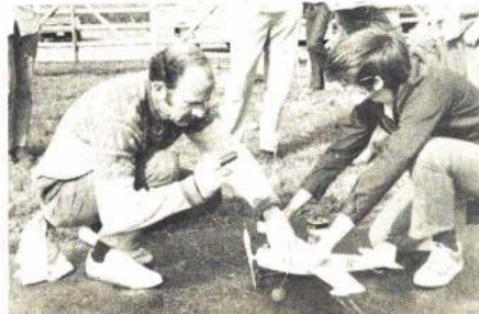
Harry Higley's Mo-Bipe for carrier with ST 35 power has ailerons, auto-rudder, all the necessary gadgets for ultra-slow flight. Very steady, even in a wind.
