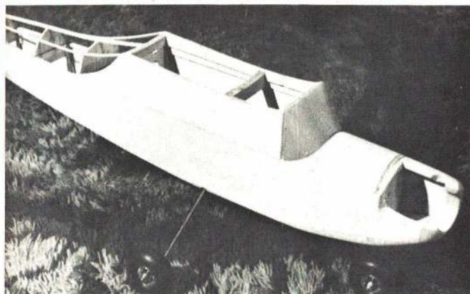
It doesn't take too much time to get the fuselage to this finalized stage. Let the sandpaper achieve those nicely rounded corners.
