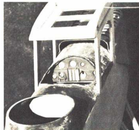
ABOVE: The completed left upper wing structure on its building jig. RIGHT: The fiberglass turtledeck, as installed on the top of the fuselage.
