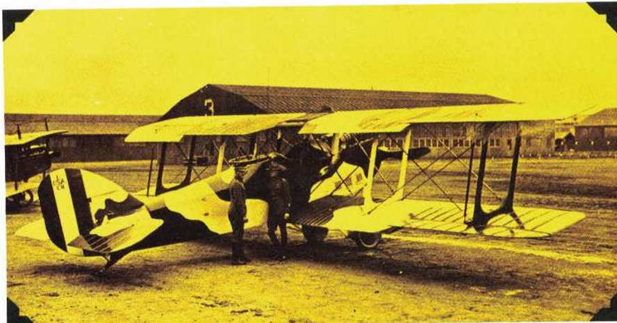
Novel inter-strut bracing gave strength, yet didn't interfere with streamlining.
