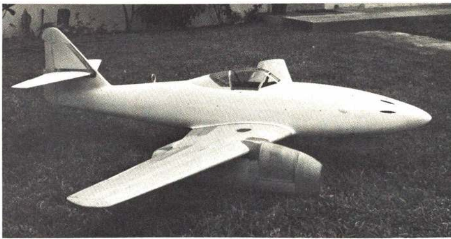
A masterpiece of design refinement, the Me 262 was well over 100 mph faster than Allied fighters in 1944. The fuse is ready for paint here, while the wings will be glassed and resined.
