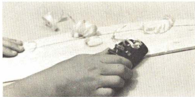
A razor plane saves time, but can cause problems if not properly used. Note that the cutting edge is angled 45° to the direction of the stroke.
