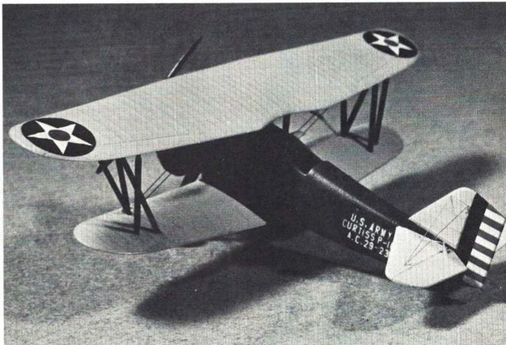
Wing and tail surfaces of P-1C are exactly as on P-6E. Level rear decking and reshaped cockpit opening are made with pieces of scrap styrene. Tail skid replaces wheel.
