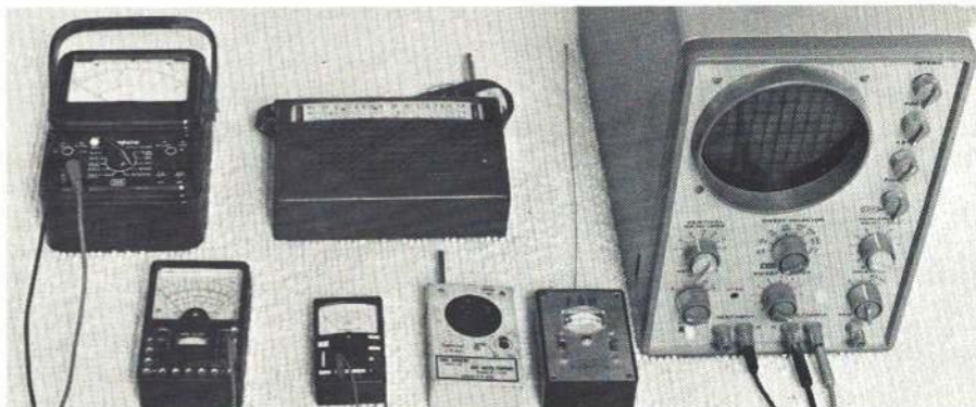
Test gear, left to right: Simpson VOM; inexpensive Aristo VOM; cheap, handy VOM; MRC regen monitor; ACE kit FSM; Eico kit oscilloscope. Center: AM radio required per FCC during Citizen's Band operations. This one also monitors modeling frequencies.
