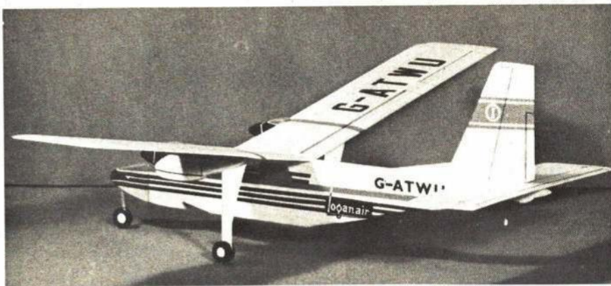
Large fin keeps Islander in the groove during catapult launching. Because of speed of launch, do not alter trim of fin or tailplane. Trim with ailerons only and little bits of clay for weight.
