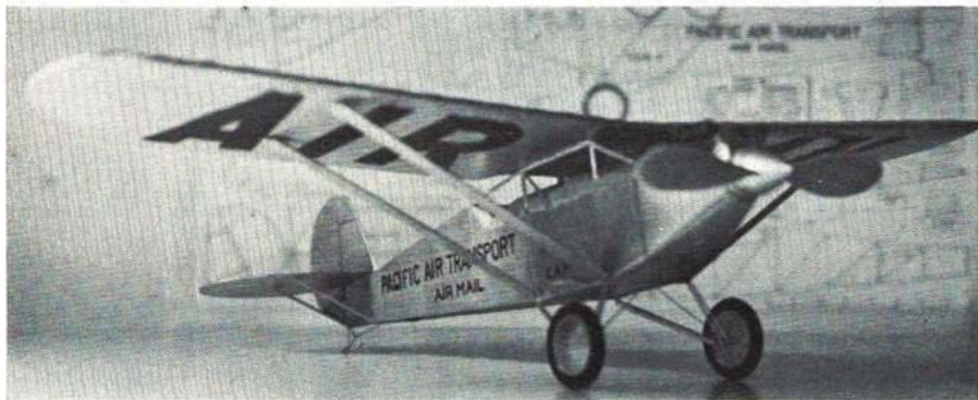
Model's structure features use of card stock, bond paper for wing leading edge, and built-up ribs. All curved outlines are laminated balsa strips. Flies great indoors or out.
