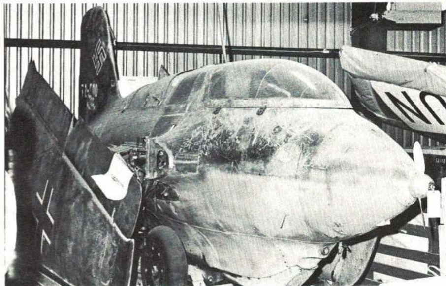
A prize from WW II is this Messerschmitt ME163 rocket-powered interceptor. It was extensively tested at Edwards AFB after the war. One of the most dangerous aircraft ever built, the Komet often exploded on a mild bounce-landing, or on over-running field, after touchy glide to earth.
