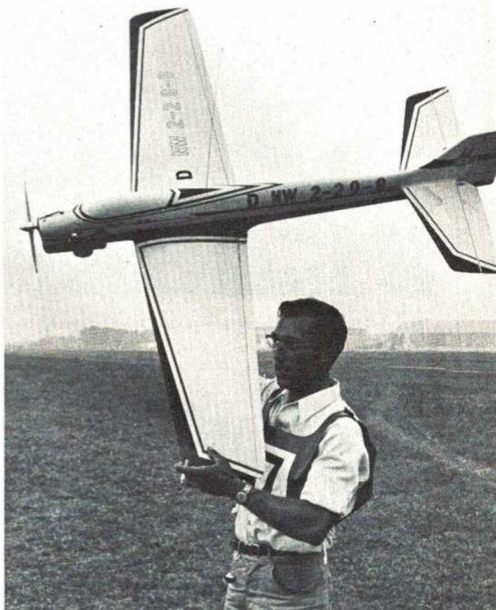
Josef Wester of Germany using Graupner Varioprop radio and ST 60, placed third. In large FAI maneuvers, strip ailerons are favored in Europe.
