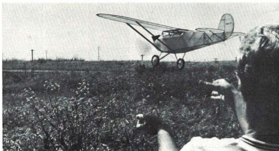
Model's structure features use of card stock, bond paper for wing leading edge, and built-up ribs. All curved outlines are laminated balsa strips. Flies great indoors or out.
