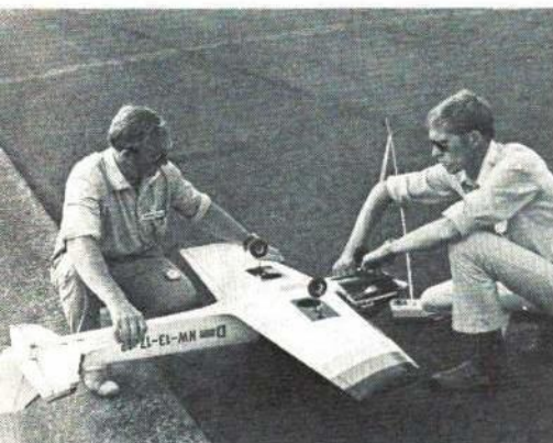
Like winner, W. Schonfeld uses retract gear on "Prestige." Radio is Simprop, S. T. engine.
