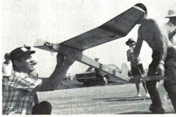
B FF model by Alan Vollmer looks like a low wing, but down angle of surfaces should give high-thrust pylon forces.
