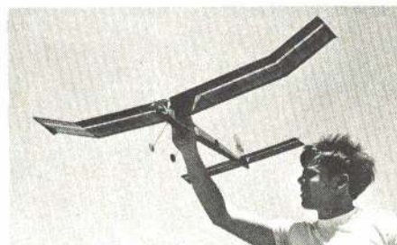
Thoughtfully designed pay load model by Marty Thompson has one-bladed prop, four-point gear, and dropped wing tips.
