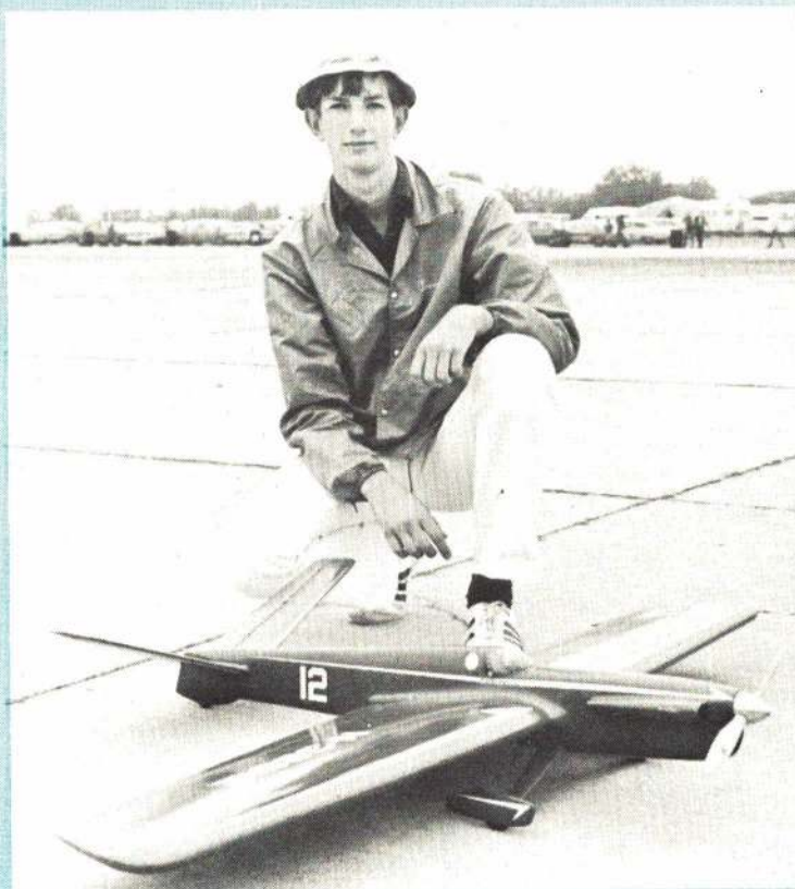
Dennis Adamisin with his V-tailed stunter Sweet Pea. An original design fashioned after the Sky Baby series, it has built-up wing with sheeting, OS-35 engine and 10-6 rev-up prop.
