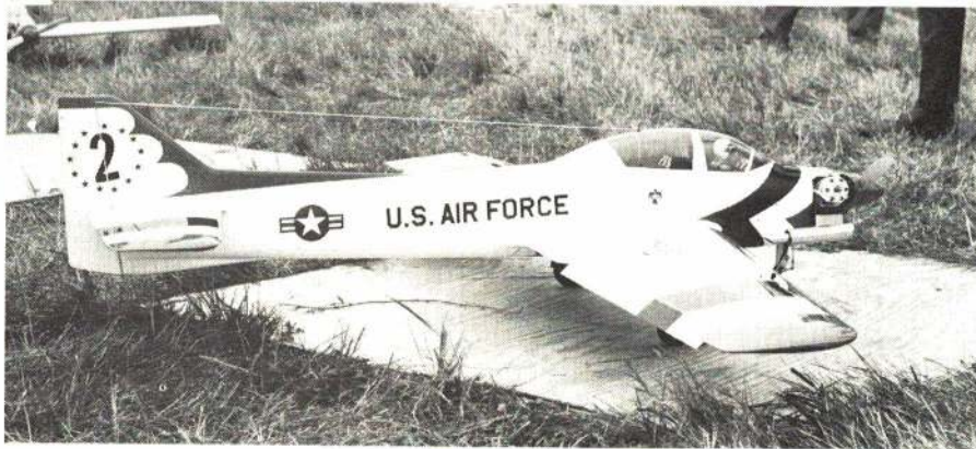
Bob Smith's T-2A designed by Tom Atkins. Bob will kit this ship. Notice the drooped aileron. Ship has coupled ailerons/flaps. Works very well.
