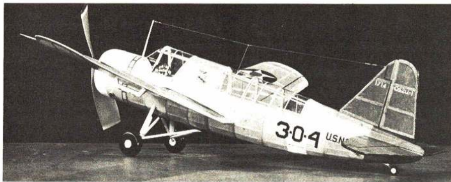
An outstanding example of traditional stick-and-tissue construction, this rubber-powered Vought OS2U Kingfisher, built by Michael Kuehne, flew in the Indoor Navy Scale event.
