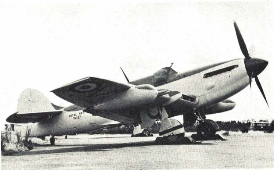
Even with all that drag hanging on the wings, the Firefly was a great performer: Max speed was 386 mph at only 14,000 feet. And it was a heavy plane at 16,096 lb.
