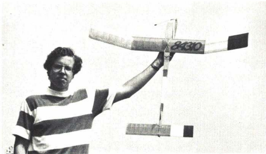
Above: Charles Wiese, Detroit, won Senior Coupe d'Hiver with his simple Maxwell Mk II, his own design. Two-piece wing and detachable tailboom facilitate transportation. Right: Rowena Barron retrieved brother Andrew's Mini Pearl from the cornfield. Below: Lee Campbell made three maxes in the Rocket-Power event, the only one to do so, with his Sundancer.
