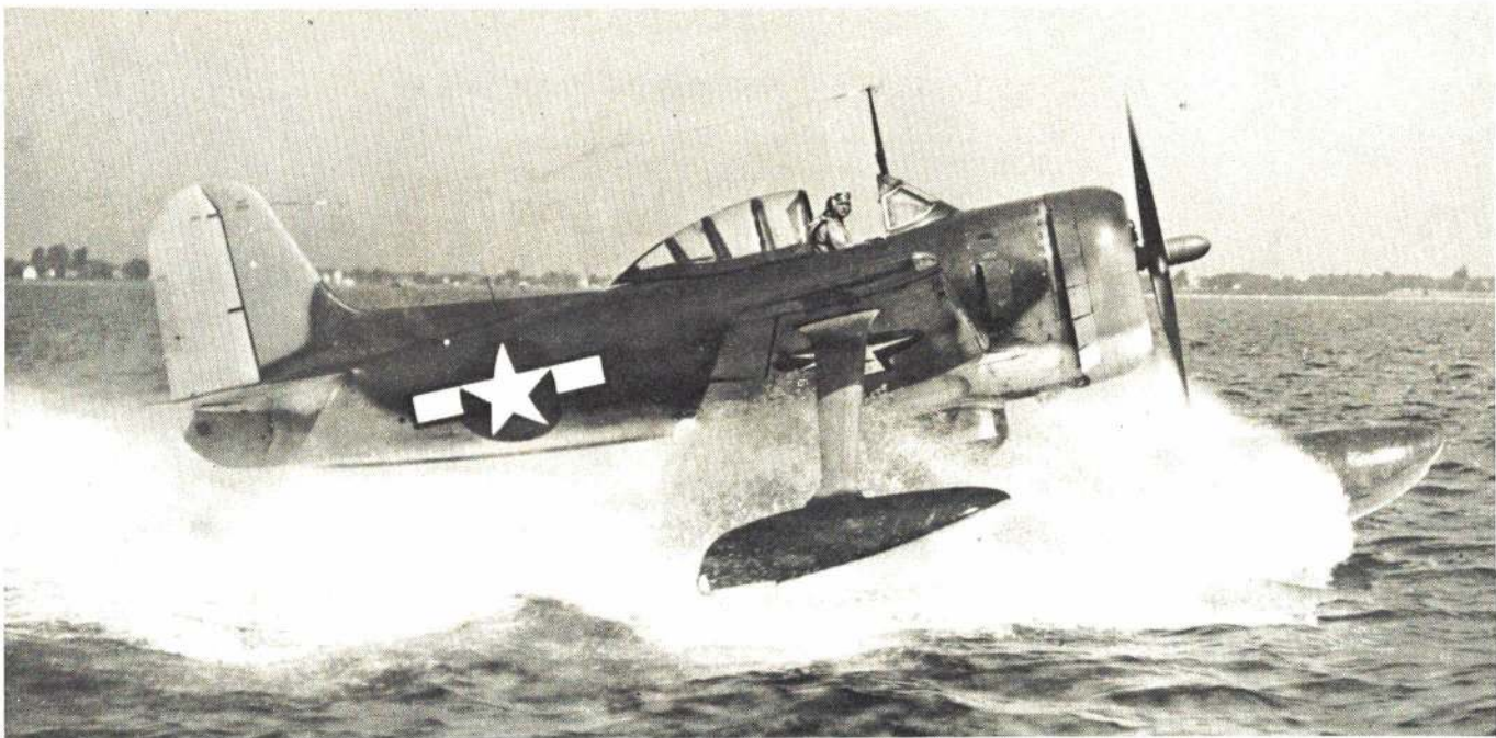
Rugged enough for rough seas, 1350 horses pulled a 4-blade, 10' 2" constant speed prop made for rapid ROWs. (Photo courtesy Smithsonian)
