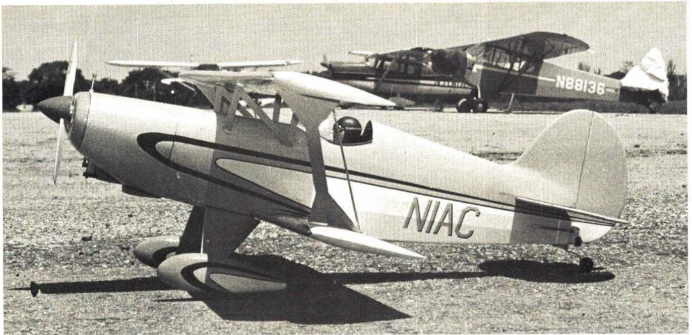
This view gives an excellent angle on those wings, which have a distinctively short chord.
