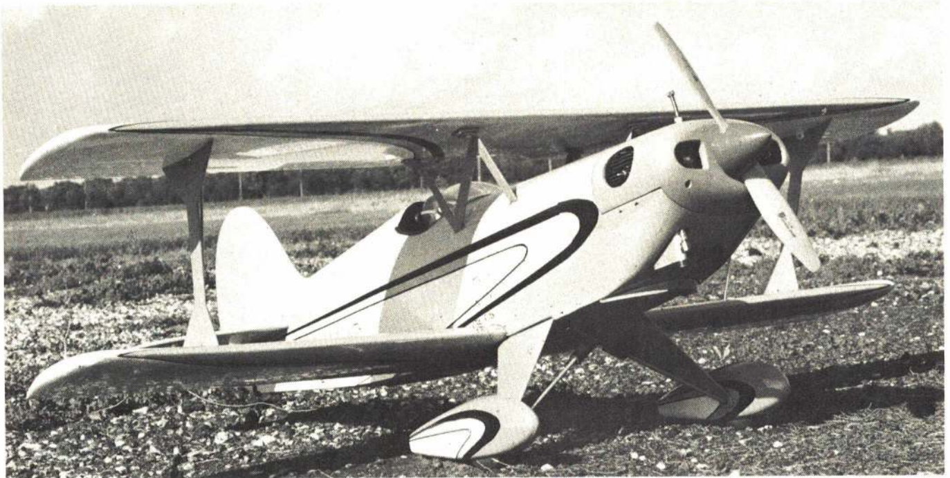
The Acro-Sport's cowl is exceptionally clean, and is uninterrupted by the usual vagaries of an exposed cylinder head. The Du-Bro Muff-I-aire keeps things quiet, yet neat. The nose of a biplane gets lots of attention, so treat it with respect.
