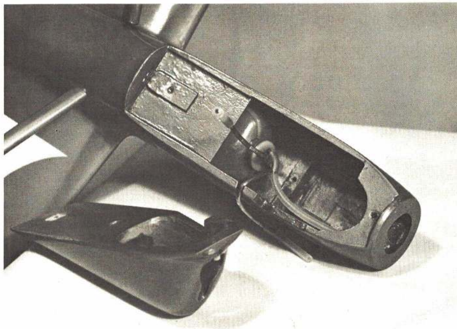
ABOVE: Bottom view of conventional cowling shows mounting and venting of a plastic tank. The tank is secured with foam rubber. BELOW: Removal of tank is accomplished by pulling forward and rotating, after engine has been removed.
