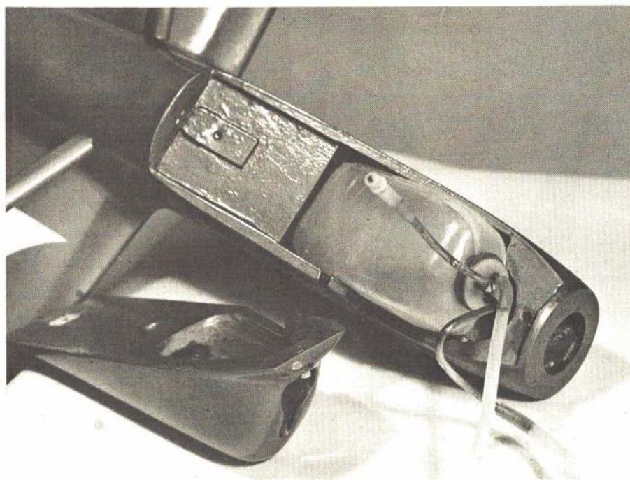
ABOVE: Bottom view of conventional cowling shows mounting and venting of a plastic tank. The tank is secured with foam rubber. BELOW: Removal of tank is accomplished by pulling forward and rotating, after engine has been removed.
