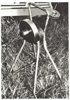
Compact Russian inertia starter had 50:1 gear ratio. Requires assistant to operate crank.
