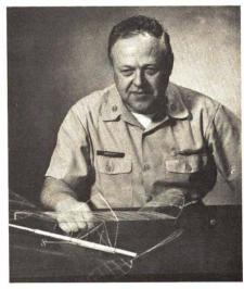
Randolph's model appears to be an adaptation of a Stick model with a "cabin" added to give the required cross-section area. The photo shows the takeoff gear in its retracted position—powered by a single strand of monofiliment nylon. An original design, the model is named Fat Cat IV.
