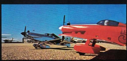
Testors designed their Silver Wind and Cosmic Wind trainers especially to make engine powered, U-control flying easy, fast and fun. Crash proof, virtually indestructible, rubber band assembly allows parts to separate on impact without breakage. They're the perfect planes for new pilots.
