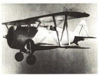
Wheels down to keep formation with a slower camera plane, an early F3F-2 with the then-sensational 1000-hp Wright Cyclone engine.
