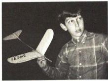
The model, designed by Jean Pailet, has a wing with 16 1/2" projected span and 3" chord; each panel is swept back 15 degrees. The wing is constructed from 1/16" sheet which is then warped to produce 1/16" undercamber; .008" music wire is glued to the wing leading edge for protection against nicks. The stabilizer, 6 1/2" span by 3" center chord, is of 1/32" sheet.
