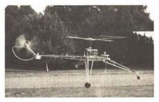
Rock's 'copter flew last August. Enya 45 turns 55-in. rotor. The tail rotor is driven by 40 D.P. timing belts.
