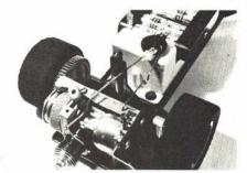
Homemade brake is stiff brass pivoting on screw beside pull-starter and bearing on clutch, Note link to servo.
