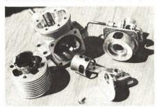
Verbitsky's disassembled engine at FF World Championships; Schnuerle porting, drum rotor, piston ports. Much dental drill work.
