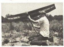
Faulkner's model was designed by Robert Johnson. The wing has 79" span, 11" center chord, 10 percent airfoil thickness. The stabilizer is 36" by 8". Both the wing and stab have multi-spar construction. The overall fuselage length, measured from the firewall, is 50". The model was covered with Sig Jap tissue and finished with Aero Gloss dope; weight was 34 ounces.
