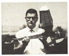
The model which set the record was the Strato-Streak design by Louis Garami published in the December 1941 issue of Air Trails magazine. It was equipped with sled floats for establishing the rise-off-water record. The wing has 39½" span, 6" center chord, flat bottom airfoil. The stab has 18" span and 5 3/8" center chord. The model weighed eight ounces.
