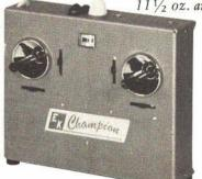
"Amp-Pak" integrates servo amplifier and receiver-decoder. Electronic circuits are proven design made famous by Logictrol. Transmitter and receiver charger built into case. Ni-Cad rechargeable batteries.
