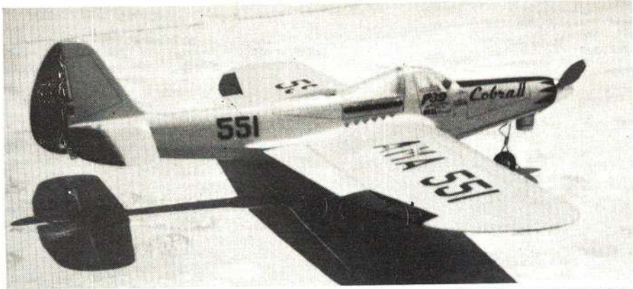
Fox 40 powers this quite real-looking P-39 stunter by Lew Wolard. Unique use of muffler pressure to tank for smooth runs.
