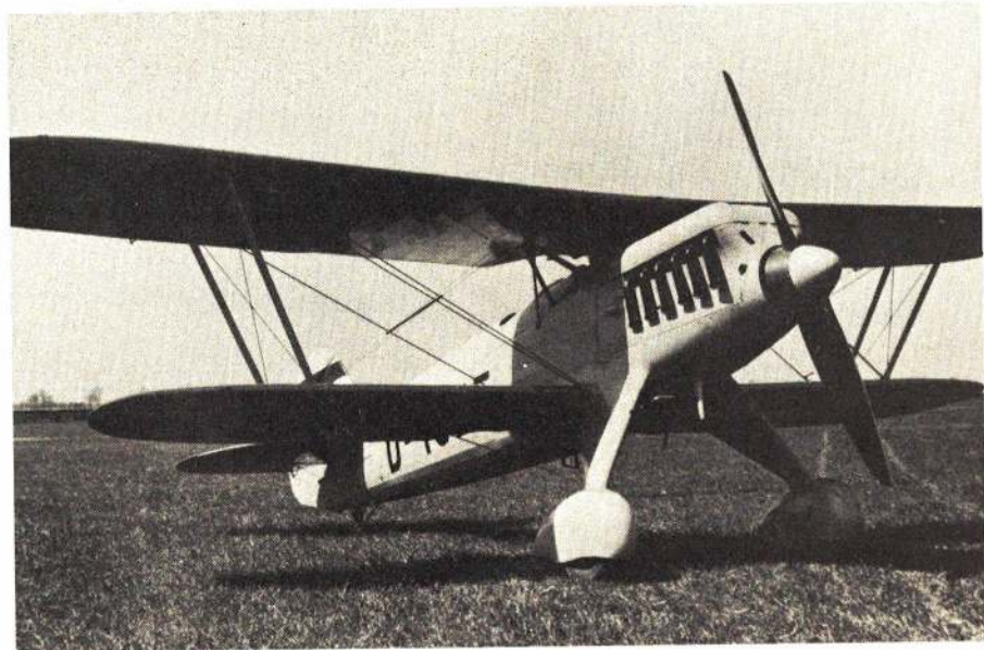
The standard production version of the He-51, showing its unequal-span wings and out-swept interplane struts to good effect.
