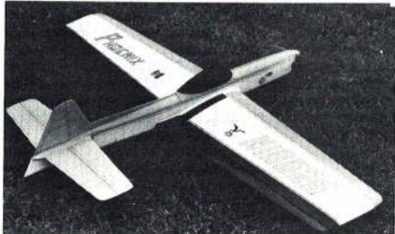
ABOVE: Tom Dixon's Stephen's Akro, 52-in. span, 53 oz. wt., OS 40. Tom is particularly proud of this Akro as it flies circles around his Phoenix. Tom plans a new Akro for next year. BELOW: Dixon's OS 35-powered Phoenix, 55-in. span, foam wing, 52 oz. wt.
