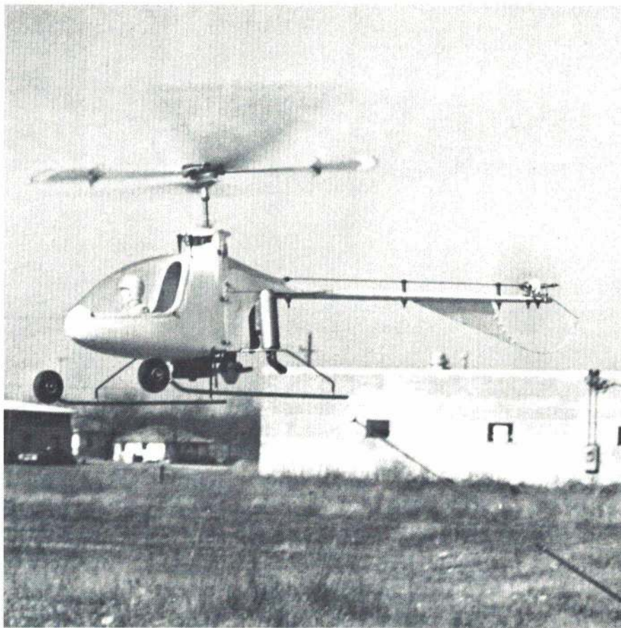
Above: The Superbird in flight with Dave Grey at the transmitter. He likes to fly so close in hovering that you can reach out and touch the helicopter. Below: Stylish body houses four-channel radio entirely inside. External fuel tank shows when to land without disaster.
