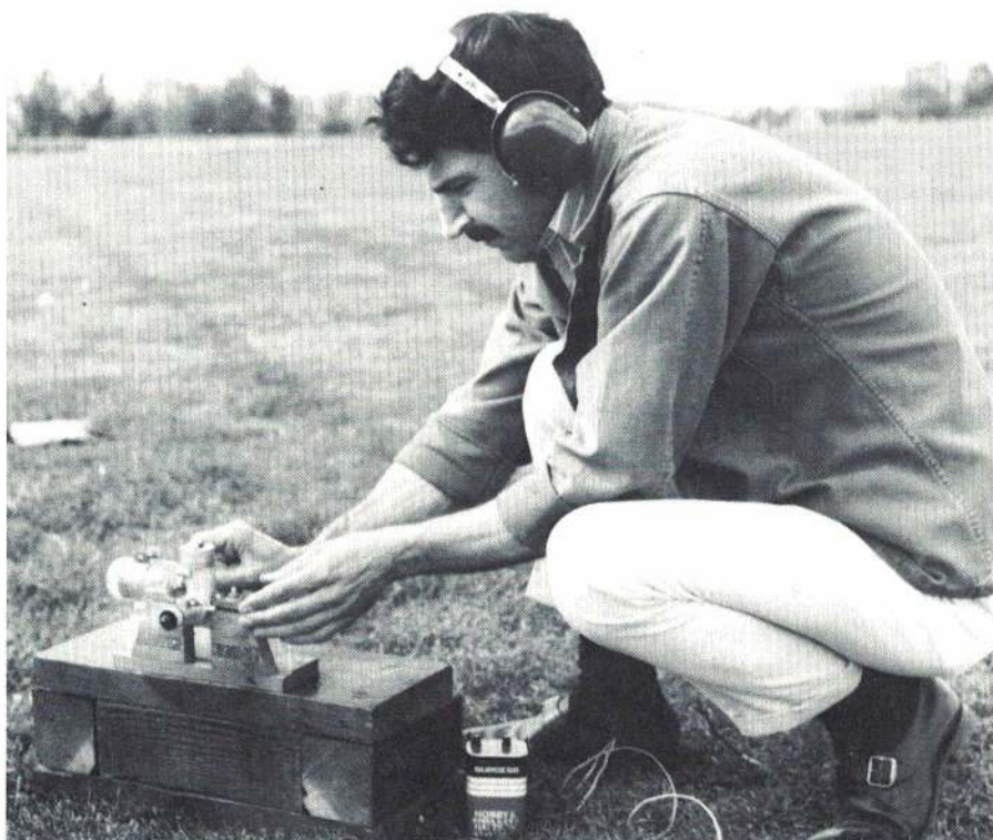
This sound level meter is used to approximate the degree of hazard to hearing from noise. Modelers should be aware of this danger and take appropriate precautions.
