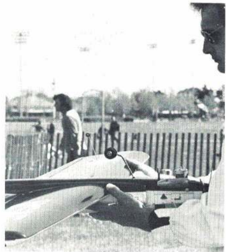
A U-2 semi-scale stunt ship by Joe Adamusko has unique landing gear system. Power is an OS 35 with Grish 10-6 three-bladed prop.
