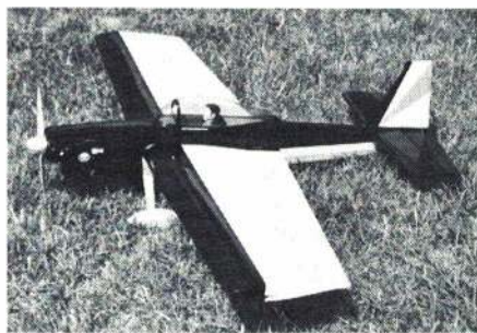
ABOVE: Tom Dixon's Stephen's Akro, 52-in. span, 53 oz. wt., OS 40. Tom is particularly proud of this Akro as it flies circles around his Phoenix. Tom plans a new Akro for next year. BELOW: Dixon's OS 35-powered Phoenix, 55-in. span, foam wing, 52 oz. wt.
