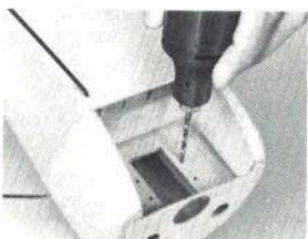
Drill engine and equipment mounting holes.
