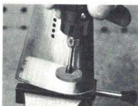
Polish intake ports. Lighten pistons and rods.
