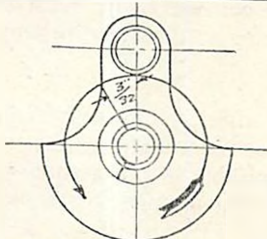
SKETCH NO. 51 SHOWING POSITION OF THE EXHAUST VALVE WITH REFERENCE TO THE CRANK PIN. VIEW LOOKING FROM FRONT SIDE TOWARD THE REAR
