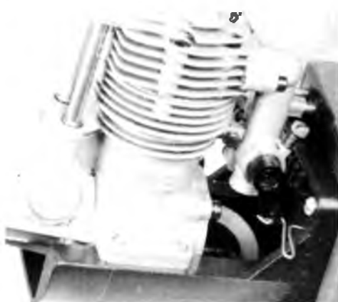
Note loop in throttle pushrod for adjustment and strain relief.
