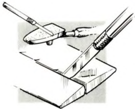
Heat knife blade on MonoKote iron, then use blade to seal down covering in awkward-to-reach places.
