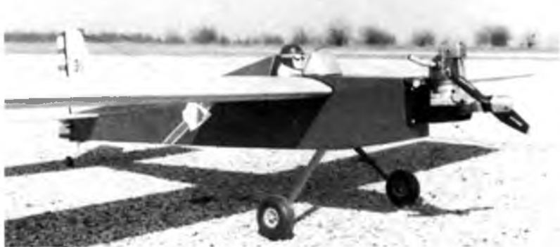
An ideal model for four-strokes, the Hawkshaw adapts readily to two-strokes as well.
