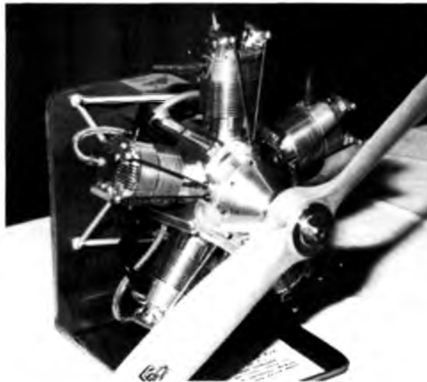
One of the most beautiful four-cycle engines available is the 5-cylinder radial from Forest Edwards. This engine has been extensively tested and flown.
