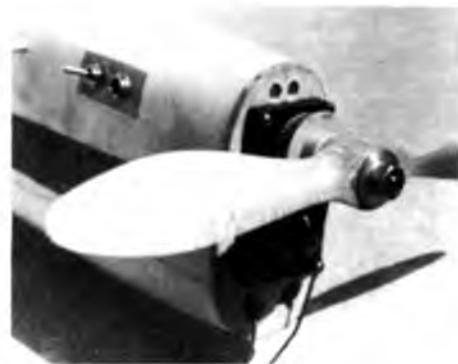
Reworked 10x8 Top Flite yields reduction in drag from hub area. Plane is King Condor conversion with Astro Flight belt drive.
