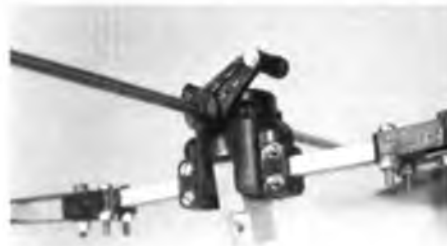
The completed mechanical assembly, far left, and close-up of main rotor head showing flybar control arm, right, show good engineering technique.
