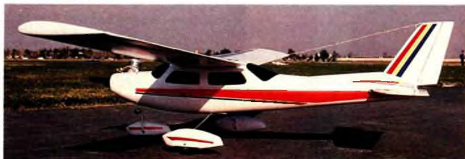
Type: Advanced trainer/scale Wingspan: 60 inches Wing Area: 520 square inches Weight: 6 pounds, 6 ounces Engine: Picco .40 Channels: 4
