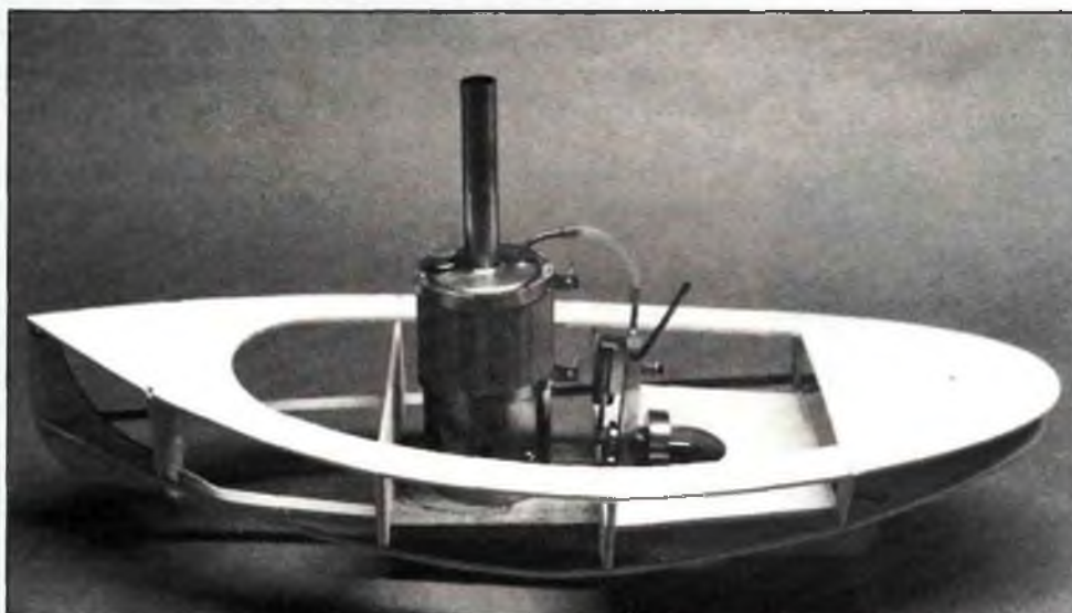
Left and above: Steam boiler is silver-soldered. A fuel used is lantern kerosene.
