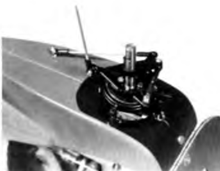
The swashplate with all linkages installed.
