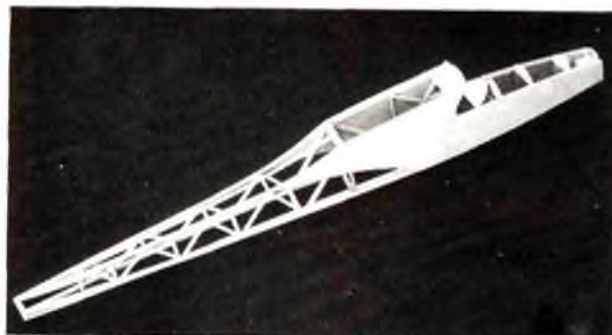
Framed fuselage is a light, strong structure.
