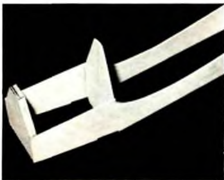
Make sure formers F1 and F2 are at right angles to fuselage sides.
