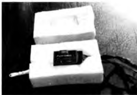
Receiver padded inside two foam blocks.
