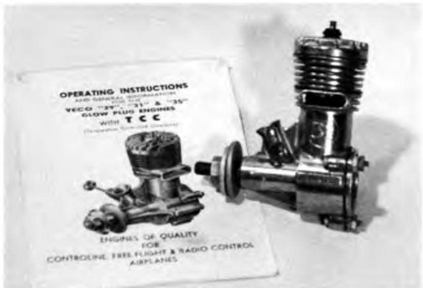
A Veco "31" circa 1953, this version made while columnist Wagner was Veco chief engineer.
