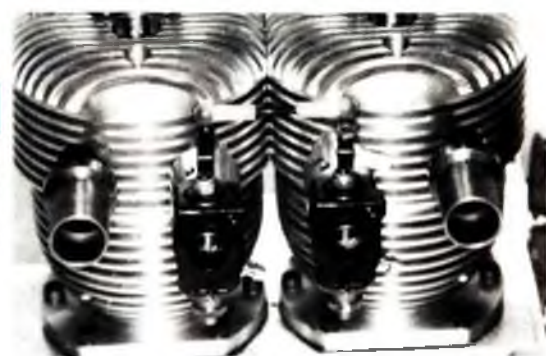
Another unique aspect of this twin is the use of dual carburetors.
