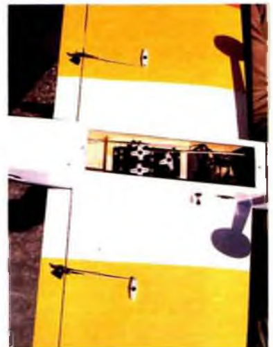
Shot of the radio installation from removable lower hatch shows use of dual aileron servos.
