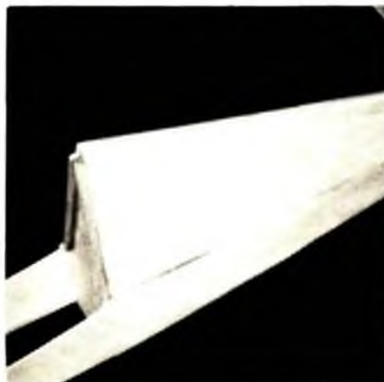
Rear fuselage sheeting in place is blended into lite-ply fuselage sides.
