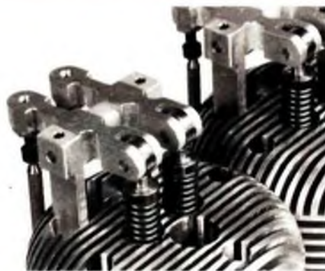
Superior workmanship and machining techniques are apparent left and above. Note man-sized rocker arms and return springs.
