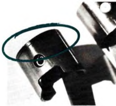
Glazed piston is a result of using improper fuel mixture.
