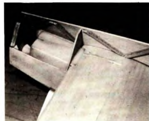
Be sure tank is installed prior to completion of top forward fuselage section.
