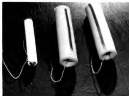
Ace battery with redundant airborne system. Note protected batteries inside sleeve.
