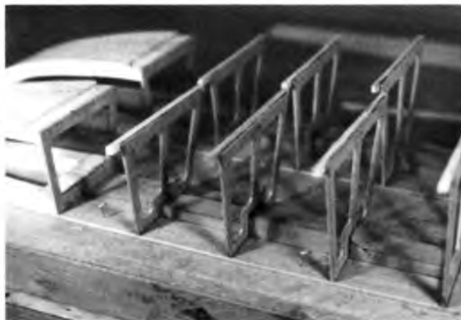
On author's current project, top deck of floats pinned down and bulkheads secured. Note hollow balsa nose.
