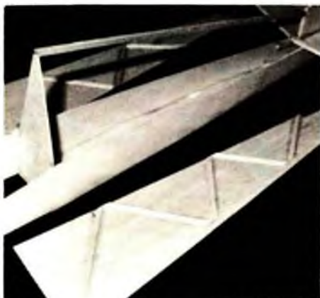
Reinforcement strips of 1/16-inch balsa save weight and add strength.
