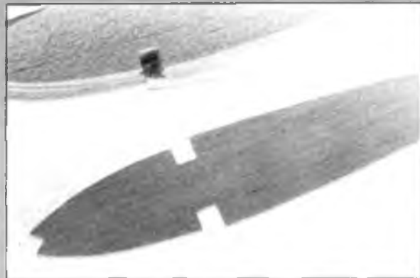
Above left: An example of bad die-cutting. Note rounded corners. Above right: A good die-cut sheet shows crisp, distinct parts. Right: An example of a machine-cut and sanded rib from a high-quality kit.
