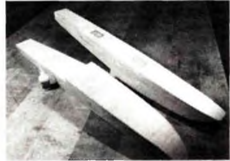
Arrow Sport's floats completed. Note plywood insert.
