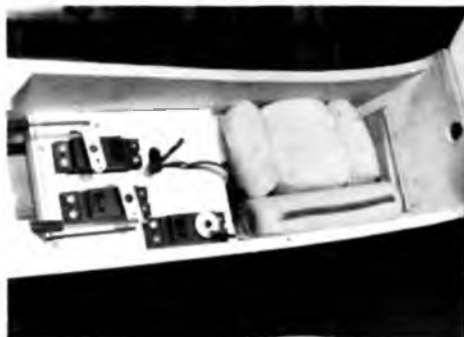
Two battery packs and Rx in place. Spaces filled with foam, no room for movement.
