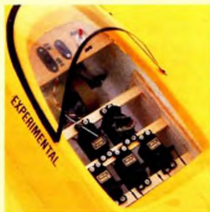
Above: Cockpit view shows servo layout. Below: The Bandit is a docile flyer.
