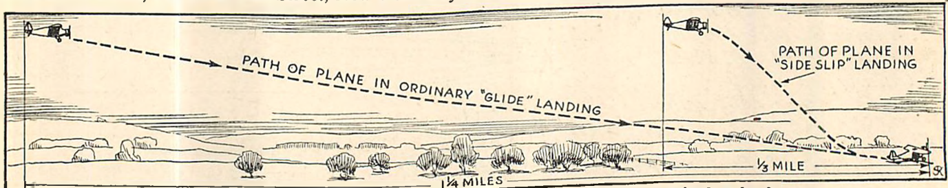
Fig. No. 2. This shows how a "side-slip" shortens the distance required to land.
