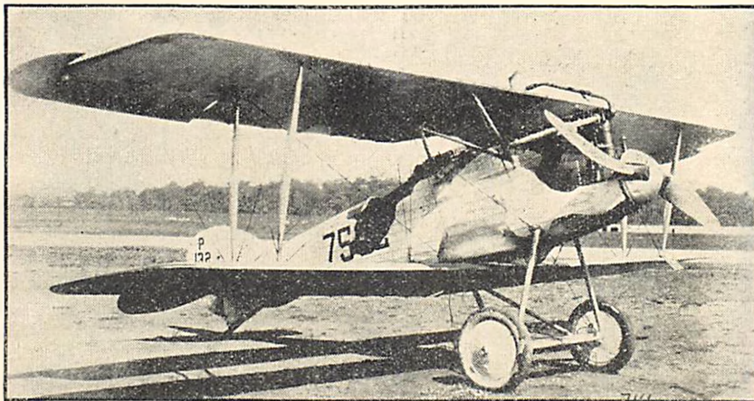
This is the German Roland D. VI, used extensively during the last year of the war. Its design is comparable with present day planes except in the type of construction used. It was powered with a 160 h.p. Mercedes six-cylinder engine. The fuselage was of the monocoque type.
