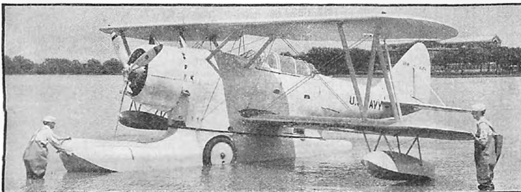
Here is the Navy's newest utility plane, the Grumman Amphibian JF-1. It is a single-bay staggered biplane of equal span. The fuselage and hull are of metal structure. The undercarriage is of the two-wheel retractable type, mechanically operated. Power is furnished by a Pratt and Whitney Twin Wasp direct drive engine, or a Wright Cyclone, under NACA cowling. The fuel tanks are carried in the hull.
