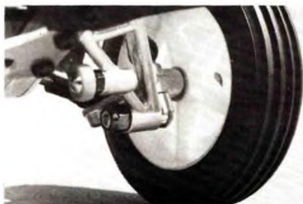
Front ribbed tire for off-road use. Good for tracks which have little mud and a fair amount of sand.
