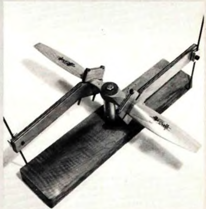
Adjusting equal pitch to both blades can be accomplished with such a jig as this. See text.
