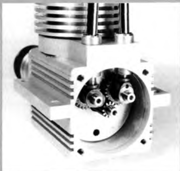
Crankcase rear end houses twin spur-gear driven camshafts. Note mushroom type cam-followers.
