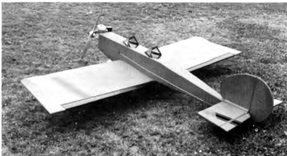
The Midwest Big Slik with Davis Diesel converted Super-Tigre 2500 proved to be an eye-opener. Read text.
