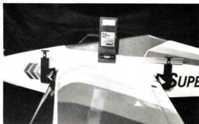
Robert Incidence Meter reading from wing tip, left, to root, above, should reveal any wing warps.
