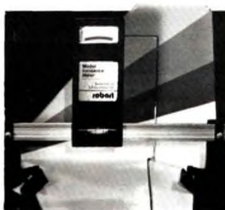
Fuselage must be level when checking engine thrust line, left, and horizontal stab, right.
