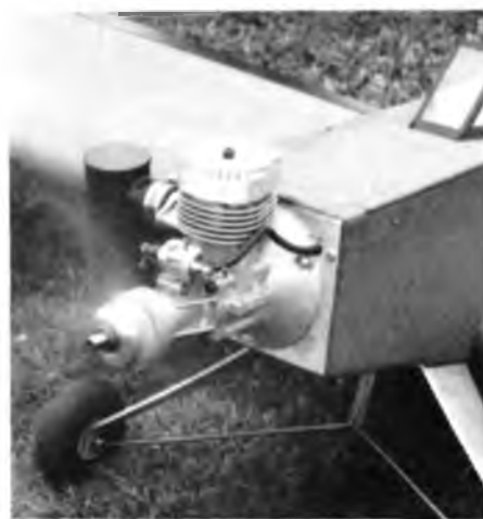
Additional power, fuel efficiency, reduced noise, and cost savings are the benefits claimed from diesel conversions.
