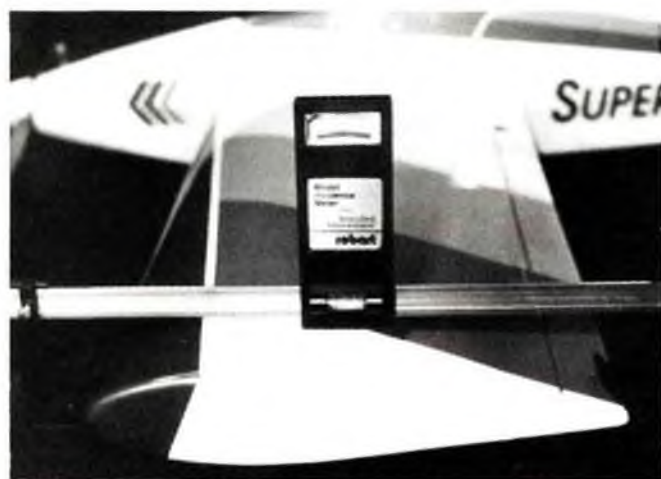
Robert Incidence Meter reading from wing tip, left, to root, above, should reveal any wing warps.
