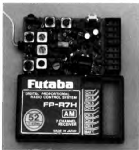
The seven-channel receiver is very compact.
