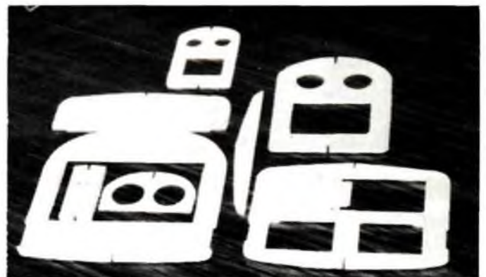
Above: Fuselage assembly begins with aft section. Right: Most fuselage bulkheads are cut from lite-ply.
