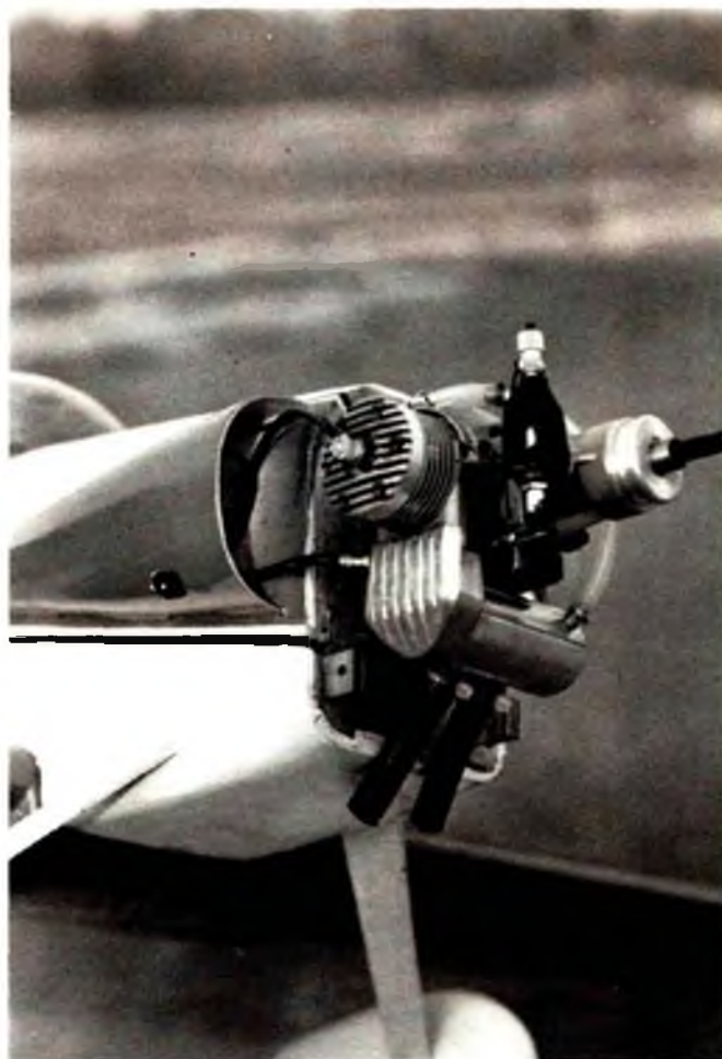
Notice at left that the firewall for four-stroke Saito .65 is recessed to achieve balance, not necessary with lighter two-stroke on right.
