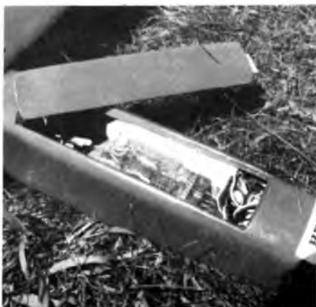
Electronics in Lelke's Heidi included electrostatic sensors.
