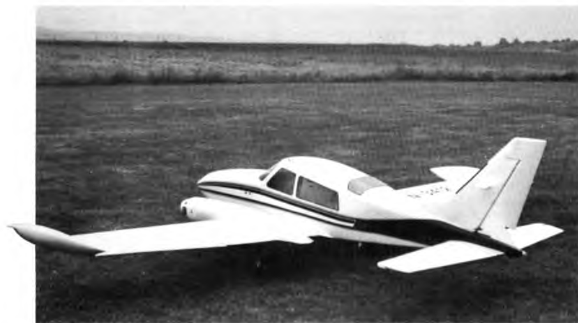
Dressendorfer's Cessna 210 is BIG! Span is over 14 feet and weight is 75 pounds. Uses two Kavan FK-50s.
