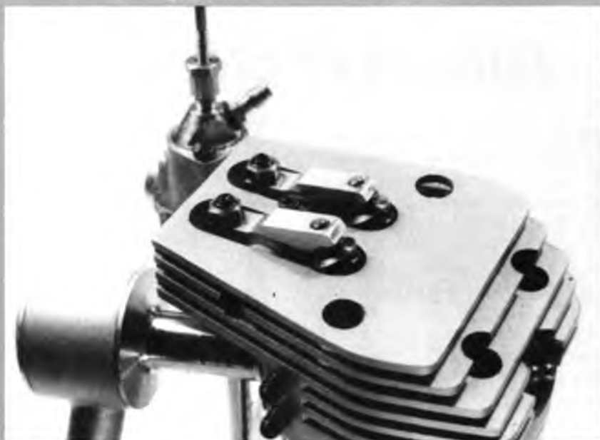
Cover removed to show rocker arms. Valves are inclined in efficient wedge head.
