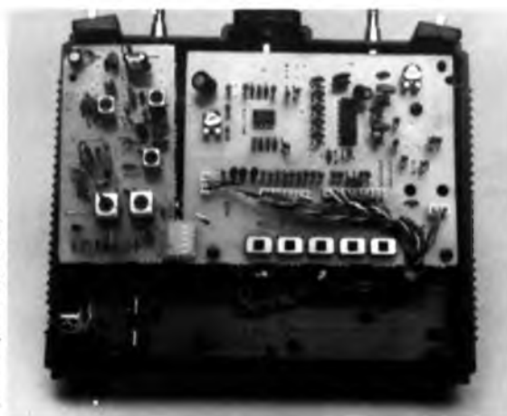
Back cover removed, RF board left, encoder right. Note 5-pin connector between boards.
