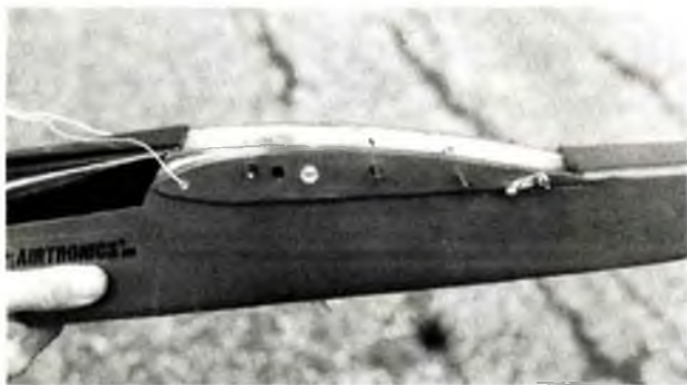
Spoiler linkages are plugged in. Actuator seen below.
