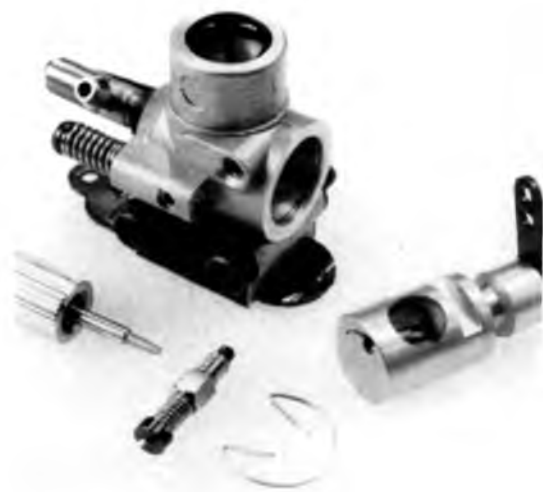
Above: Inclined valves are Saito tradition. Rocker covers removed to show neat valve gear. Right: Saito carburetor has automatic fuel metering via tapered groove in end of throttle barrel.
