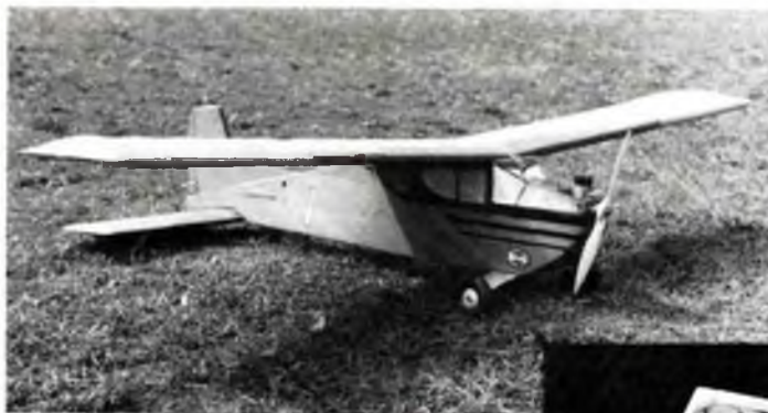
deBolt's Live Wire Senior, 1952 vintage, was a trendsetter. Box below is removable carriage that housed receiver in suspension by use of rubber bands for shock dampening.
