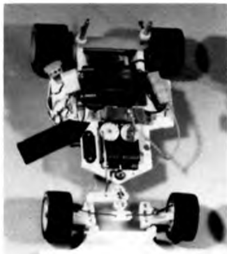
Electric road racer displays common ceramic resistor speed controller with contact wiper.
