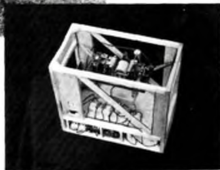
deBolt's Live Wire Senior, 1952 vintage, was a trendsetter. Box below is removable carriage that housed receiver in suspension by use of rubber bands for shock dampening.
