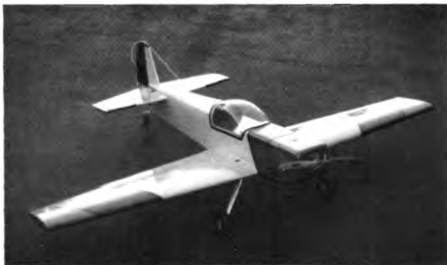
McFarlane's Model Tech CAP 21 on electric is a smooth and steady flyer. Uses a Keller 50-24 but will do equally well with an Astro 40 Cobalt.
