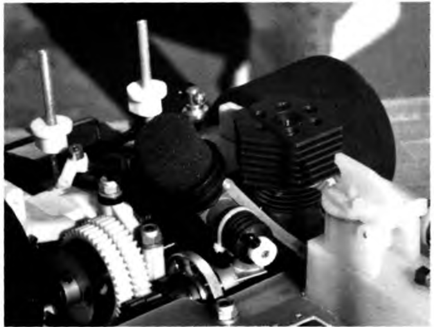
A typical gas car setup with slide carburetor. Setting a throttle response to your liking can be made easy. See text for details.
