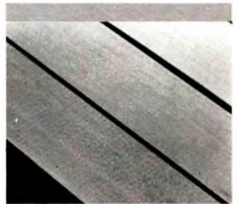
Three sheets of balsa with three different grains; left to right, C-grain, B-grain, and A-grain.
