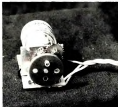
The Multi-Servo replaced the escapement and two-cent rubber band for single-channel control.
