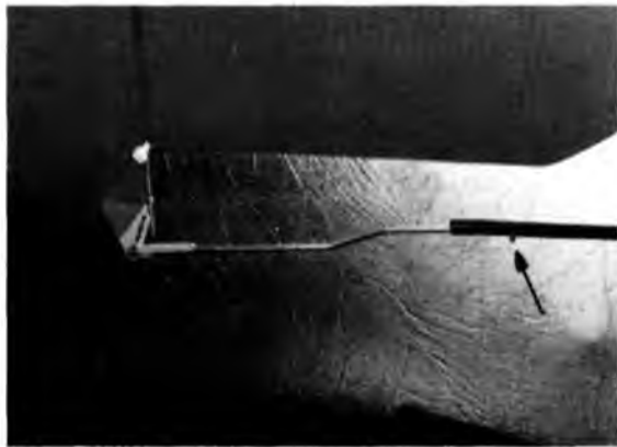
Arrow points to end of wire connector trapped by hole in arrow shaft.
