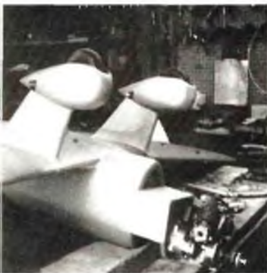
Fiberglass parts for the STA can either be formed as described in text or obtained from Fiberglass Master.
