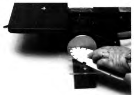
Calico Miniatures Sanding Table is used here with Dremel sanding disc adaptor.
