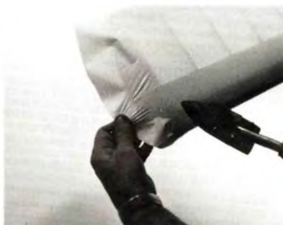
Grasp material and stretch while heating with iron.
