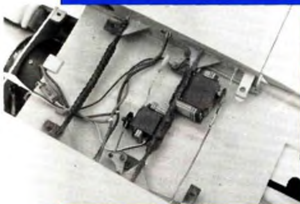
Left, servo arrangement for wing. Right, another hatch reveals nose gear setup.
