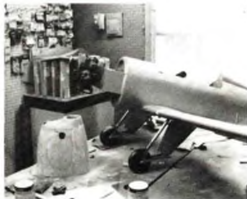
Fiberglass parts for the STA can either be formed as described in text or obtained from Fiberglass Master.
