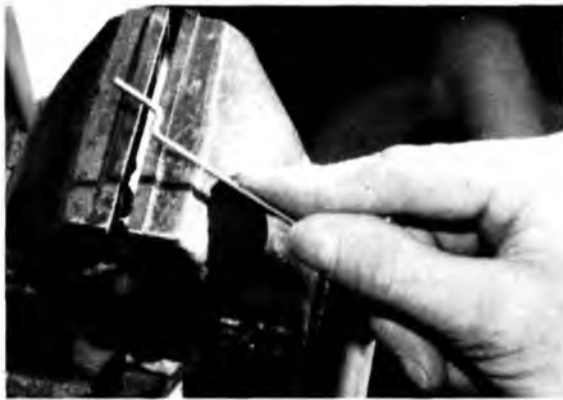
Finished Z-bend is hard to do correctly with a pair of pliers.
