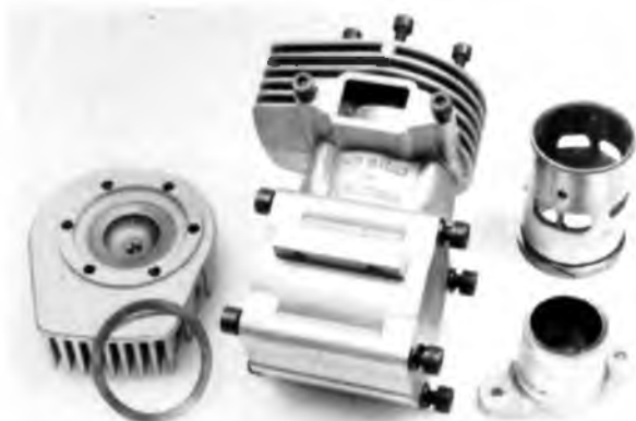
Fin area on cylinder head is biased toward hottest part of engine to even out heat dissipation.
