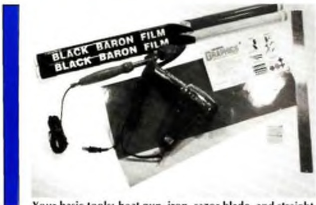
Your basic tools: heat gun, iron, razor blade, and straight-edge.
