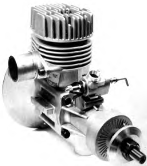
S.2000/25 here equipped with firewall mount. Note sensible size of prop driver.
