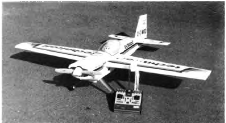
Hobby Shack's 1/4-scale Diablo (described in text) is a fully capable aerobatic design with a four-stroke engine.
