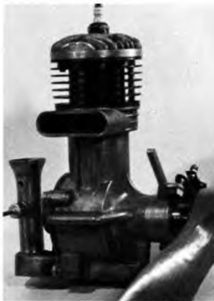
The 1946 Atwood Super Champion .60 with both rear rotary disc and crankshaft intake ports.
