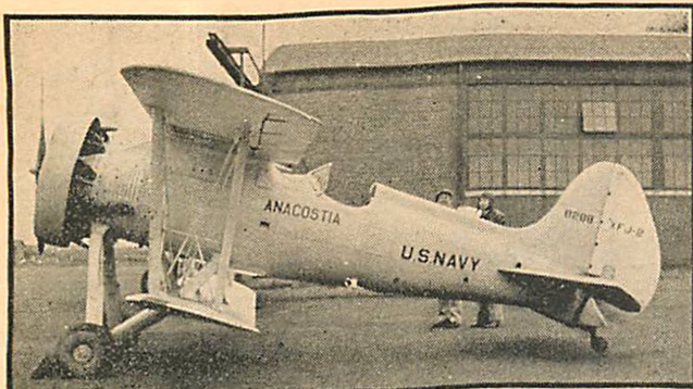
A B/J XFS-2 Navy Fighter P&W Wasp engine of 450 h.p. Speed 193 m.p.h.
