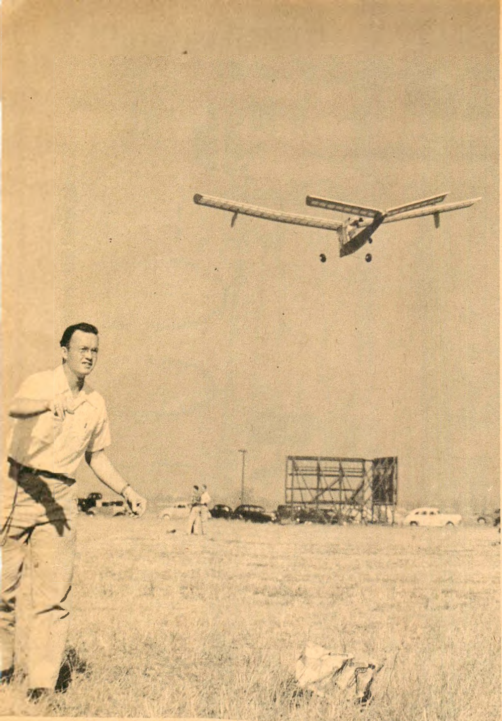
Tail first. A Spitfire-powered canard is test glided by Eugene Smith, who has developed a whole series of successful canards. Though a tail-first job, this canard is not a pusher. Note engine.
