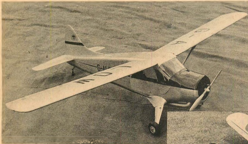
DH Beaver, by Polish builder T. S. Nachtman, Elfin 1.8 Diesel, gorgeous flier. Doors, cockpit details, adjustable pitch propeller. Has 54 inch span, won one of biggest British meets.
