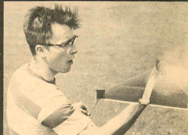
Delta 50. Part of longitudinal stability obtained by sanding the trailing edge on bottom only for a reflex section. Increased deflection is warped in during tests. The author waits tensely to launch the Delta 100 job. Note the control vane (effective under power) similar to that of the V-2 rocket.
