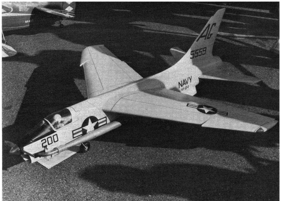
Sven Wiesendanger's Navy Crusader with piped engine driving a propeller. Ducted-fan technology now allows greater realism when modeling jet aircraft.
