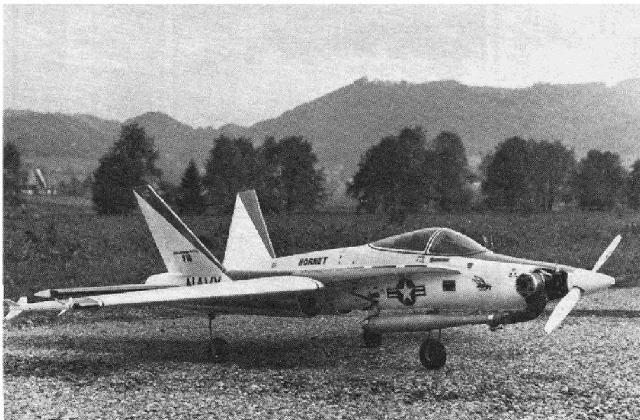
Mean-looking McDonnell-Douglas F-18 by Fred Meier is powered by a piped OS 60 pumper and uses Swiss-made Colibri retractable landing gear.
