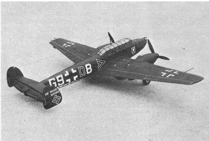
Large clear canopy requires some cockpit detailing; see plans, and cockpit photos on this page. Canopy is one piece of plastic.
