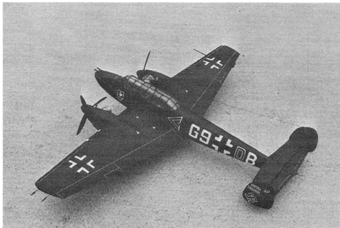
Small tabs on wing trailing edge should be bent so that outboard one is up, inboard is down. All trim is from tape and decal sheet.
