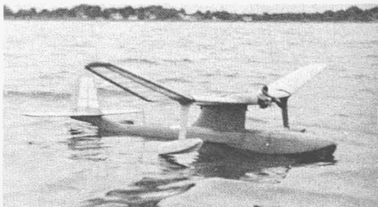
Years of research and development went into development of a design with excellent ROW characteristics. Model weighs 64 oz., gets off in 50 ft.
