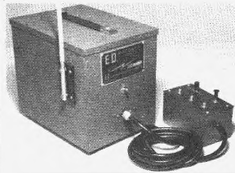
E.D. 3-channel tone equipment, to be augmented by new 6-channel, similar design. Top, right, inside control box; bottom, top, underside of receiver. Has two lever sticks and two push buttons.
