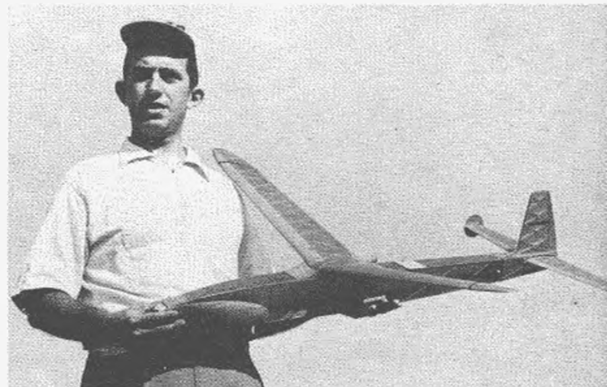
Very successful Wakefield by Carl Hermes, Arlington, Texas, under both old, new rules, Swedish Isaacson .06 airfoil and geodetic construction.
