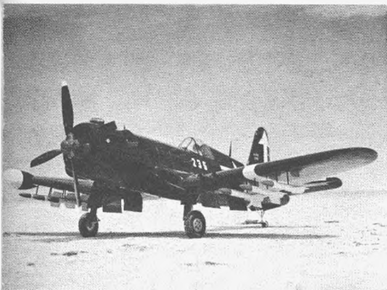
Truly incredible job done by Hess is indicated by such details as fully retractable gear powered by HO gauge locomotor. They rotate 1/4 turn.
