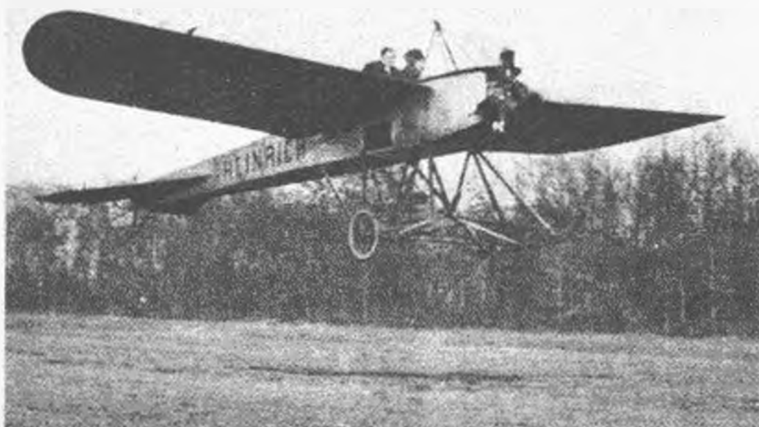
PASSENGER ON 35 HP HEINRICH MONOPLANE After 1910 plane flew, the Heinrich's built this 28-30 hp 1911 ship. Its big achievement was ability to carry a passenger. Carved own props.
