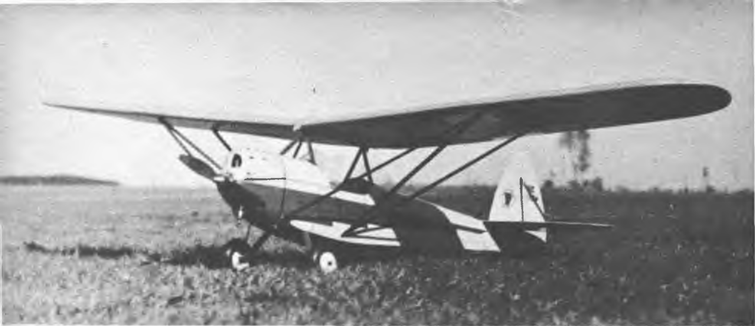
Real plane or model? Can't tell, eh? Only the cylinder head of the inverted engine is the tip-off. Wings and struts detach; are fly-off.
