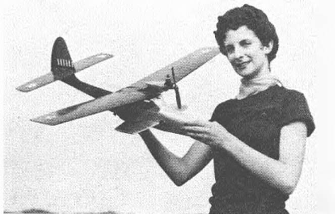
Typical Half-A powered flying boat. Author favors tip floats, rather than the more frequently seen sponsons. His three-view, herewith, is tops.
