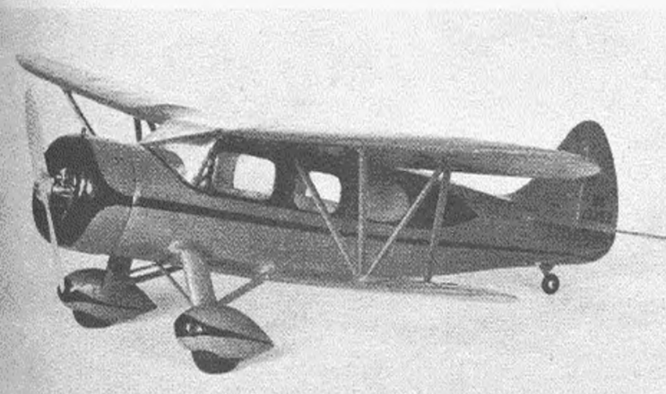
Unusual feature of Waco Cabin was the interplane strut system which, on model, adds crack-up resistant rigidity. Glow plug juts through cowl.
