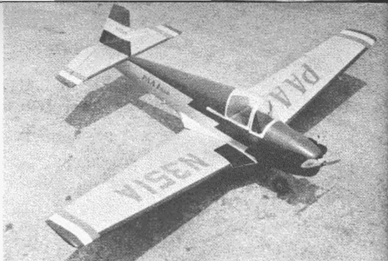
Spectacular paint scheme tops off exciting model. Canopy works. Wood is substituted for all metal surfaces and silk for fabric ones.
