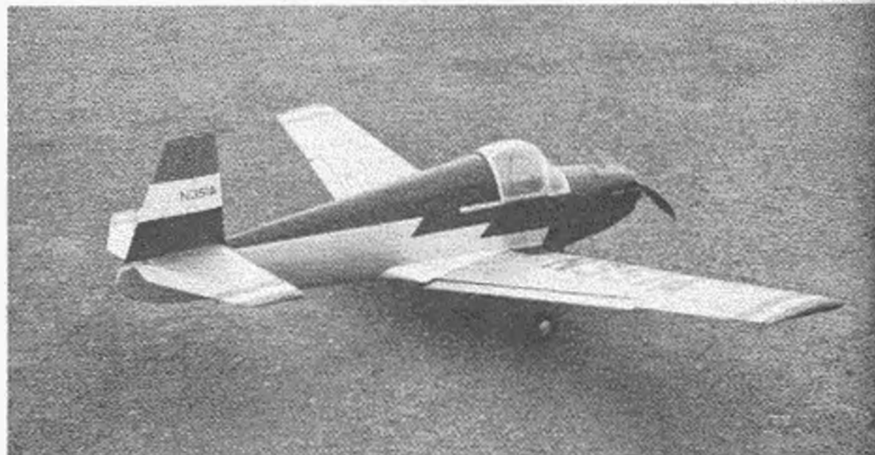
Only the usual increase in dihedral and stabilizer area departs from true scale. Tricycle gear makes take-offs thrill to watch. A prop saver.
