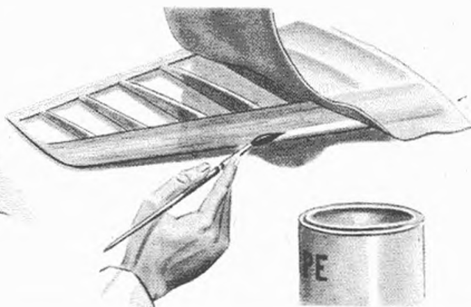
Wing sections in one piece, grain spanwise. If dihedral, use piece each panel. Dope edges, pull out to eliminate wrinkles.
