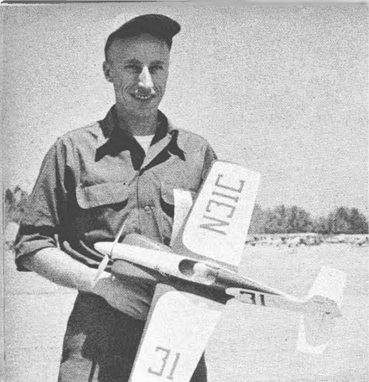
Sheet-metal team racer here displayed by author is his K & B Allyn .23-powered Skeeter, a faithful copy of the prototype. A Goodyear racer.
