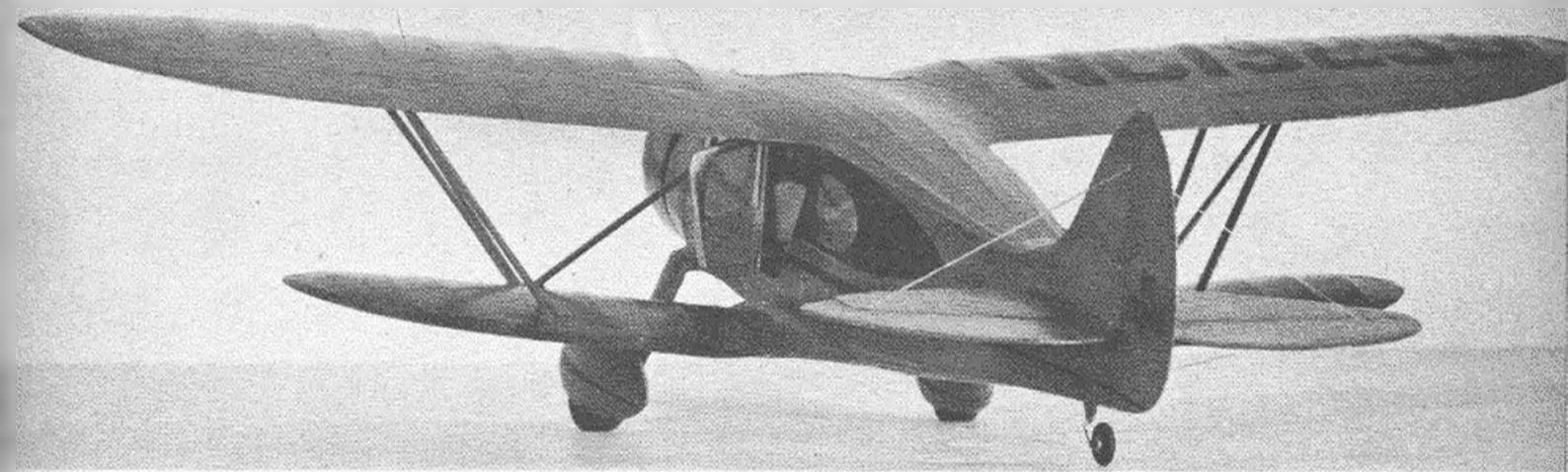
An almost indiscernible increase in dihedral and a slight addition to the stabilizer area are the only departures from scale. Note open cabin door.
