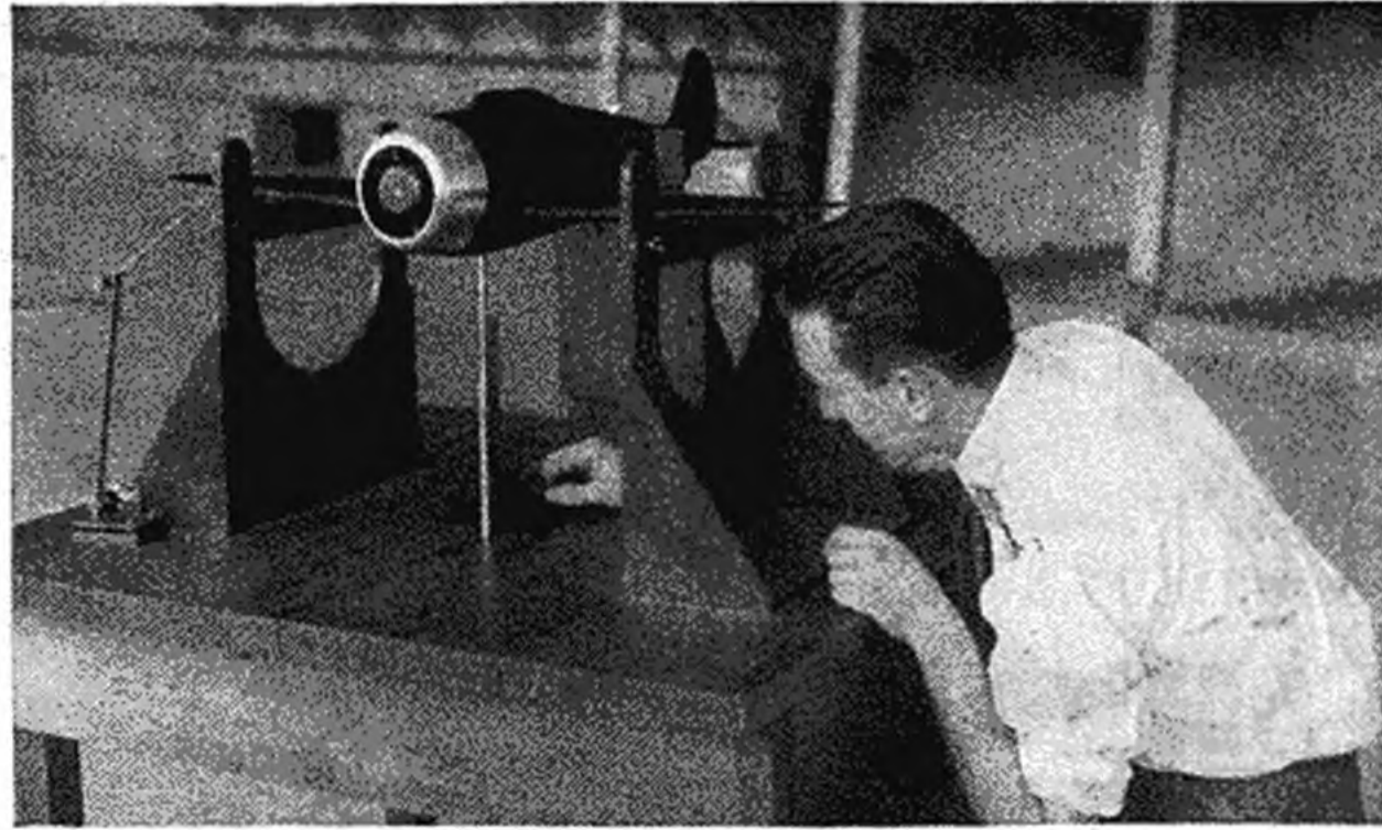
Checking the accuracy of a tunnel model with precision instruments
