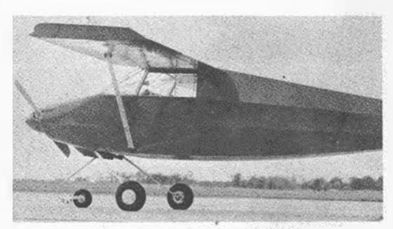
Unique trike gear an Wittman W-9L. Tailwind, handles beautifully, minimizes bad landing shocks, virtually eliminates fuse damage.
