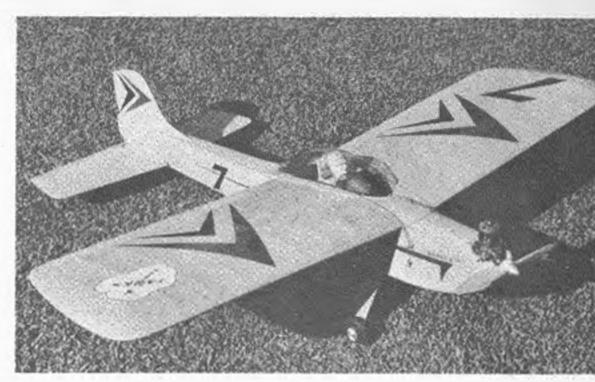
Detailed cockpit and dummy pilot Shearer's model suggests racer. To hold down nose at high speeds, use 5-8 degrees down thrust.
