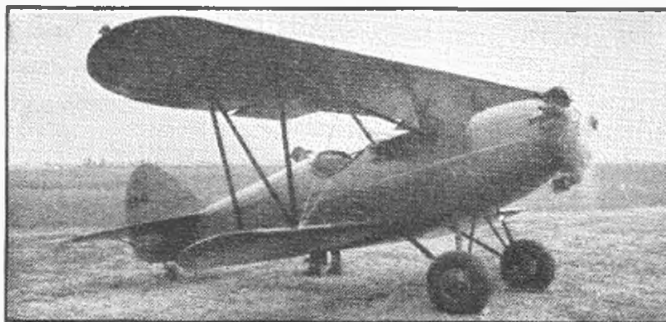
Here is the new Bird "Speed" powered with a LeBlond 90hp. engine
