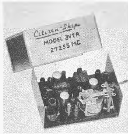
Relay, Citizen-ship 3VTR, can be removed, if so desired because of high current change possible.
