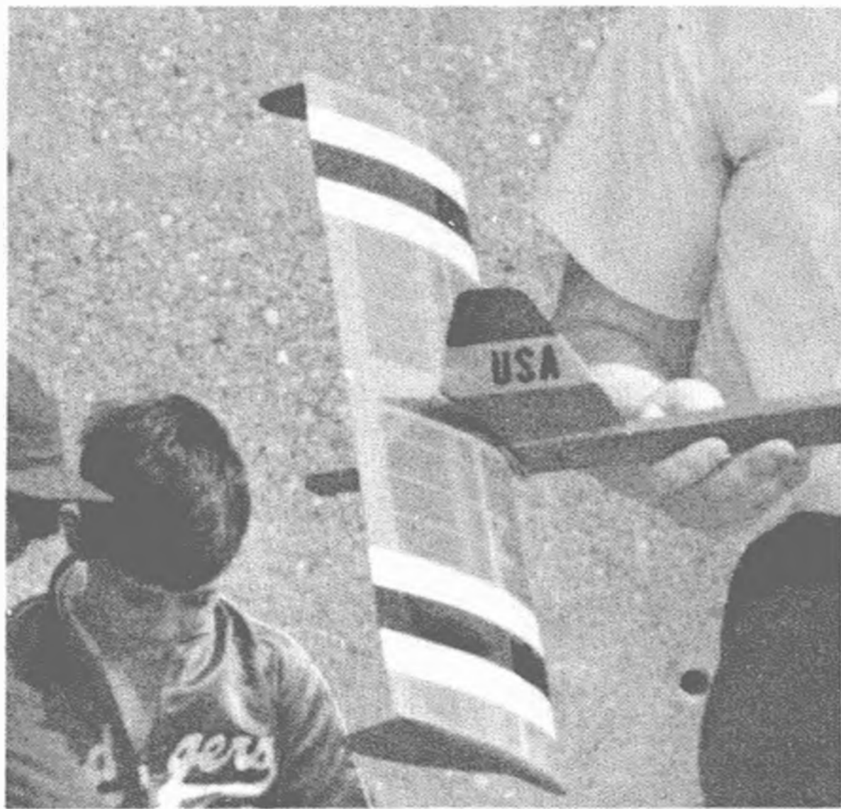
Typical "pop up" tail, this case a stabilizer, with fixed rudder. Proper action brings ship down steeply but with nose up, steady. No turns.
