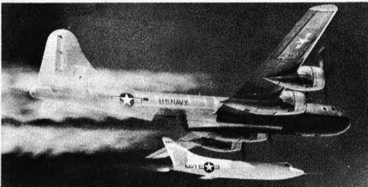
Shortly after this launching shot of the Douglas Skyrocket dropping from its mother ship was taken, the needle-nosed rocket job-jet was removed—set speed and altitude records estimated as high as 1,324 mph at 72,000 feet. Below—Take-off on the desert for an earlier speed run.
