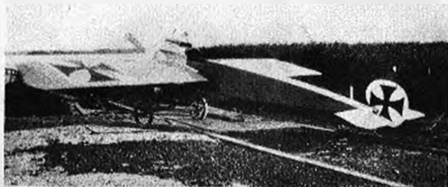
Powered by an 80 hp Oberursel, E-1 had wing warping lateral control.
