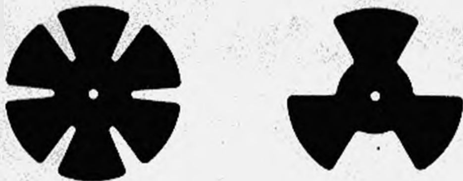
Half-size patterns of two successful fans used by author. Specifications must be carefully followed for successful flying of jet planes.
