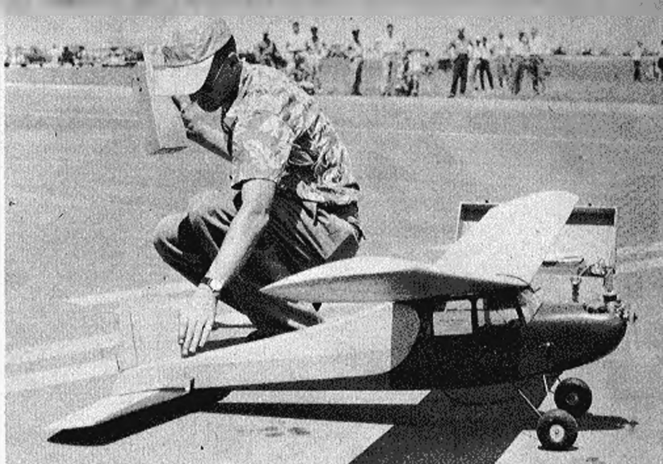
Howard Bonner about to release MacNabb equipped rc job. Two-speed K & B glow .19 really howls.
