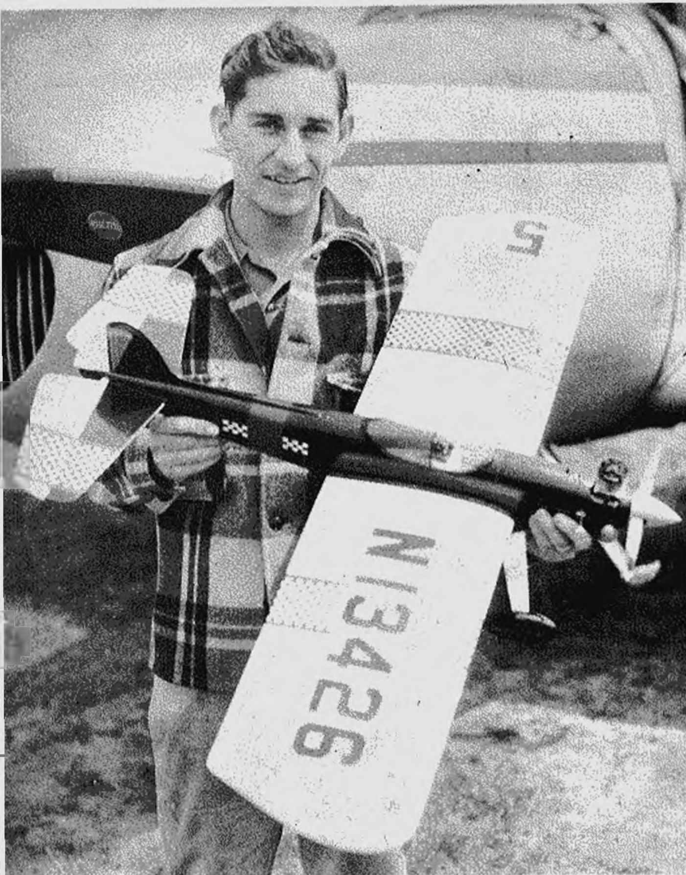
Built in all sizes from AA jobs to big "60's," the Ringmaster has proved its ability. Wing construction features an I-beam, sheeted edges; fuselage has sheet sides, extra long motor mounts.
