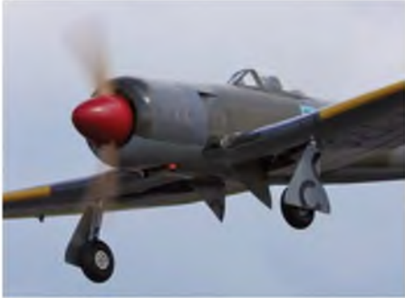
Brian Rawcliffe's superb MK II Hawker Tempest. It spans 97" and weighs 41 lbs. Moki five-cylinder radial.
