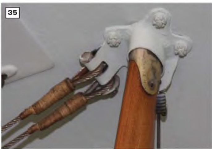
29: The complete tailcone. Note the space between the fin and tailplane. 30: Bracing wire anchor point on the tailplane upper surface. 31: Rudder, showing the bracing wire from the control horn to the rudder trailing edge. 32: Rudder control horn close-up. 33: Tailplane underside bracing strut. 34: Tailplane underside bracing wire. 35: Detail of one of the interplane strut locating 'shoes'. 36: Same view, showing the access panel in the upper wing lower surface. 37: Detail of the instrument venturi (upper left outer wing) close to the leading edge. 38: Another view of the instrument venturi run to the upper wing aileron. 39: Lower wing/ fuselage. 40: Another view showing the centre-line cap between the upper wing panels
