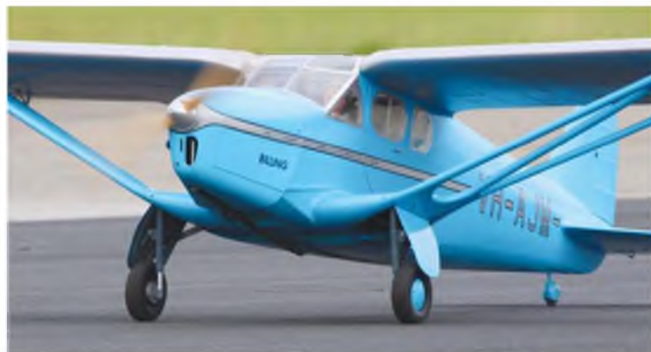
Derek Martin's exquisite 1/4 scale Heston Phoenix. Wing Span: 10 foot 1 inch; weighs: 39lbs. Engine is a 3W 70i driving a 24x10 prop.
