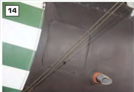
13: General view of the forward fuselage. 14: Fuselage access panel, just behind the engine cowl. 15: Wing root detail, showing the anchor point for bracing wires that run from the top outer wing strut. 16: Rear fuselage lifting handle, positioned forward of the tailplane. 17 & 18: Two views of the cabane assembly, viewed from front three-quarter. 19: Cabane again, viewed from rear. 20: Cabane assembly, also revealing the 'lip' on the cowl rear edge and the narrow space between the wing halves on the centre-line.
