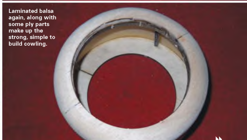
Laminated balsa parts provide the nose shape and the motor mount parts set the thrust lines.
