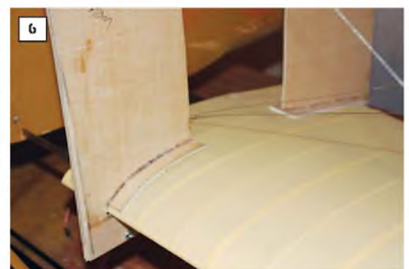
1: The components of the ply support jigs band-sawn to shape and with the strip wood fore & aft joiners glued on. 2: One of the support jigs, now with the support shoes in place. Note the foam cushions. 3 & 4: Close-ups of the support shoes showing the foam inserts that protect the fabric covering when slotted over the wing leading and trailing edges. 5: Here the left hand wing sub-assembly is being slid off the Graupner wing joiner 'blades'. 6: Detail of the support jibs, slotted over the wing panel leading and trailing edges. 7: One complete wing 'half' supported by the jig and the interplane struts. All the wire rigging remains in place.
