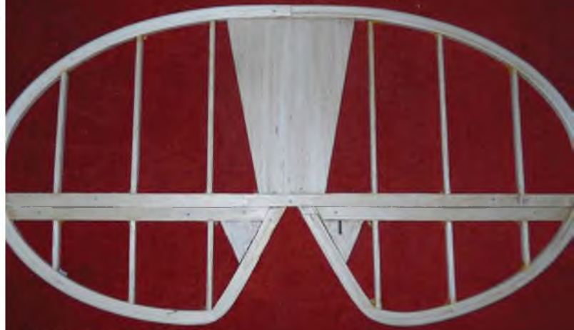
The only difficult part of the tail surfaces is laminating the outlines.
