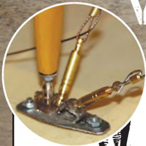
LEFT: This is as close as I could get, with just hand tools, to the interplane strut anchor-point brackets that were a feature of the full size Albatross D.II., made from sheets metal and brass picture hooks.
