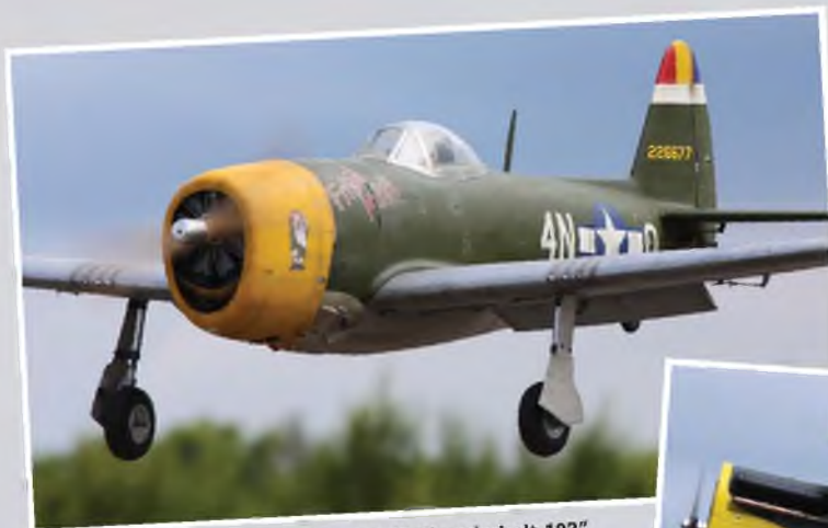
Ray 'Ozyray' Peters Frigid Midget P-47 Thunderbolt 102" span from the Martyn Serginson plan pack. ZDZ 80cc power / Menz 26x8* prop. Ray Slack retracts.
