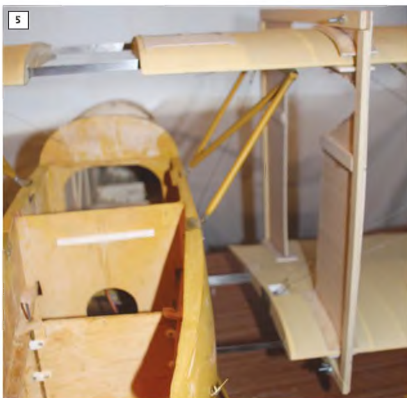
1: The components of the ply support jigs band-sawn to shape and with the strip wood fore & aft joiners glued on. 2: One of the support jigs, now with the support shoes in place. Note the foam cushions. 3 & 4: Close-ups of the support shoes showing the foam inserts that protect the fabric covering when slotted over the wing leading and trailing edges. 5: Here the left hand wing sub-assembly is being slid off the Graupner wing joiner 'blades'. 6: Detail of the support jibs, slotted over the wing panel leading and trailing edges. 7: One complete wing 'half' supported by the jig and the interplane struts. All the wire rigging remains in place.
