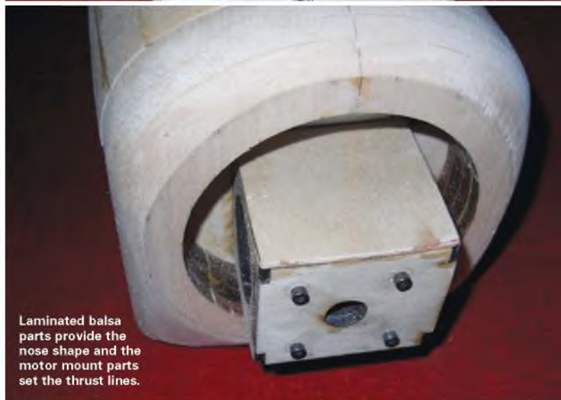
Laminated balsa again, along with some ply parts make up the strong, simple to build cowling.
