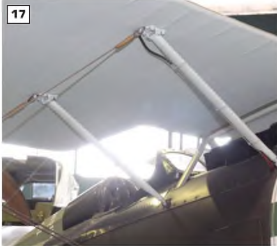
13: General view of the forward fuselage. 14: Fuselage access panel, just behind the engine cowl. 15: Wing root detail, showing the anchor point for bracing wires that run from the top outer wing strut. 16: Rear fuselage lifting handle, positioned forward of the tailplane. 17 & 18: Two views of the cabane assembly, viewed from front three-quarter. 19: Cabane again, viewed from rear. 20: Cabane assembly, also revealing the 'lip' on the cowl rear edge and the narrow space between the wing halves on the centre-line.
