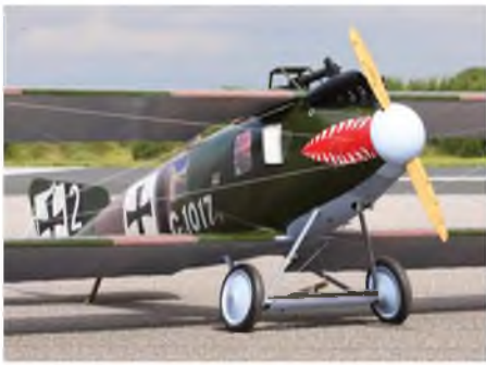
Superb LFG Roland CII 'Walfisch', built by Barry Banks, to 1/3rd scale. Spans 135" and weighs 42 lbs, with Moki .75 power.
