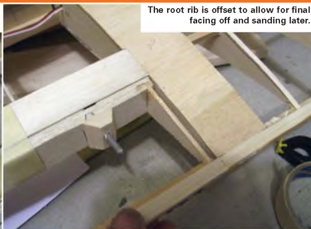
The Robert hinges supported in 9mm dowel.
