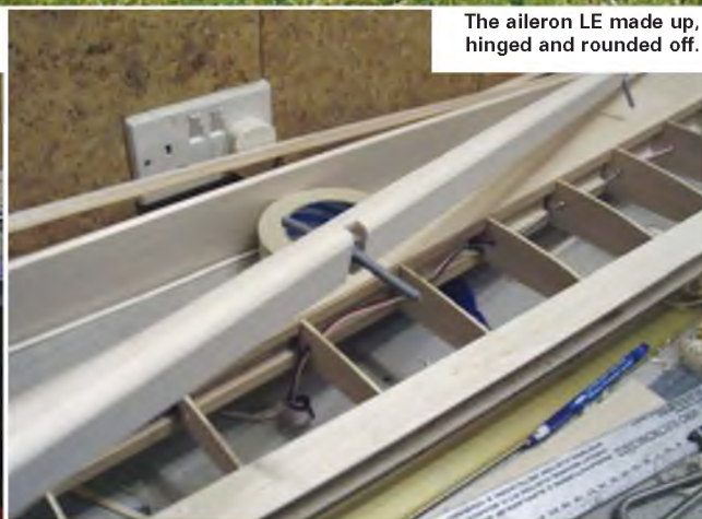
The aileron trailing edges made up from a lamination of balsa & spruce.
