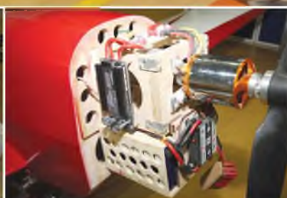
Andy Boylett's half-scale / 14 foot span Spacewalker 2 from the factory drawings. Fitted with twin/tandem Turnigy 15 Kilowatt-rated motors (20 Kilowatts peak).
