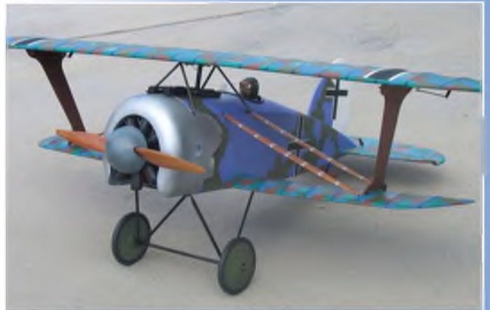
For a 'quick and dirty' build Pat Lynch's DXI looks pretty good to me. This time the lozenge is painted onto film covering.
