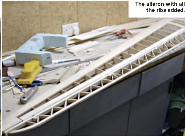
As the initial ribs are added, the TE must be checked for straightness.
