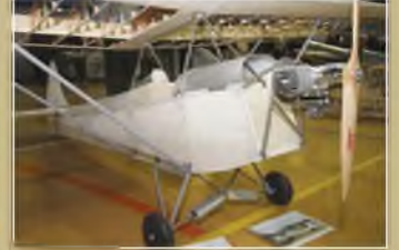
Tony Hill's Luton Minor spans 12 feet six, weighs approximately 50 lbs. DLA 112 petrol engine.
