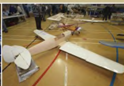
The "Nearly Done Aircraft Company Inc's" DH 94 Moth Minor. 146" span, weighs 22 kgs, and powered by a Revolution 50 electric motor.
