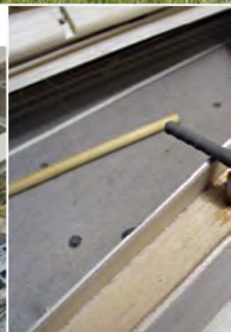
The aileron LE made up, hinged and rounded off.
