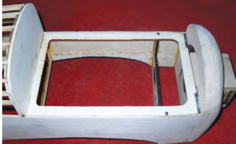
The liteply plate around the avionics bay adds rigidity and provides a good base for the hatch to sit on.
