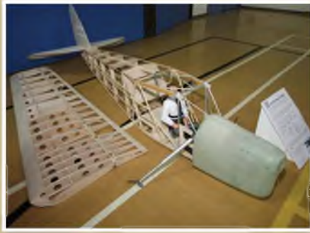
John Rickett's 1/3rd scale DH 85 nearing completion. Model spans 12' 6", and weighs 35 lbs.
