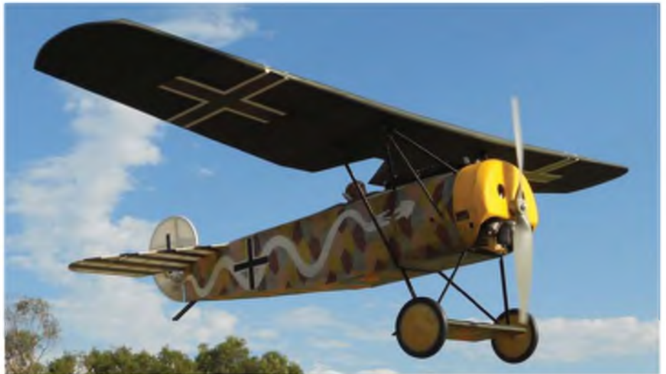
Another one there wasn't room for is the Fokker DVIII by Simon Uglow. The lozenge uses an interesting cut tissue over Litespan technique.
