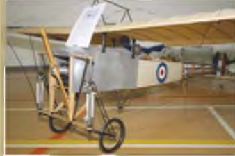
Dave Bailey's Bleriot Parosol 1914 is 1/3rd scale, and weighs 42 lbs. Wingspan 13 feet, powered by a 70cc two-stroke twin.
