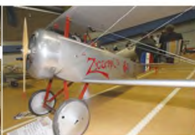
Tony Slater's Zigomar 5 Nieuport 24. 1/3rd scale, spans 108", and weighs 26 lbs. RCG 62cc direct drive petrol engine.
