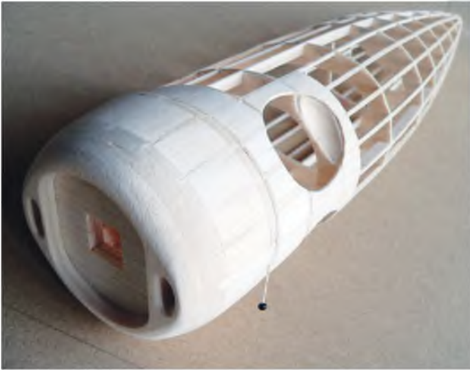
My model was to be a competition scale job, so features realistic cut outs for the landing gear. It's a real fiddle, so if your model is for general flying just paint a black circle here. If you are flying outdoors just leave the gear off and make dummy half-wheels.
