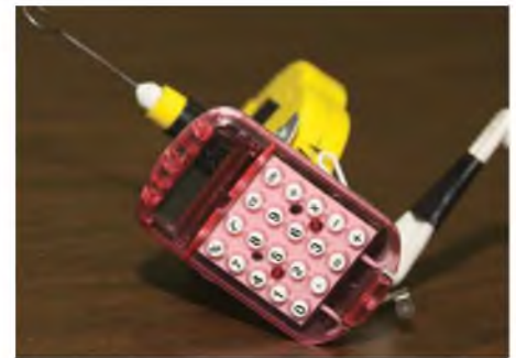
Tim Milner's clever (Electronic Calculator) Digital Turns Counter grafted onto a geared winder.
