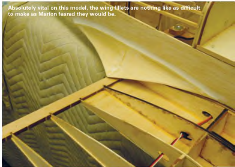
A ply rib, cut to accept the main u/c wire, with a ply doubler each side, makes for a very sturdy u/c mounting in the wing.
