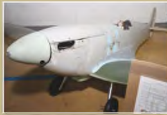
Rob Buckley's Spitfire Mk IIa built to 1:5 scale, weighs 25 lbs, and a wingspan of 89 inches. Powered by a 3W 40cc petrol engine.
