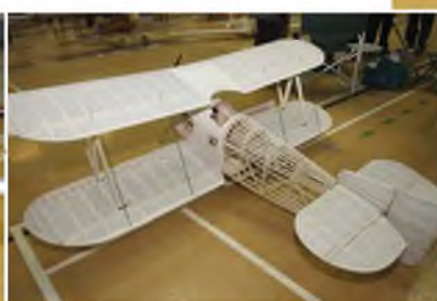
Ken Dallow's Flycatcher built to 1/4 scale to Ken's own plan, weighs 22 lbs, and spans 87 inches. Saito 36cc power.
