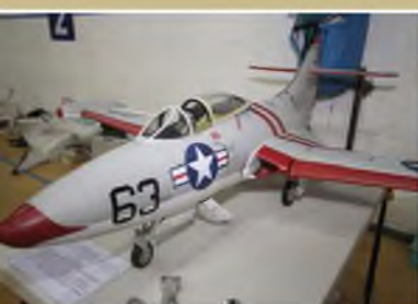
Grumman Panther, the F9F-2P version, to 1:63 scale and weighing 9 kgs without fuel. Built by George Firth from fibreglass components made by Jim Ashcroft. Powered by a Wren 70 gas turbine.
