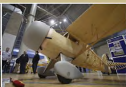
Mr Mulligan is built to 45% scale, and spans 171 inches. 342cc boxer twin.
