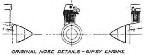
ORIGINAL NOSE DETAILS - GIPSY ENGINE
