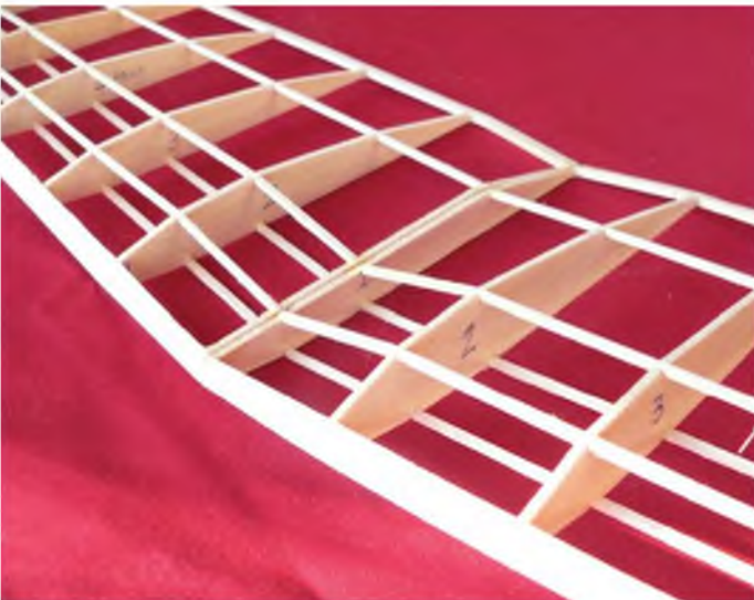
Note how the centre rib is a strange shape to allow the rubber motor to pass over the top. This straight-through wing design is very strong. You may also notice that I have 'faceted' the wing ribs between the spars. This makes for a smoother looking wing as the bumps caused by the ribs don't show through the tissue covering.
