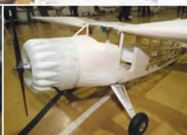
Dave Houghton's Stinson Reliant spans 100" and weighs 27 lbs. Powered by a Saito 182 Four-stroke twin engine.
