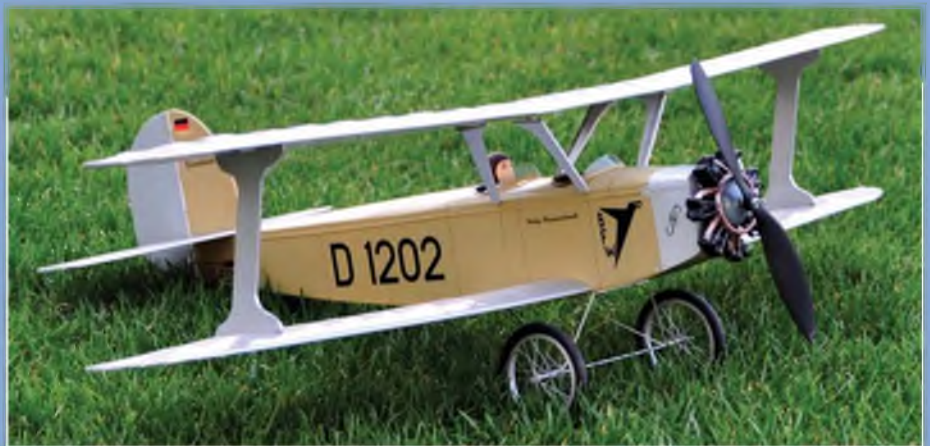
Painted laminating film and Solarfilm combine to result in a rather nice looking little Udet Flamingo.
