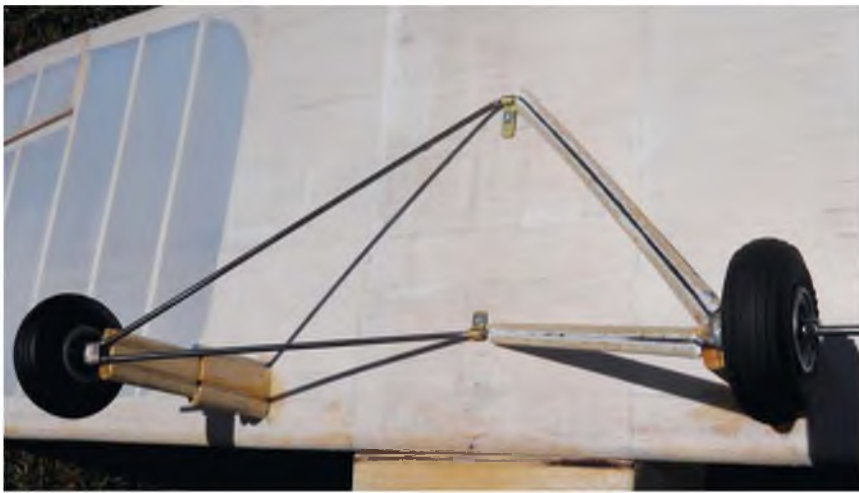
As the scrap balsa fairings start to go on the u/c, you can see clearly how the front and rear legs are retained.
