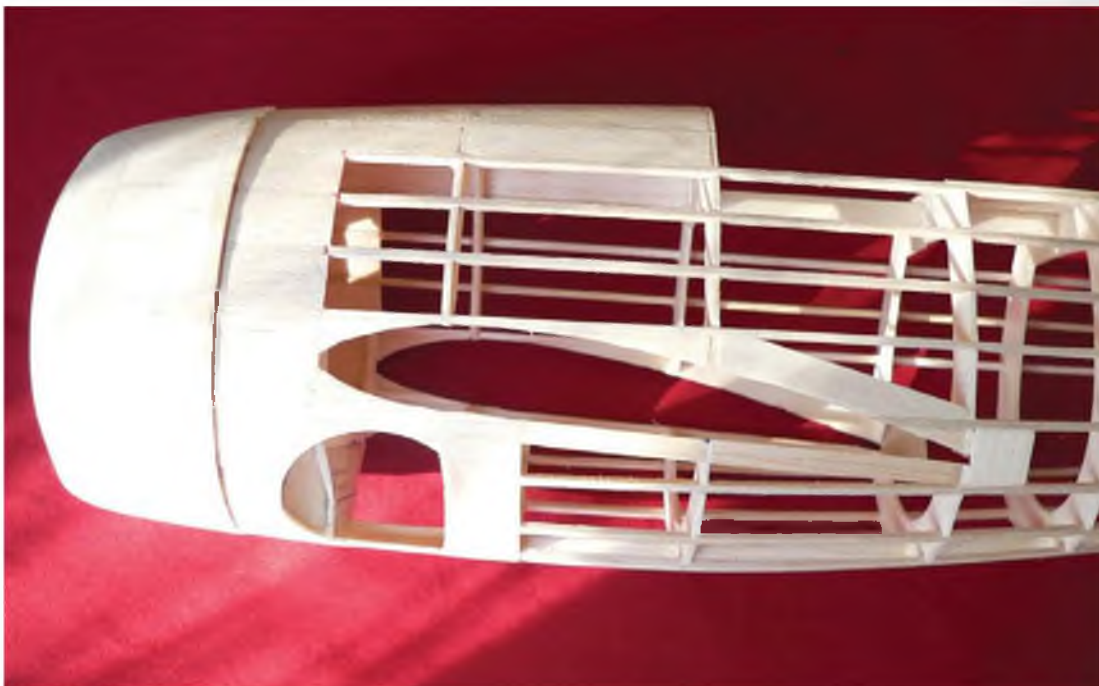
Note how the shape of the wing aperture is cut out of 1/16" sheet balsa in-fill. Note also the fill-in 1/16" soft balsa sheet around the nose. You can afford a little weight at the front end like this, but keep the rear of the model as light as you can at all costs!
