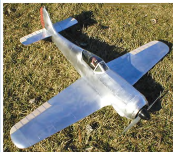
It takes a lot of surface preparation and careful application to get the aluminium tape to go onto the model as well as this.
