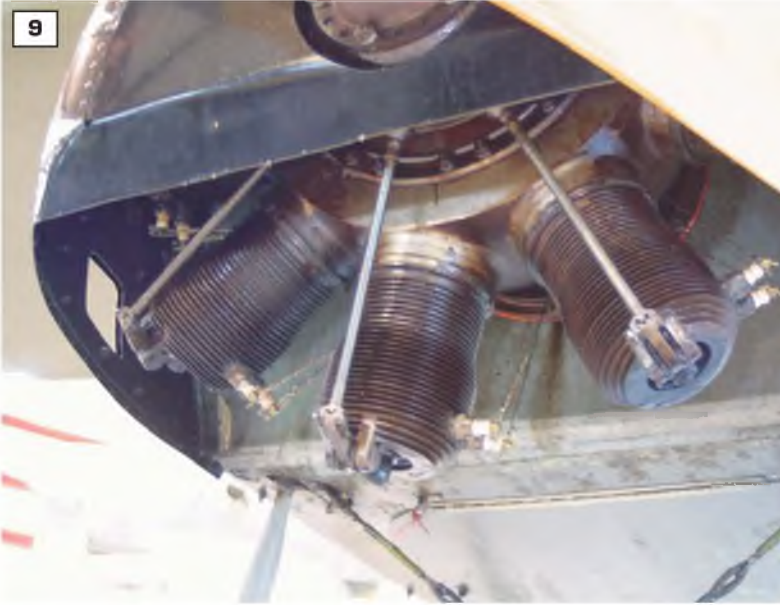
6: Cockpit rim, showing leather coaming and binding. 7: Pilot's seat and safety straps. 8: Inside the cockpit looking forward toward the instrument panel. 9: Close-up of the lower cowl showing the cylinders of the rotary engine. 10 & 11: Two views showing the cockpit windscreen and the twin Spandau machine guns. 12: The engine cowl and the access panels behind the rear cowl line.
