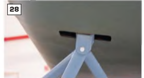
24: Lower surface of the aileron showing the control horn. 25: Close-up of the aileron control horn, control link and aileron hinge. 26, 27 & 28: Three views of the anchor point on the wing undersurface of the front wing strut. 29: Detail of the anchor point on the wing undersurface for the rear wing strut. 30: View of the undercarriage legs where they enter the undercarriage fairing viewed from the outside, looking forward. 31: View looking rearwards along the fuselage underside, from just behind the engine cowl, showing the main undercarriage cross-brace wires and fuselage access panel. 32: A look at the same components, looks rearwards toward the inside face of the wheel. Note the anchor point for the undercarriage cross-brace wire. 33: The main wheel - not known how authentic the tyre is. 34: General view of the main undercarriage, showing the struts and the cross brace wires. 35 & 36: Three views of the tail skid, which has been modified with the addition of a metal shoe that gives a degree of ground steering
