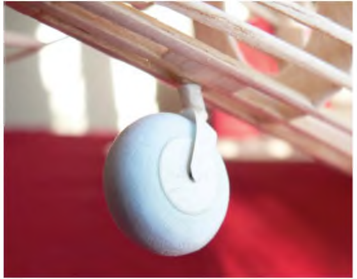
I used blue Floormate foam for the prominent tailwheel. The core is thin wire and details are from card and balsa.
