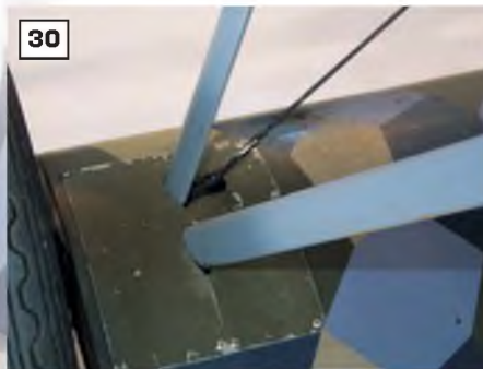
24: Lower surface of the aileron showing the control horn. 25: Close-up of the aileron control horn, control link and aileron hinge. 26, 27 & 28: Three views of the anchor point on the wing undersurface of the front wing strut. 29: Detail of the anchor point on the wing undersurface for the rear wing strut. 30: View of the undercarriage legs where they enter the undercarriage fairing viewed from the outside, looking forward. 31: View looking rearwards along the fuselage underside, from just behind the engine cowl, showing the main undercarriage cross-brace wires and fuselage access panel. 32: A look at the same components, looks rearwards toward the inside face of the wheel. Note the anchor point for the undercarriage cross-brace wire. 33: The main wheel - not known how authentic the tyre is. 34: General view of the main undercarriage, showing the struts and the cross brace wires. 35 & 36: Three views of the tail skid, which has been modified with the addition of a metal shoe that gives a degree of ground steering
