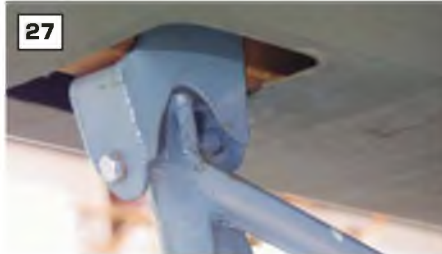
24: Lower surface of the aileron showing the control horn. 25: Close-up of the aileron control horn, control link and aileron hinge. 26, 27 & 28: Three views of the anchor point on the wing undersurface of the front wing strut. 29: Detail of the anchor point on the wing undersurface for the rear wing strut. 30: View of the undercarriage legs where they enter the undercarriage fairing viewed from the outside, looking forward. 31: View looking rearwards along the fuselage underside, from just behind the engine cowl, showing the main undercarriage cross-brace wires and fuselage access panel. 32: A look at the same components, looks rearwards toward the inside face of the wheel. Note the anchor point for the undercarriage cross-brace wire. 33: The main wheel - not known how authentic the tyre is. 34: General view of the main undercarriage, showing the struts and the cross brace wires. 35 & 36: Three views of the tail skid, which has been modified with the addition of a metal shoe that gives a degree of ground steering
