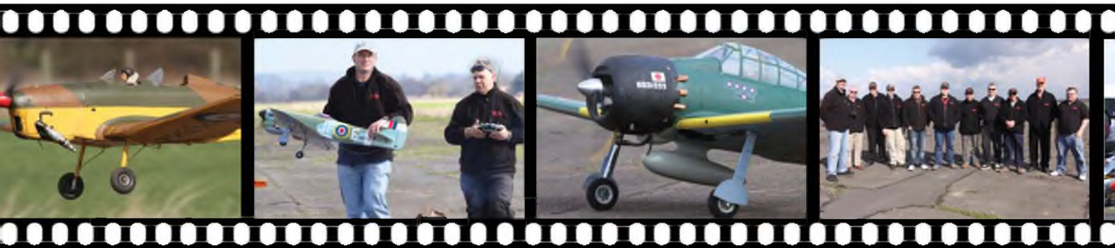
Babe Magnet Alan Griffiths' Bowman Kits Miles Magister. 90" span foam wing, ASP 180 power, weighs 17 lbs.
