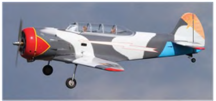
Dave Gent's Yak 11, powered by a CRRC 26 driving a 17x8 prop.
