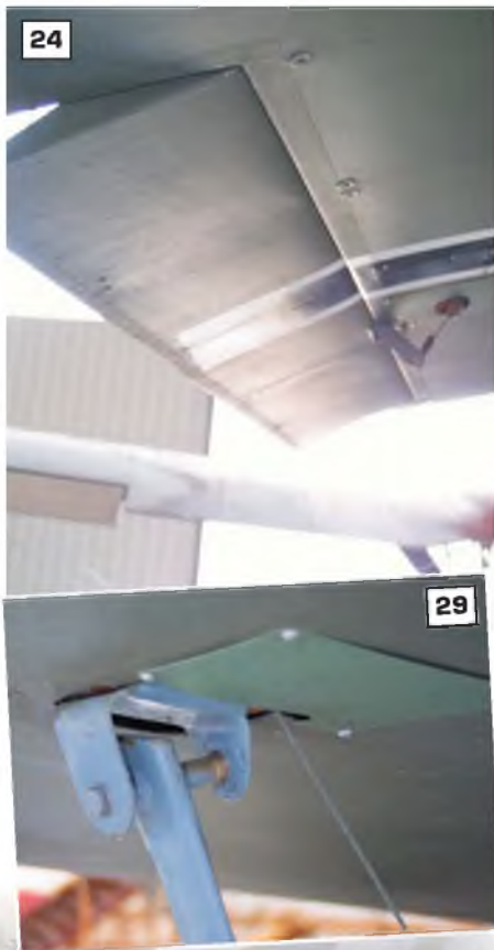
24: Lower surface of the aileron showing the control horn. 25: Close-up of the aileron control horn, control link and aileron hinge. 26, 27 & 28: Three views of the anchor point on the wing undersurface of the front wing strut. 29: Detail of the anchor point on the wing undersurface for the rear wing strut. 30: View of the undercarriage legs where they enter the undercarriage fairing viewed from the outside, looking forward. 31: View looking rearwards along the fuselage underside, from just behind the engine cowl, showing the main undercarriage cross-brace wires and fuselage access panel. 32: A look at the same components, looks rearwards toward the inside face of the wheel. Note the anchor point for the undercarriage cross-brace wire. 33: The main wheel - not known how authentic the tyre is. 34: General view of the main undercarriage, showing the struts and the cross brace wires. 35 & 36: Three views of the tail skid, which has been modified with the addition of a metal shoe that gives a degree of ground steering
