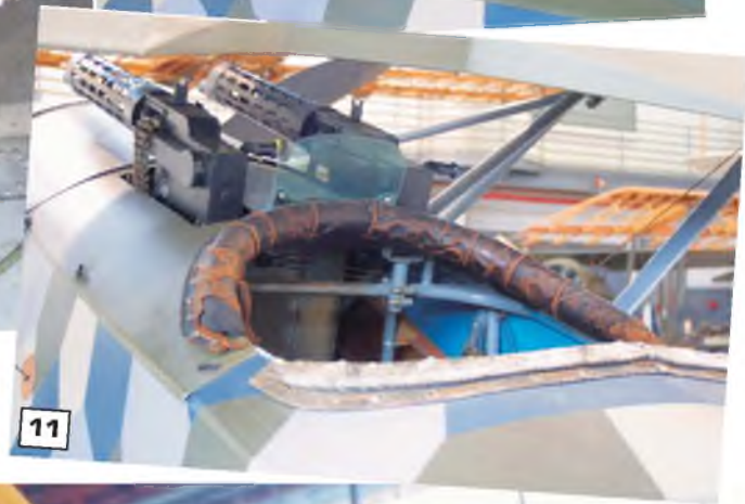
6: Cockpit rim, showing leather coaming and binding. 7: Pilot's seat and safety straps. 8: Inside the cockpit looking forward toward the instrument panel. 9: Close-up of the lower cowl showing the cylinders of the rotary engine. 10 & 11: Two views showing the cockpit windscreen and the twin Spandau machine guns. 12: The engine cowl and the access panels behind the rear cowl line.
