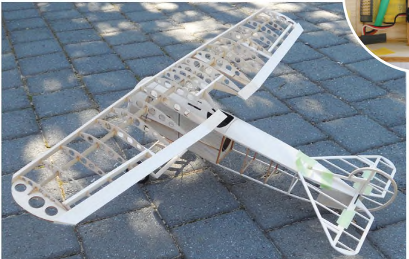
Although seen here with the aileron wing option (Simon built both wings) the little DVIII shows off the uncomplicated structure.
