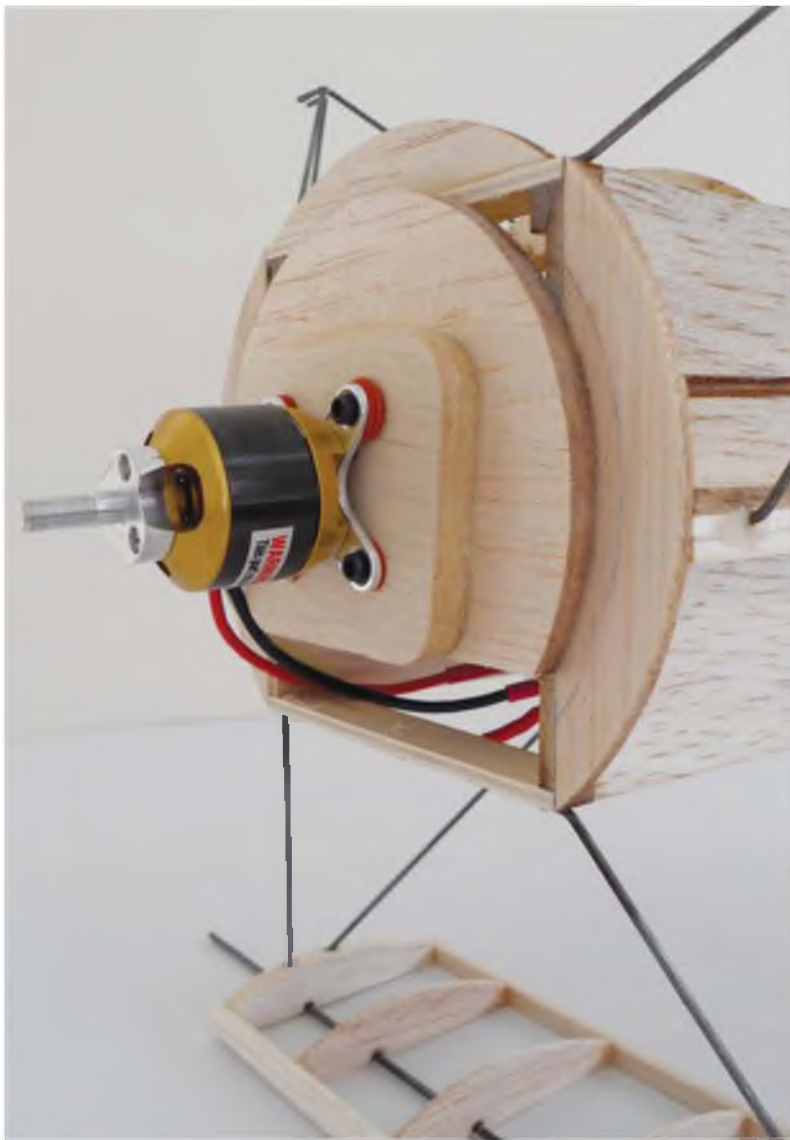
The simple modification Simon made to fit a brushless motor.
