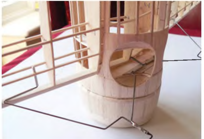
Here is the gear wire temporarily in place. I have not yet installed the gear mount plates in the wings. Note also on my model the ply reinforcement plate on the rear of former F1A is not deep enough. Use epoxy resin to glue the tubes in place.
