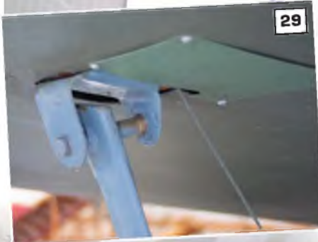
24: Lower surface of the aileron showing the control horn. 25: Close-up of the aileron control horn, control link and aileron hinge. 26, 27 & 28: Three views of the anchor point on the wing undersurface of the front wing strut. 29: Detail of the anchor point on the wing undersurface for the rear wing strut. 30: View of the undercarriage legs where they enter the undercarriage fairing viewed from the outside, looking forward. 31: View looking rearwards along the fuselage underside, from just behind the engine cowl, showing the main undercarriage cross-brace wires and fuselage access panel. 32: A look at the same components, looks rearwards toward the inside face of the wheel. Note the anchor point for the undercarriage cross-brace wire. 33: The main wheel - not known how authentic the tyre is. 34: General view of the main undercarriage, showing the struts and the cross brace wires. 35 & 36: Three views of the tail skid, which has been modified with the addition of a metal shoe that gives a degree of ground steering
