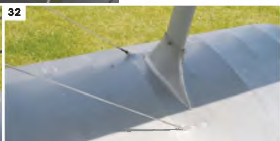
25: Further view of the tailcone. 26: Tallplane and elevator - note the aerodynamic balance. 27: View along the upper wing showing the aileron and its control rod. 28: A full close-up of the wing fairing. 29: Upper wing centre section - top side. 30: Close-up of the aileron control horn and drive rod. 31: Lower wing bracing wing anchor point. 32: Wing strut anchor point showing the streamlined fairing.
