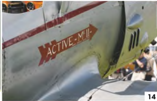
11: Tailplane, fin and rudder. Note the stitching below the fin. 12: Fuselage centre section showing the wing bracing wires and centre section wing strut anchor points. 13: Lower wing fillet and detail of wing bracing wire anchor point. 14: Further view of the lower wing fillet and louvres in the engine cowl. 15: Upper wing centre section detail. 16: Interplane wing struts and detail of the streamlined bracing wires.
