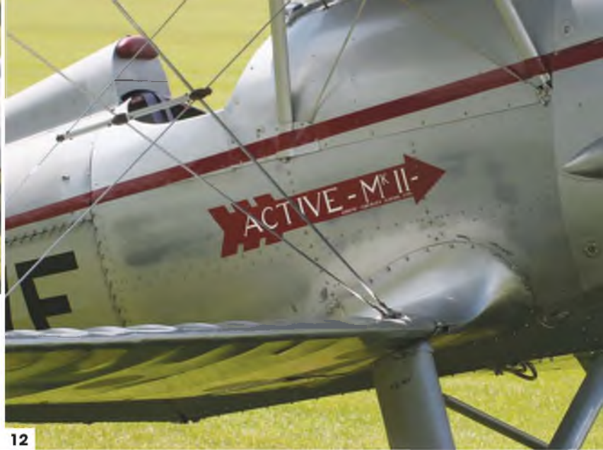
11: Tailplane, fin and rudder. Note the stitching below the fin. 12: Fuselage centre section showing the wing bracing wires and centre section wing strut anchor points. 13: Lower wing fillet and detail of wing bracing wire anchor point. 14: Further view of the lower wing fillet and louvres in the engine cowl. 15: Upper wing centre section detail. 16: Interplane wing struts and detail of the streamlined bracing wires.
