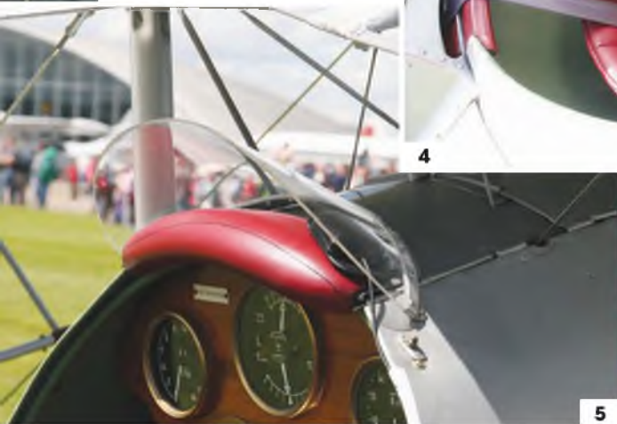
2: Profile of the cockpit rim. 3: Pilot's headrest on the top of the dorsal fuselage fairing. 4: Into the rear of the cockpit well, showing seat and pilot's safety straps. 5: View into the cockpit showing the top of the instrument panel, windscreen and padded head protector. 6: Another view into the cockpit well, showing the pilot's seat. 7-10: Details of the engine cowl, showing louves, air scoops and bulges. Note four-pipe exhaust stack in the bottom of the cowl and the oil coolers, rear of the cowl bottom panel. Centre-section struts, wing fillet and undercarriage attachment also revealed.
