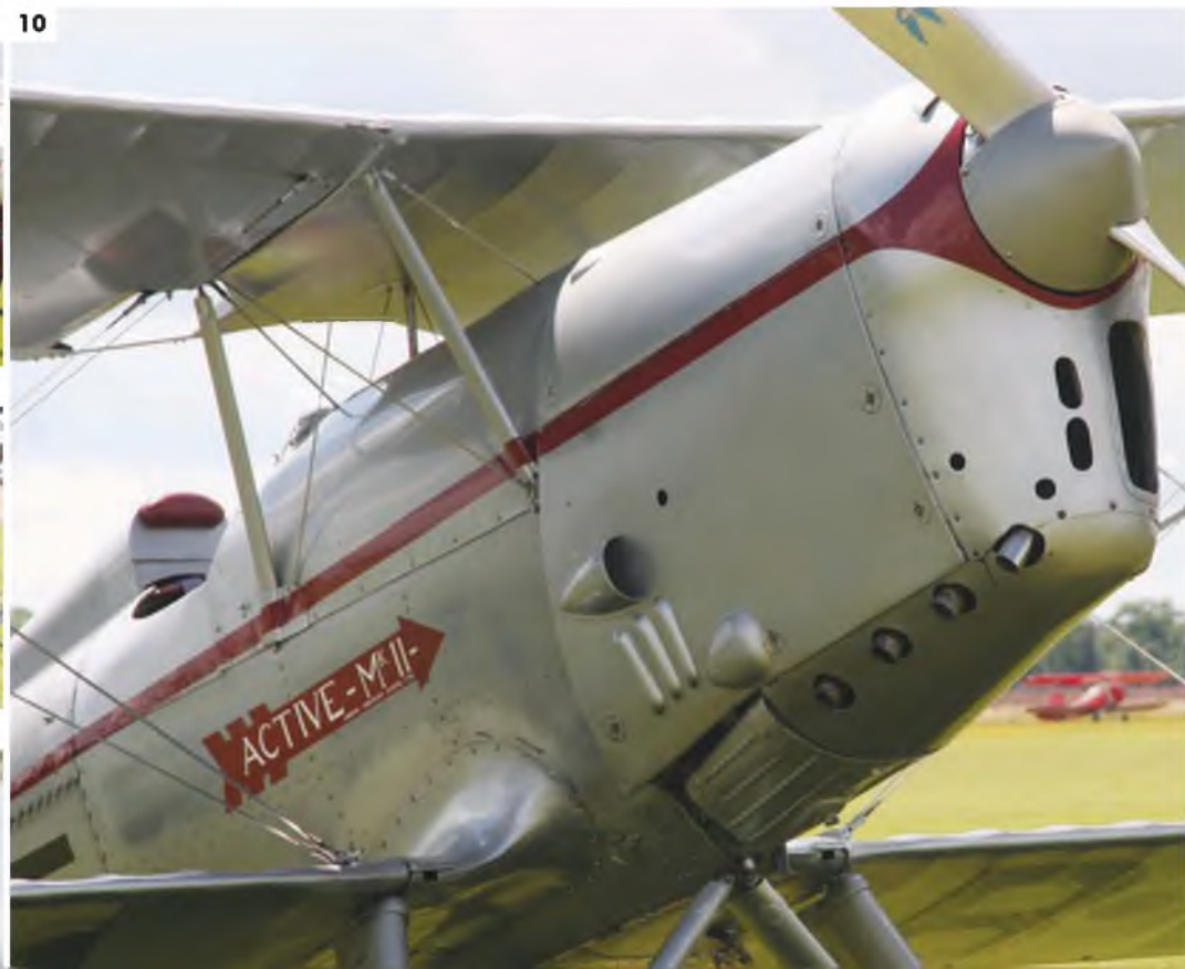
2: Profile of the cockpit rim. 3: Pilot's headrest on the top of the dorsal fuselage fairing. 4: Into the rear of the cockpit well, showing seat and pilot's safety straps. 5: View into the cockpit showing the top of the instrument panel, windscreen and padded head protector. 6: Another view into the cockpit well, showing the pilot's seat. 7-10: Details of the engine cowl, showing louves, air scoops and bulges. Note four-pipe exhaust stack in the bottom of the cowl and the oil coolers, rear of the cowl bottom panel. Centre-section struts, wing fillet and undercarriage attachment also revealed.
