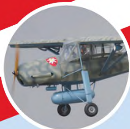
Chris Harle's beautifully finished Fieseler Storch on a typically steep approach. Laser 300 V Twin powering a 22x10 prop.
