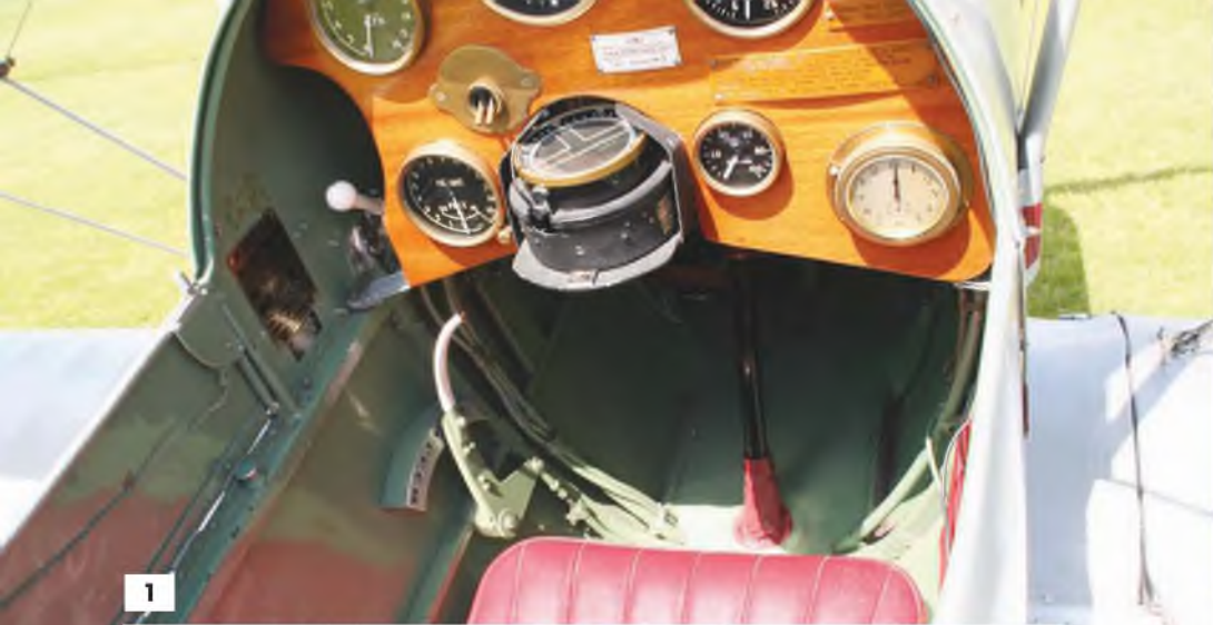
1: A view down into the cockpit well, showing instrument panel, control column and compass. Note also the hinged cockpit access door down on the left.
