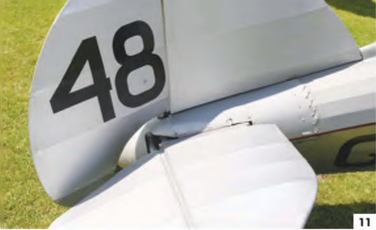
11: Tailplane, fin and rudder. Note the stitching below the fin. 12: Fuselage centre section showing the wing bracing wires and centre section wing strut anchor points. 13: Lower wing fillet and detail of wing bracing wire anchor point. 14: Further view of the lower wing fillet and louvres in the engine cowl. 15: Upper wing centre section detail. 16: Interplane wing struts and detail of the streamlined bracing wires.
