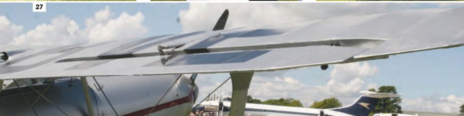
25: Further view of the tailcone. 26: Tallplane and elevator - note the aerodynamic balance. 27: View along the upper wing showing the aileron and its control rod. 28: A full close-up of the wing fairing. 29: Upper wing centre section - top side. 30: Close-up of the aileron control horn and drive rod. 31: Lower wing bracing wing anchor point. 32: Wing strut anchor point showing the streamlined fairing.
