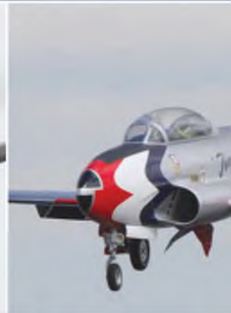
Mick Burrell's lovely Skymaster Lockheed T-33. It spans 105", weighs 10 lbs, Merlin 160 turbine power.
