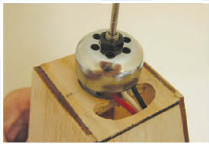
Typical of so many very cheap motors this 'bell' outrunner is great in 40-50 inch, lightly loaded monoplanes and 36-40 inch biplanes.
