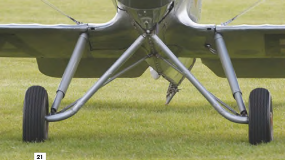
21: Full frontal view of the main undercarriage showing the oleo shock struts and main axle members. 22: Side view shows the shape of the struts. 23: Wheels hub and doughnut type tyres. 24: The main undercarriage, viewed from the rear.
