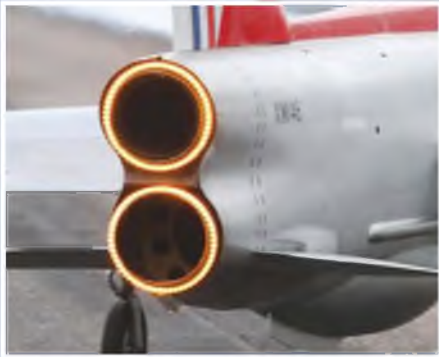
Ian Wylde has found a convincing way of simulating afterburners with these very effective LED arrays on his Lightning.
