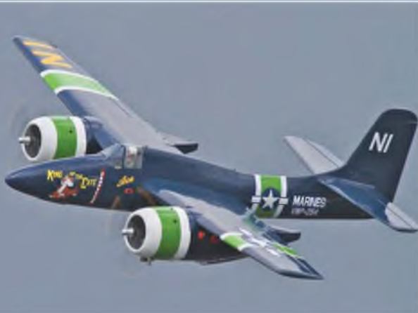
Mark Roberts' 1/8th scale King Of The Cats Grumman Tigercat F7F. 83" span, 2x DLE 20s, three-bladed props.
