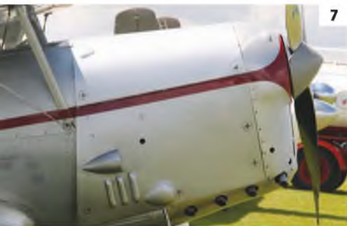
2: Profile of the cockpit rim. 3: Pilot's headrest on the top of the dorsal fuselage fairing. 4: Into the rear of the cockpit well, showing seat and pilot's safety straps. 5: View into the cockpit showing the top of the instrument panel, windscreen and padded head protector. 6: Another view into the cockpit well, showing the pilot's seat. 7-10: Details of the engine cowl, showing louves, air scoops and bulges. Note four-pipe exhaust stack in the bottom of the cowl and the oil coolers, rear of the cowl bottom panel. Centre-section struts, wing fillet and undercarriage attachment also revealed.
