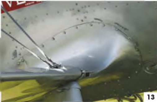
11: Tailplane, fin and rudder. Note the stitching below the fin. 12: Fuselage centre section showing the wing bracing wires and centre section wing strut anchor points. 13: Lower wing fillet and detail of wing bracing wire anchor point. 14: Further view of the lower wing fillet and louvres in the engine cowl. 15: Upper wing centre section detail. 16: Interplane wing struts and detail of the streamlined bracing wires.
