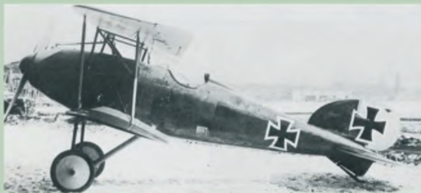
ABOVE: Only a single example of the Albatros D.IV is believed to have been built. It was used as a test-bed for a special geared version of the Mercedes D.III engine the profile of which allowed the engine to be fully enclosed with the fuselage profile.
