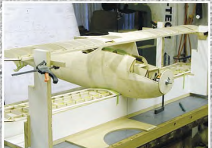
The model mounted in a jig in preparation for precise fitting of centre section struts, interplane struts and tail surfaces. If you get this right, everything else has to be right.
