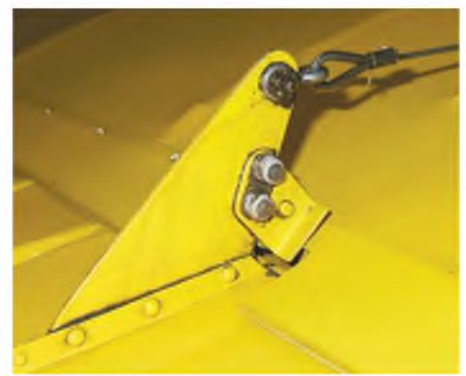
The port top aileron horn ('Pull-pull' is used throughout).
