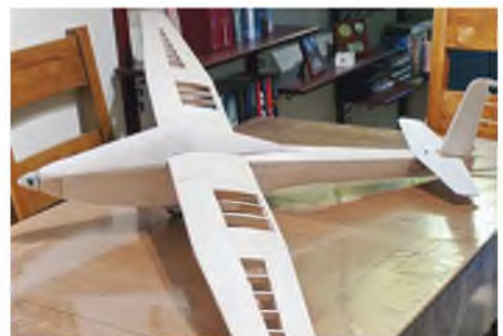
The airframe, ready for covering.
