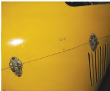
Starboard engine cover (sheet aluminium) with fastenings and louvres.
