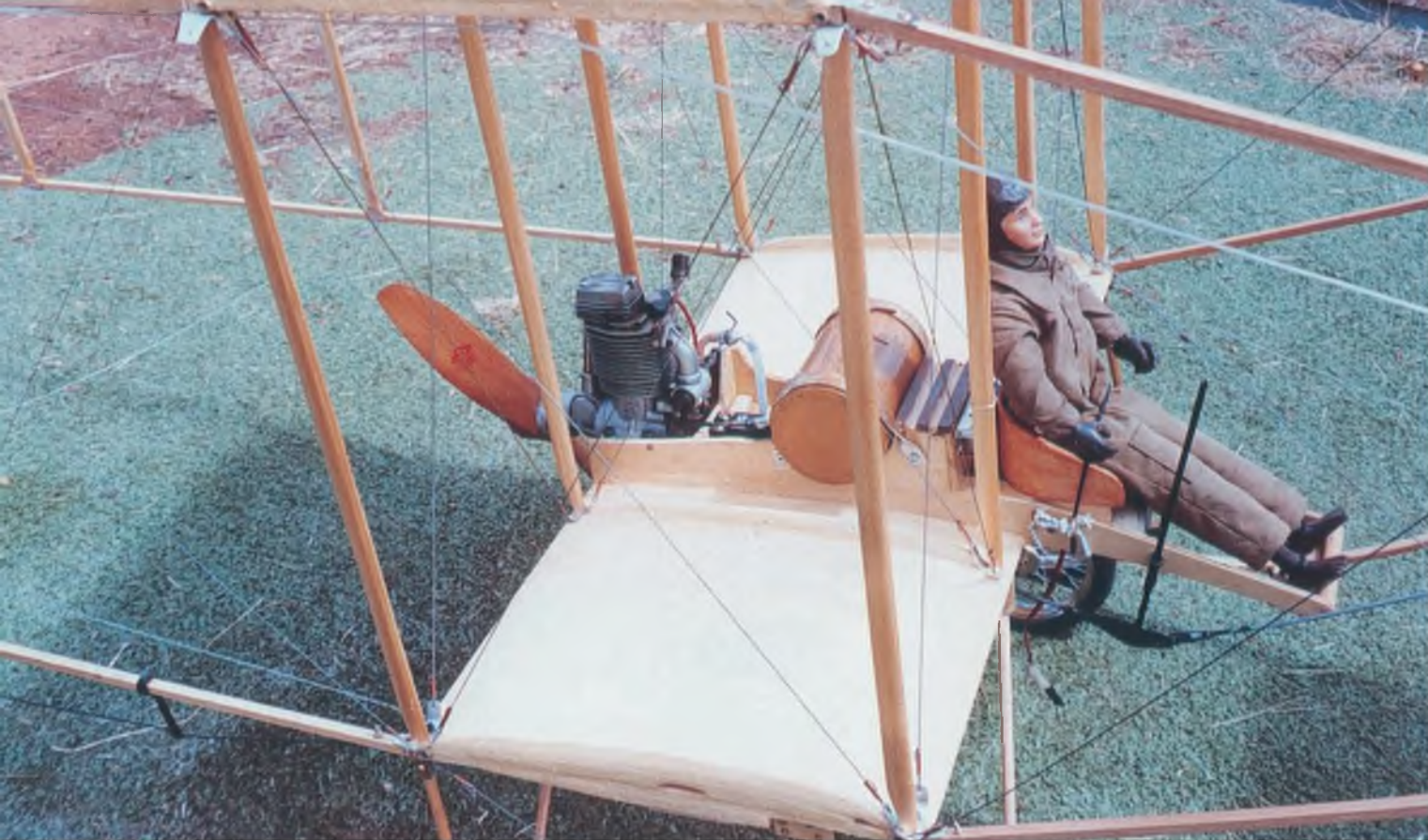
READY FOR THE FIRST FLIGHT AT BACCHUS MARSH CLUB FIELD. THE ENGINE IS NOW UPRIGHT AND THE FUEL TANK FORWARD. NOTE THE RECEIVER AERIAL AT LOWER LEFT, TRAILING BELOW THE TAILBOOM AND SUSPENDED FROM PLASTIC TIES.
