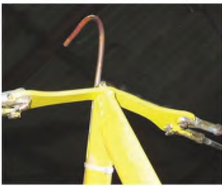
King-post with pitot tube and flying wires attached.
