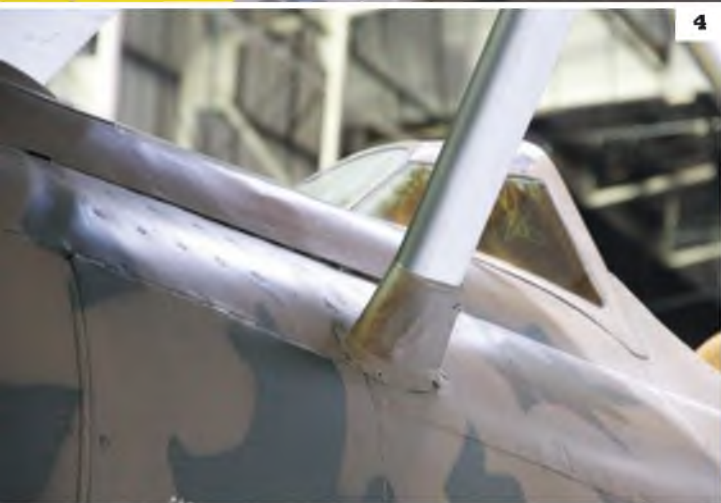
1: Centre section struts are fully streamlined and substantial. 2: Close-up of the centre section struts upper anchor-point showing the cuff fairings. 3: Lower centre section strut anchor-point. 4: Wing strut lower anchor point and cockpit windscreen. 5 & 6: Two views of the fully faired interplane struts. 7 & 8: Two views of the cockpit and windshield.
