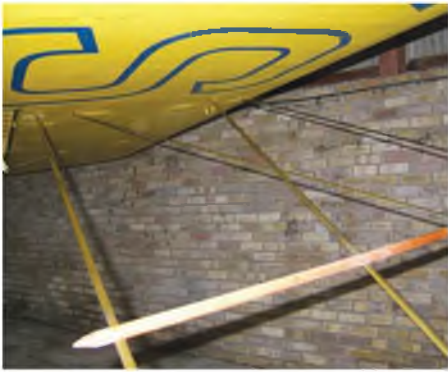
Port streamlined wing bracing wires and wooden dowel spacer (anti-vibration?).
