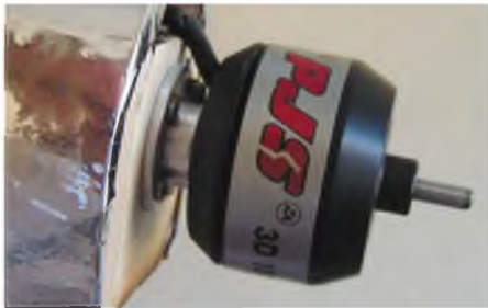
One of those strangely labelled motors, but a good indication of an alternative style of radial mount.
