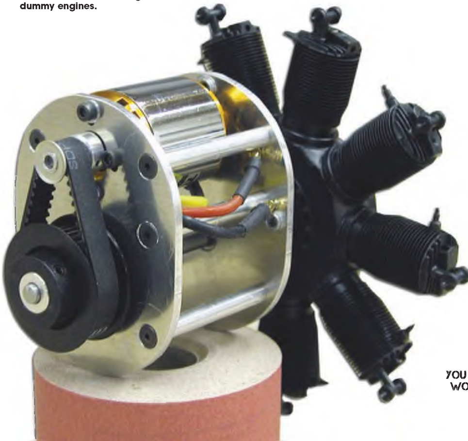
The compact nature of outrunners make them ideal for concealing within dummy engines.
