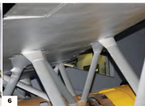
1: Centre section struts are fully streamlined and substantial. 2: Close-up of the centre section struts upper anchor-point showing the cuff fairings. 3: Lower centre section strut anchor-point. 4: Wing strut lower anchor point and cockpit windscreen. 5 & 6: Two views of the fully faired interplane struts. 7 & 8: Two views of the cockpit and windshield.
