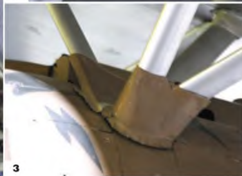
1: Centre section struts are fully streamlined and substantial. 2: Close-up of the centre section struts upper anchor-point showing the cuff fairings. 3: Lower centre section strut anchor-point. 4: Wing strut lower anchor point and cockpit windscreen. 5 & 6: Two views of the fully faired interplane struts. 7 & 8: Two views of the cockpit and windshield.
