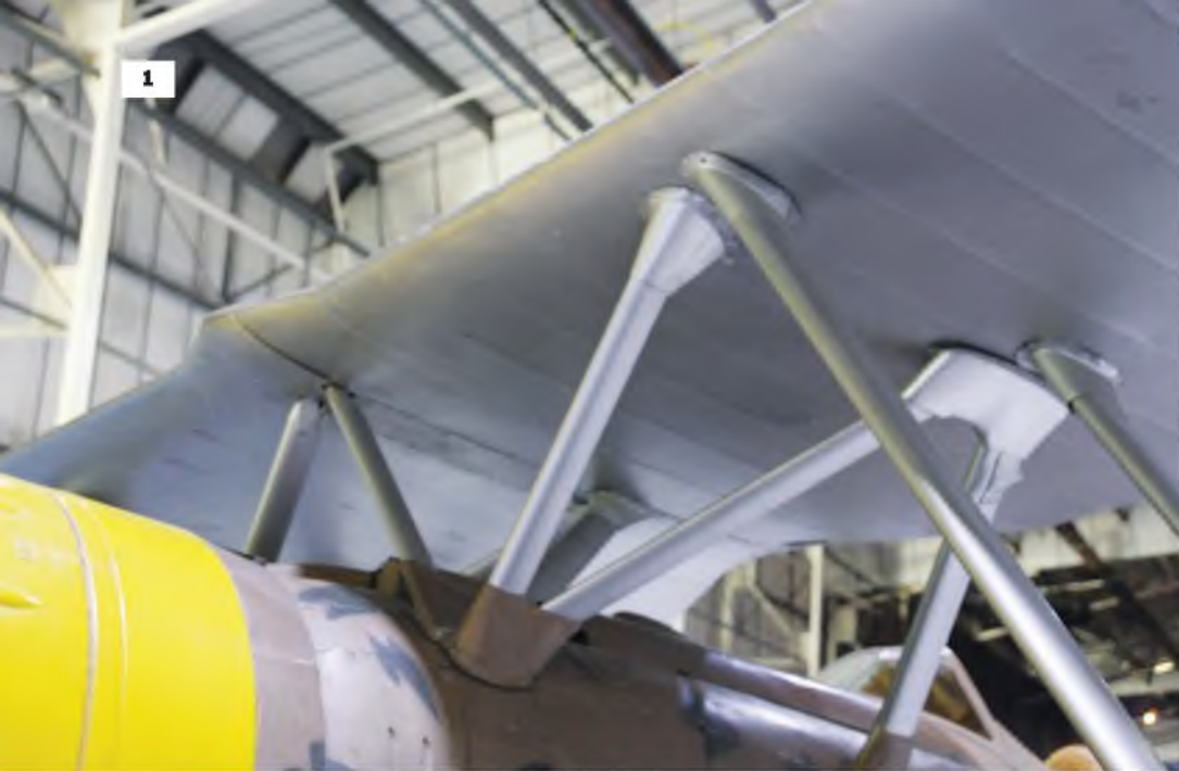
1: Centre section struts are fully streamlined and substantial. 2: Close-up of the centre section struts upper anchor-point showing the cuff fairings. 3: Lower centre section strut anchor-point. 4: Wing strut lower anchor point and cockpit windscreen. 5 & 6: Two views of the fully faired interplane struts. 7 & 8: Two views of the cockpit and windshield.
