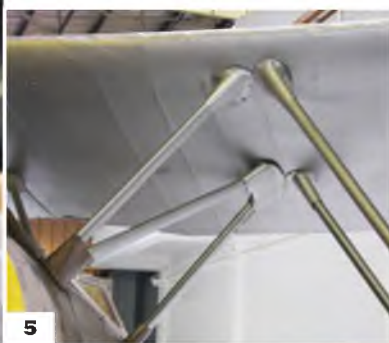
1: Centre section struts are fully streamlined and substantial. 2: Close-up of the centre section struts upper anchor-point showing the cuff fairings. 3: Lower centre section strut anchor-point. 4: Wing strut lower anchor point and cockpit windscreen. 5 & 6: Two views of the fully faired interplane struts. 7 & 8: Two views of the cockpit and windshield.
