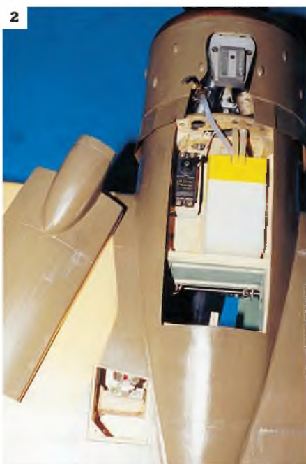
1: Detail of the removable top hatch behind the cockpit, showing the air reservoir tank feeds the air driven retracting undercarriage. The main radio installation is also seen here.
