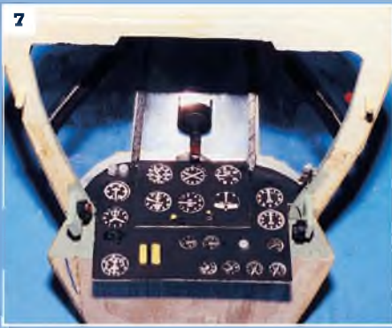
7: Cockpit instrument panel made by sandwiching photocopied instruments between clear acetate and 'authenticated' with a little application of 'wear-and-tear'.
