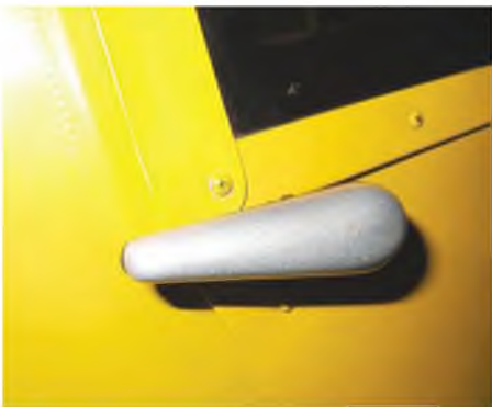
Streamlined 1930s cabin door handle in natural aluminium - note pinking-shears finish on Ceconite fabric overlap.
