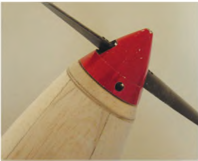
With a nose this restrictive, there is still a time when direct drive brushed motors have their advantages.
