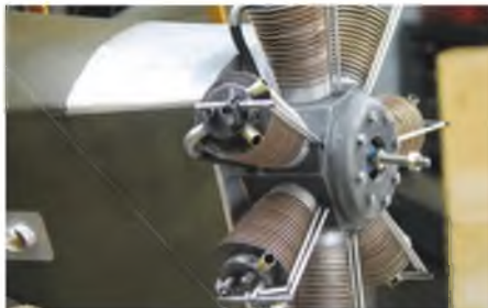
The compact nature of outrunners make them ideal for concealing within dummy engines.
