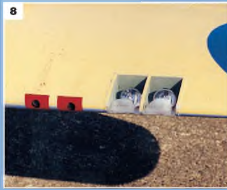
8: Left wing leading edge showing dummy landing lights and gun ports. 9: Dummy radial engines made from bath overflow pipe. Crankcase centre from yoghurt pot.
