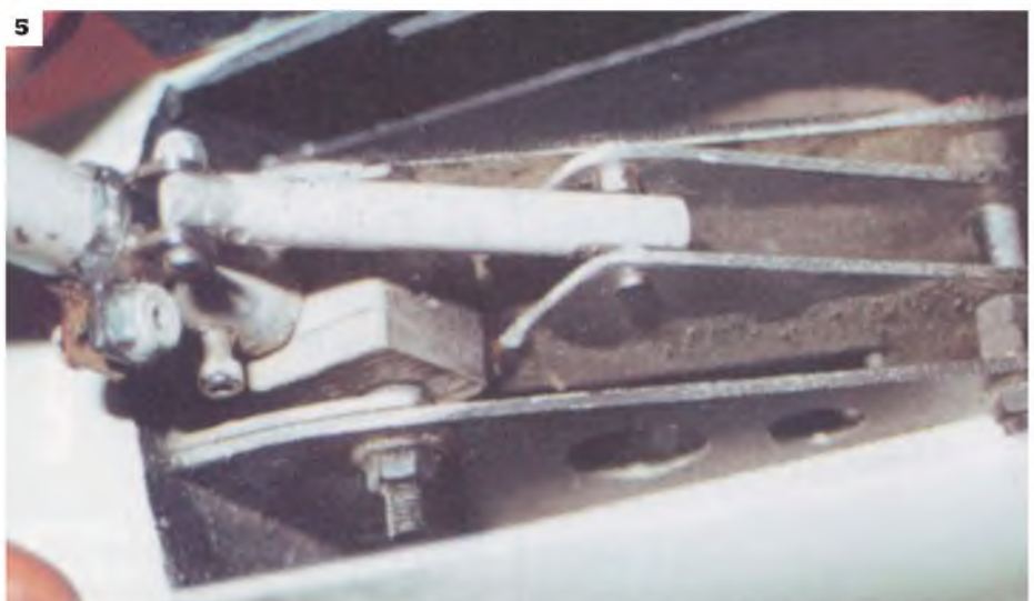
5: Close-up of the undercarriage mechanism as installed.
