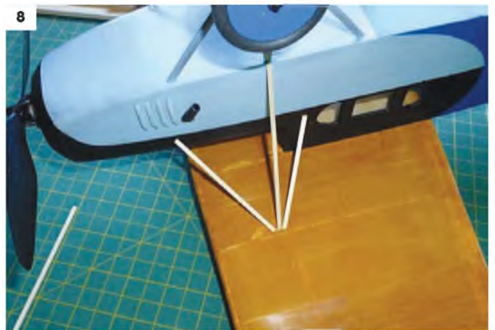
5: The fuselage is a simple sheet and strip balsa box. All very basic and straightforward. 6: After a bit of planning and sanding the upper hatch takes shape. The passengers may have been inside, but the poor pilots were still exposed to the elements. 7: There you have it, a Fokker F.II all ready to cover. Model structures don't get much simpler than this. 8: The struts are purely cosmetic and glued in place after the model is assembled.
