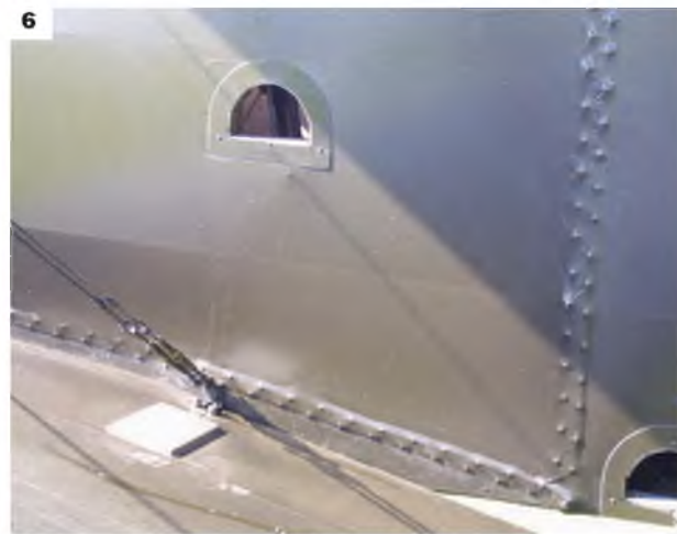
4, 5 & 6: The Shuttleworth Collection's Avro 504K is an example of the instance in which the lacing runs have been taped over, and which thus have to be removed to allow the lacing to be undone to allow maintenance work to be carried out.
