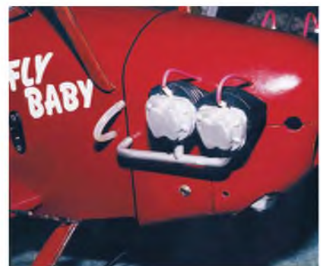
With this size of model, the dummy flat-four engine just has to be accurately replicated. For four cylinders, it is worth making a mould for the cylinder heads. If you have the skill to do it.
