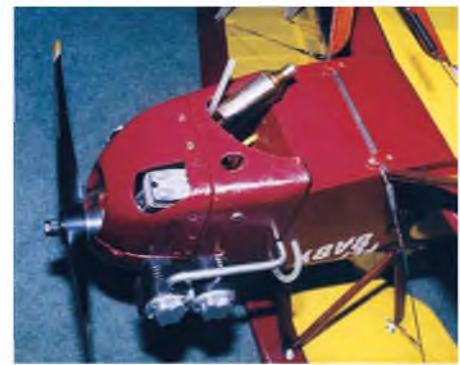
The SC.91 four-stroke fits nicely into the cowl with just a cooling hole to clear the rocker cover. Note the wing rigging wire fitting that passes under the undercarriage front leg clamp plates.
