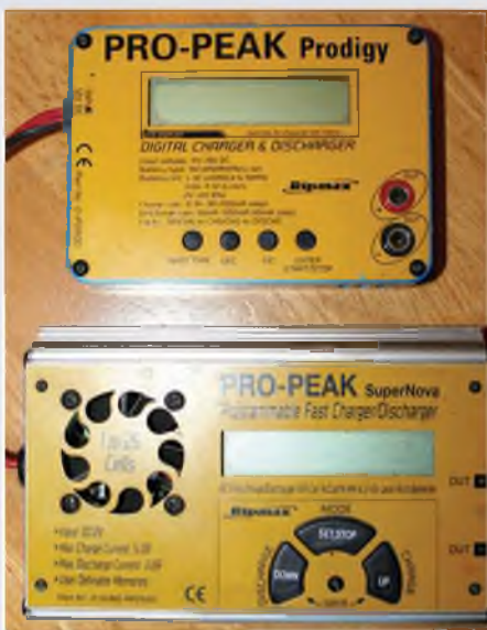
Two similar, multi purpose chargers from the mid-price range. Both will charge just about anything you want, but you can go more or less technical if all you want is to charge LiPo packs.
