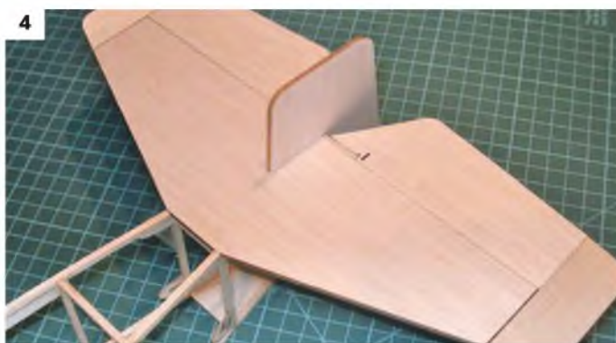
1: Begin the wings by joining the spars with the dihedral brace, and then build the centre section. 2: Lower the spar over the plan and build a wing panel. Repeat for the opposite side. 3: A complete wing, all sanded and ready to cover. 4: Nothing at all complicated about the tail surfaces. Note the dowel joiner and the grain on the elevator balances. Also visible are the cable exits.
