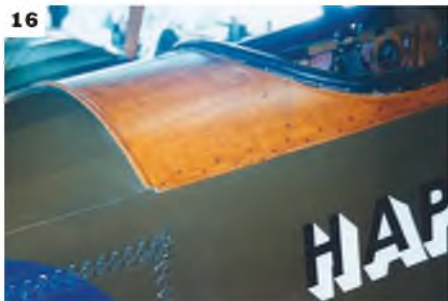
13, 14, 15 & 16: Sopwith Pup and Sopwith Triplane seem to feature very neat and unobtrusive lacing runs. The laced leather cockpit rim shown is on the Sopwith Triplane.
