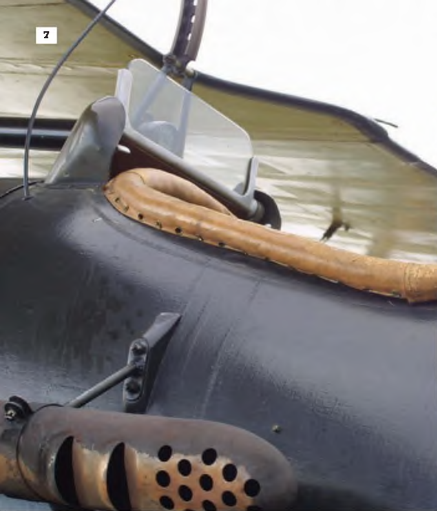
7, 8, 9, 10, 11 & 12: The Shuttleworth Collection's SE5a is another example in which the lacing runs have been taped over. Pictures here also illustrate the laying-and-eyelet binding of the leather cockpit rim surround.
