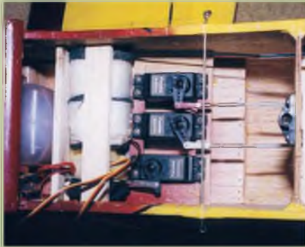
Not exactly short of space in the cavernous equipment bay! Note that the rigging wire fitting extends across the full width of the fuselage to spread the load. Note also that there is no dowel location for the lower wing - Mike finds the notched leading edge more than adequate - and allows for shock absorption in the case of a cartwheel.
