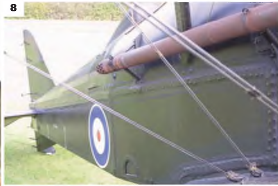
7, 8, 9, 10, 11 & 12: The Shuttleworth Collection's SE5a is another example in which the lacing runs have been taped over. Pictures here also illustrate the laying-and-eyelet binding of the leather cockpit rim surround.
