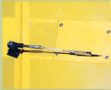
The aileron servos are mounted in the lower wing. Note ball-joint horn arm used because of the swept-back hinge line. The linkages are nicely short too.
