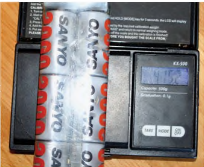
The 7 cell Ni-Cad (yes, I do still have some) was state of the art in its day, but weighed in at a whopping 415 grams. The similar LiPo weighs well under a quarter of that.
