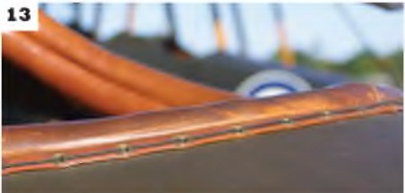
13, 14, 15 & 16: Sopwith Pup and Sopwith Triplane seem to feature very neat and unobtrusive lacing runs. The laced leather cockpit rim shown is on the Sopwith Triplane.
