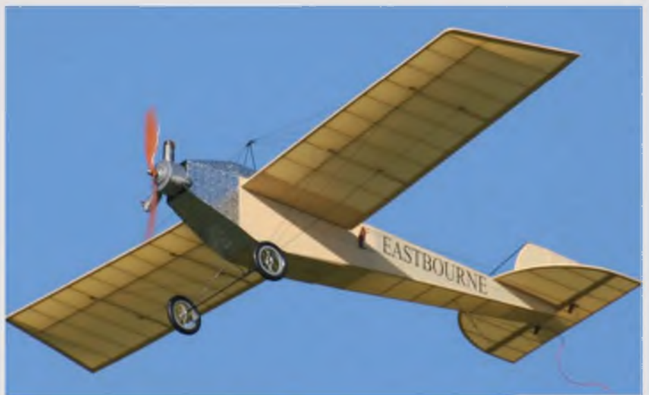
Careful matching of the power train resulted in ample power and 30 minute flight times on this 48", 20 ounce model. It really is worth taking the time to get it right.
