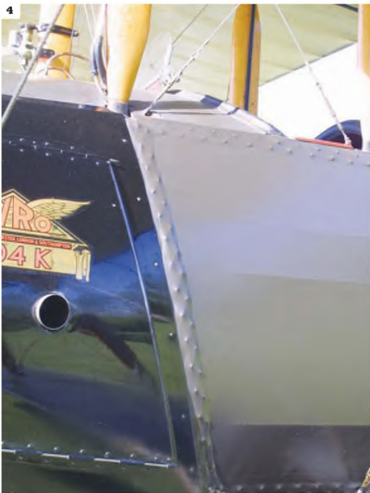
4, 5 & 6: The Shuttleworth Collection's Avro 504K is an example of the instance in which the lacing runs have been taped over, and which thus have to be removed to allow the lacing to be undone to allow maintenance work to be carried out.
