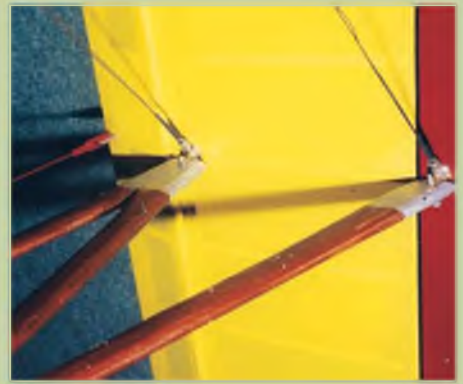
The interplane strut fittings are standard Ripmax clevises bonded into the wing - the strut ends fit onto the clevis end, secured with a screw through strut into the tapped clevis arm. The rigging wires are attached to piano wire 'S' hooks. Which wrap around the clevis.
