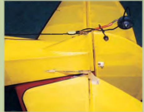
The tail end linkages are strictly traditional and present no problem. Note the wire guide on the rudder for the steerable tailwheel - minimal loads are transmitted to the rudder in this manner.
