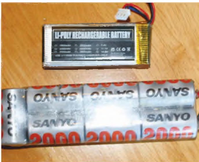
Of similar capacity, and only just over 1 volt difference, which lump would you sooner fit to your model?
