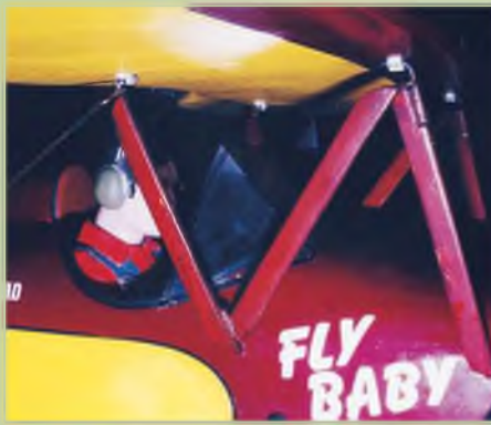
The top wing location is via four saddle clamps, one on each cabane wire. Slipping the wires in and out of the saddle clamps smoothly, involves a certain amount of trial and error, but make fitting the top wing very easy, once achieved.
