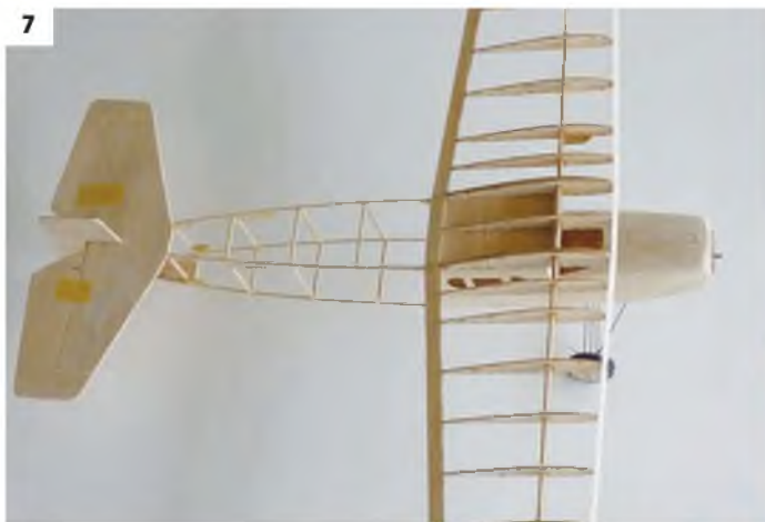
5: The fuselage is a simple sheet and strip balsa box. All very basic and straightforward. 6: After a bit of planning and sanding the upper hatch takes shape. The passengers may have been inside, but the poor pilots were still exposed to the elements. 7: There you have it, a Fokker F.II all ready to cover. Model structures don't get much simpler than this. 8: The struts are purely cosmetic and glued in place after the model is assembled.
