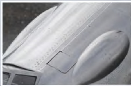
All blisters and hatches are moulded in at the factory.
