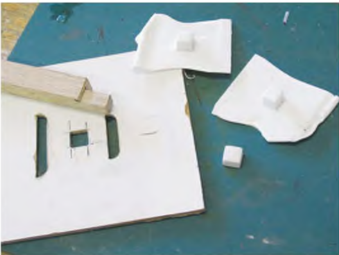
Here you see the forms for round counter boxes and louvers, along with a couple of demonstration boxes.
