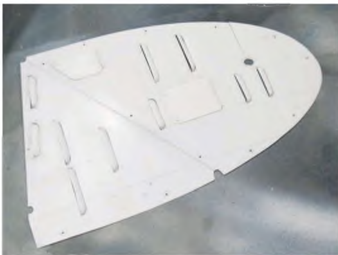
Once the louvers are fitted, a few panel lines scored on and some sheet plastic access panels added the side panels really begin to look the part.
