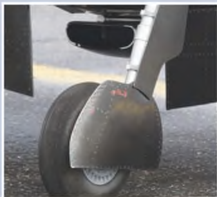
The leg detailing is impressive. Mick altered the retracts to hydraulic operation.
