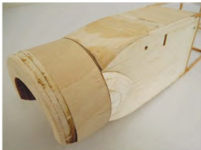
Only glue the fairing blocks to the cowl during the shaping process. It makes finishing the cowl a whole lot less fraught.
