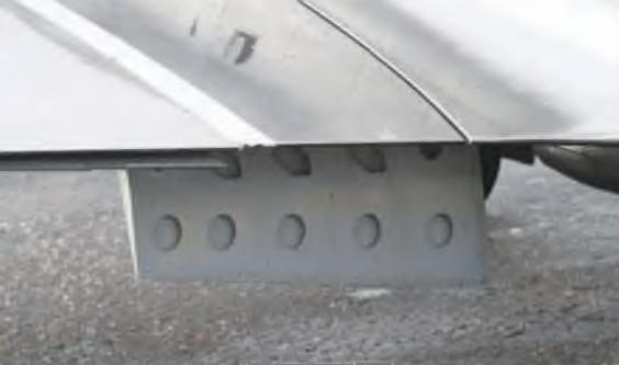
Rivet and lightening hole detail on split flap.
