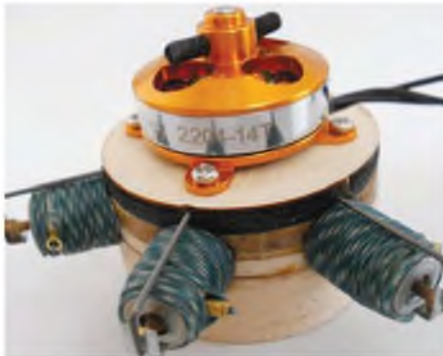
A simple partial engine fits easily behind the motor and fills the lower cowl nicely.
