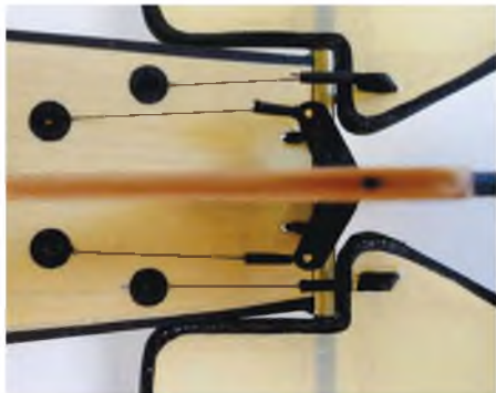
How the closed loop cables exit the lower fuselage. An aluminium, or even plastic, elevator hinge tube makes balancing easier.
