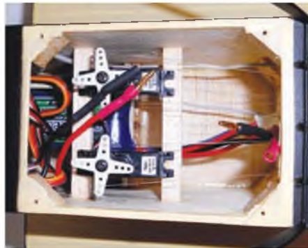
Not huge amounts of room in the avionics bay, but enough to do the job. Make sure you get everything as far forward as possible.
