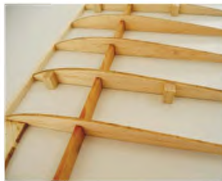
In retrospect, I'd probably recommend making the grain in the rigging blocks run chord wise. It prevents the rigging cutting into the grain.
