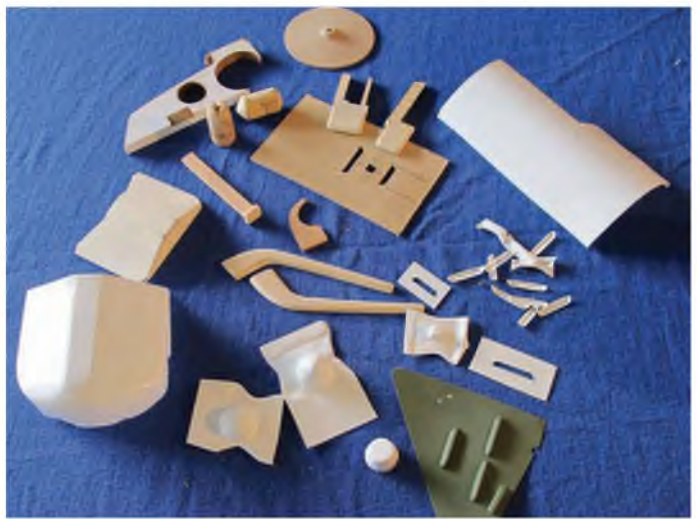
A selection of formed parts and some of the forms used to produce them demonstrate just how well this low-tech approach can work.
