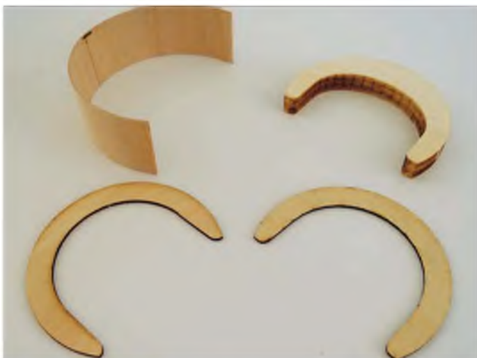
Pre-curving the ply for the cowl makes assembly so much easier.
