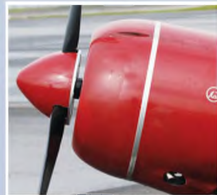
Collector ring on engine means that the engine cowling is unsullied by model exhaust cut-outs. Note 'La7' legend in cyrillics.
