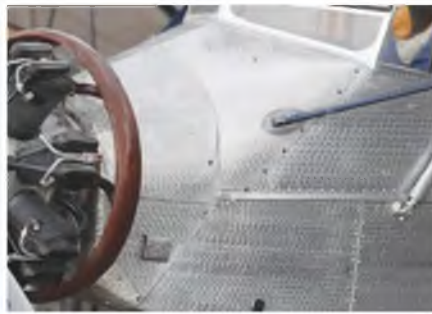
Meticulous engine-turned panels, plus varieties of rivets and fasteners.
