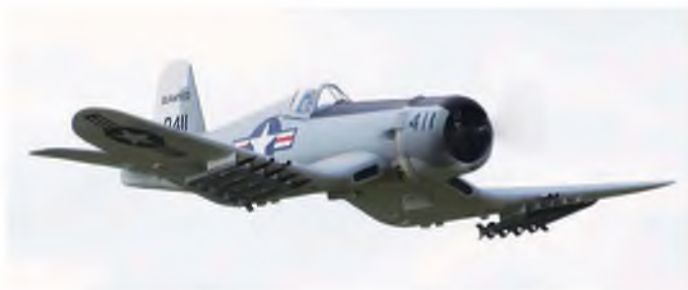
The rockets on Gary Mills Chance Vought AU-1 Corsair just look cool! 100"WS, 53#'s, Moki 150.
