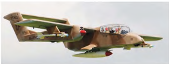
David Hart, who provided many of the brilliant photos for this article, got this shot of my North American OV-10 Bronco coming by for a pass. Rich Uravitch design, 109"WS, 52 lbs, 2 X Hacker A60's on 12S.
