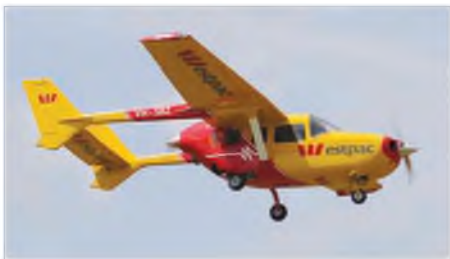
John Boyko had a lot of heart in his Cessna Skymaster 337 and fought a few obstacles to get it to the flight line. A few gremlins are still being sorted on this completely scratch built, own designed Master Class entry. Not surprising considering the complexity of the subject, I am sure John is busily sorting the gremlins out now for Top Gun 2013! 2 x Moki 1.50's, 120"WS, 40#s.
