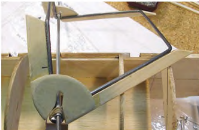
Ply plates on Tim's model keep the sprung axle in place. See text for an alternative method.
