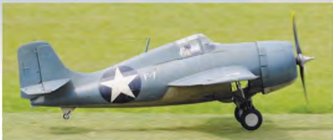
Kyle Goodwine flew this Grumman F4F Wildcat for the Unlimited Team Goodwine. Built from Bates plans and powered by a Moki 150, this plane weighted in at 42#'s, 92"WS.
