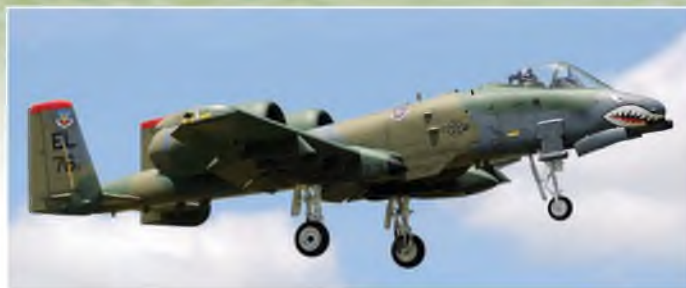
Greg Foushi flies his Skymaster Fairchild-Republic A-10 like it should be flown - low and slow! Jetcat P80 x 2, 110"WS, 55 lbs.
