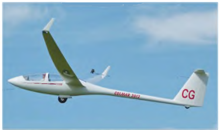
Chris Garrod's ASH 25 preserving the on-board batteries by means of an aerotow launch.
