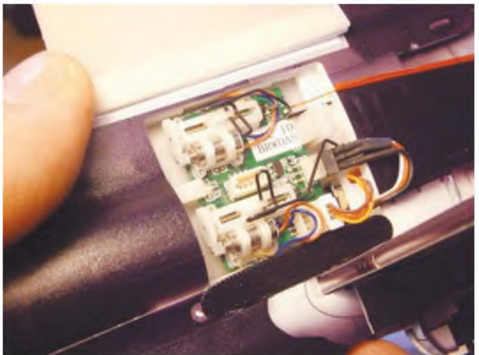
Here you see how the stickers and various other parts work together to virtually hide the unsightly linkages and servo lead. It also reveals some of that instruction manual.
