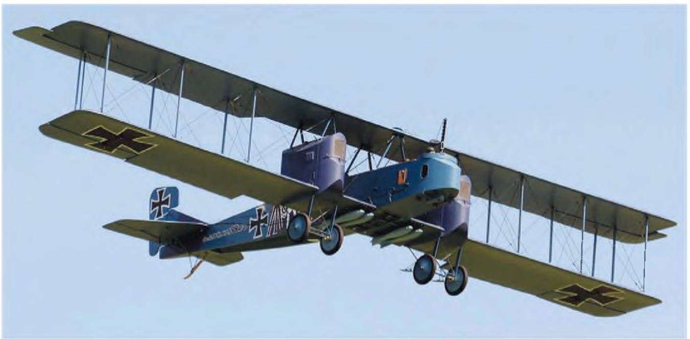
Talk about GIANT. This WWI Gotha Bomber was flown by Jim Suchy in Pro- Am Sportsman. At 192", I believe it holds the record for largest wingspan ever at Top Gun! 2 x Zenoah G-38, 52 lbs.
