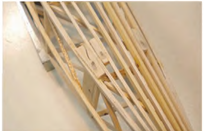
Once you've determined where you control cables will exit the fuselage scrap balsa supports the nylon tube exits.
