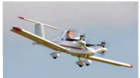
Not too many half scale models on the competition circuit and I am willing to bet this is the smallest of them! 96" WS, 24#s, AXI 4120-18 x 2.
