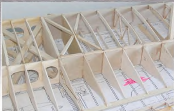
The first will panel of the basic wing. Note the 'W'-braced centre sections of the ribs. It is designed for lightness, without loss of airframe strength.
