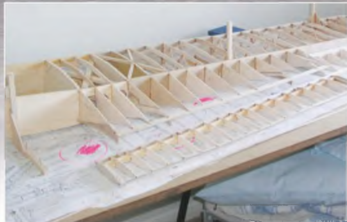
A further view of the right hand wing panel, also showing the flap sub-assembly.
