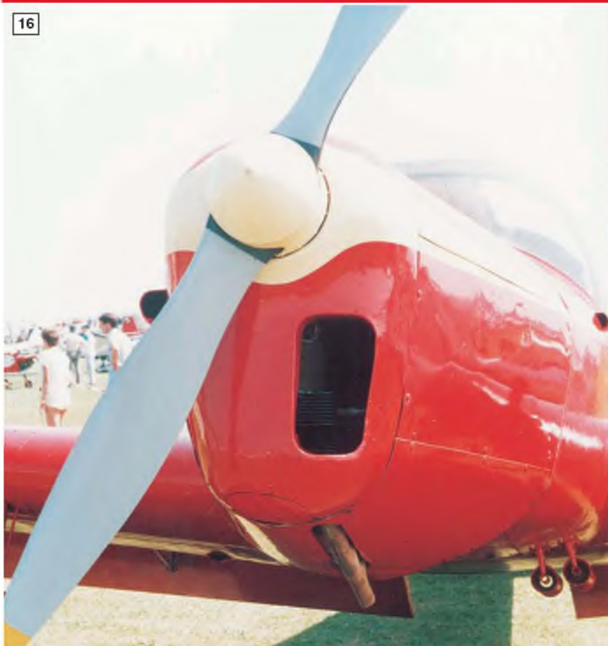
11-13: The cockpit/passenger cabin is a prominent feature of the Myles Messenger, so needs much attention. These views show the individual glazed panels. 14: Detail of the hinges of the cockpit hatches that hinge upwards. 15: The tailwheel unit. 16 & 17: Two views of the engine cowling showing panel lines and air intakes. 18: Profile of the propeller spinner.
