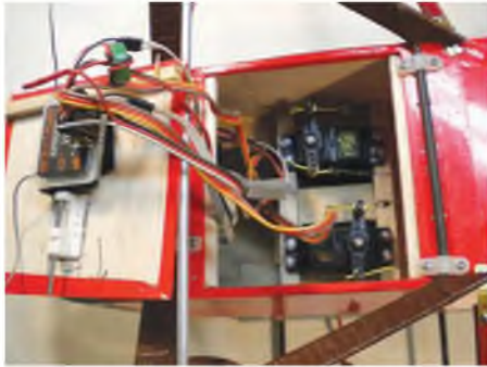
Saddle clamps are a good u/c mounting alternative, as it Tim's radio access hatch. There's no shortage of space for the gear.
