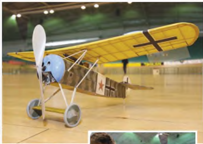
ABOVE: Peter Fardell's new Fokker E.V 20.5" span, weighs 40 grams. RIGHT: Peter's Fokker E.V was made from the Aerowekes kit. 2 loops of 1/8" rubber for power.
