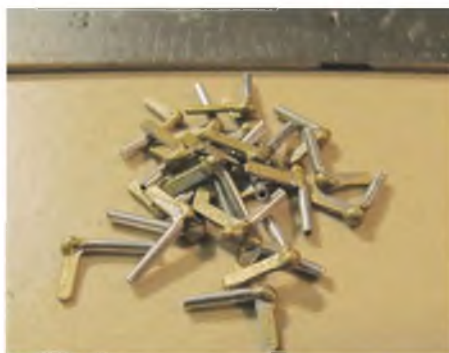
A multitude of Fokker nuts. The idea is that they work like weather vanes - the slipstream prevents them unscrewing if they come loose.
