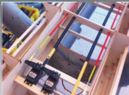
Servo installation and control snakes installed whilst access is good.
