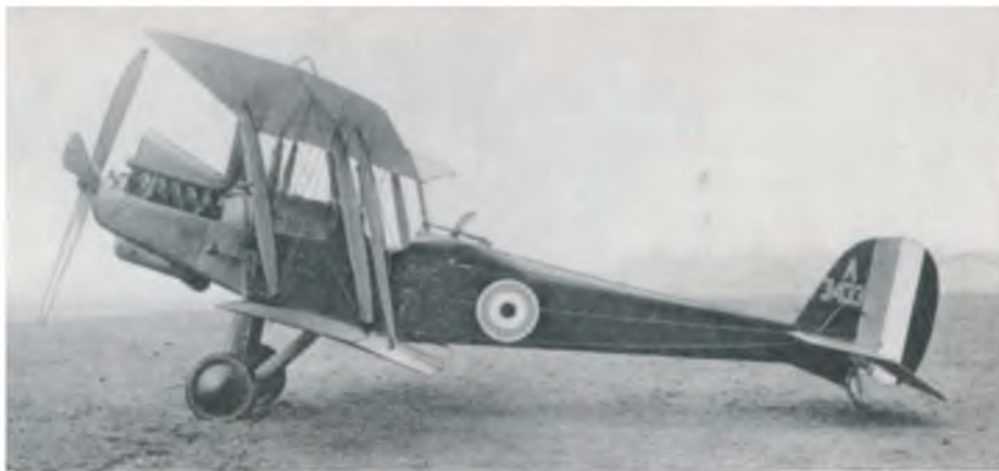
ABOVE LEFT: This very early R.E.8 has the original fin shape, with triangular underside sub-fin in front of the the tailskid. ABOVE RIGHT: One of the extremes of fin area revisions applied to the R.E.8, this one, in May 1917 is all of 12 sq.ft. in area.
