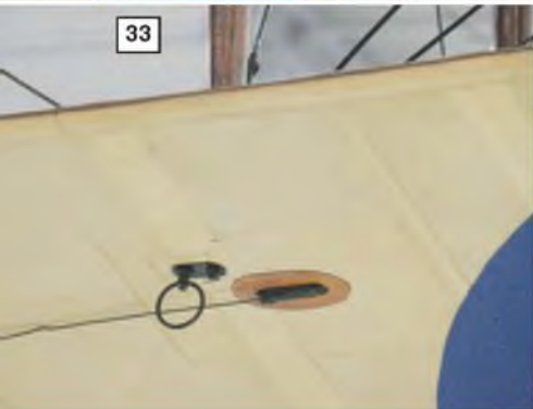
30, 31 & 32: General views showing the arrangement of bracing wires. 33: Aileron control cable runs externally from the fuselage, along the wing underside before feeding into the outer wing. 34: Another view of the fuselage centre section from the wing underside, showing the wing cut-outs to facilitate downward clear vision. 35: Bomb racks on the lower wing underside - four per wing panel. Note also, again, the aileron control run along the wing panel underside. 36: Detail of the main undercarriage rear strut mounting point. Note also the aileron control crank linked to its control cable. 37: Detail of the main undercarriage front strut mounting point. 38: Front profile of the main wheel. 39: A full view of the main undercarriage. 40: Mainwheel and axle close-up.
