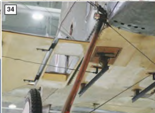
30, 31 & 32: General views showing the arrangement of bracing wires. 33: Aileron control cable runs externally from the fuselage, along the wing underside before feeding into the outer wing. 34: Another view of the fuselage centre section from the wing underside, showing the wing cut-outs to facilitate downward clear vision. 35: Bomb racks on the lower wing underside - four per wing panel. Note also, again, the aileron control run along the wing panel underside. 36: Detail of the main undercarriage rear strut mounting point. Note also the aileron control crank linked to its control cable. 37: Detail of the main undercarriage front strut mounting point. 38: Front profile of the main wheel. 39: A full view of the main undercarriage. 40: Mainwheel and axle close-up.
