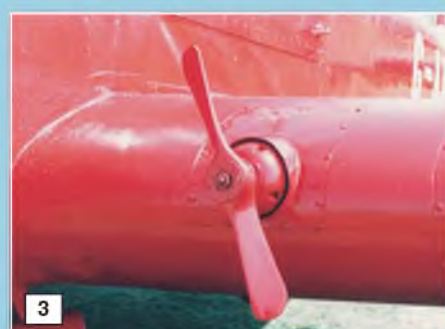
1 & 2: Two views of the outer aileron hinge. Inner hinge similar. 3: Propeller driven generator at the left wing leading edge. 4: Cockpit windows and glazing, also showing the cockpit access tread mat and the foot step, let into the flap. Also shows the wing-to-fuselage fairing.
