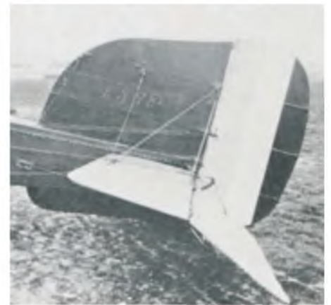
ABOVE LEFT: This very early R.E.8 has the original fin shape, with triangular underside sub-fin in front of the the tailskid. ABOVE RIGHT: One of the extremes of fin area revisions applied to the R.E.8, this one, in May 1917 is all of 12 sq.ft. in area.
