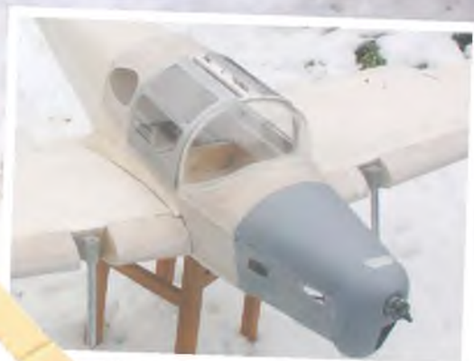
Glass fibre moulded cowl on Peter Shaw's model.
