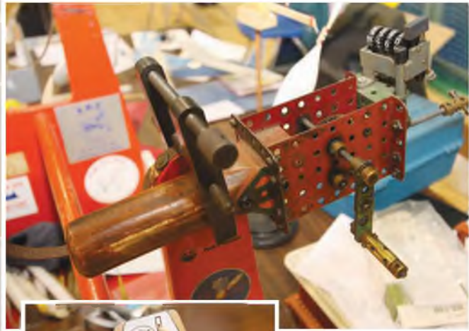
ABOVE: Meccano-based rubber winder. Love it. LEFT: Ski Hi Products Rubber Torque Meter http://www.skyhi.org.uk
