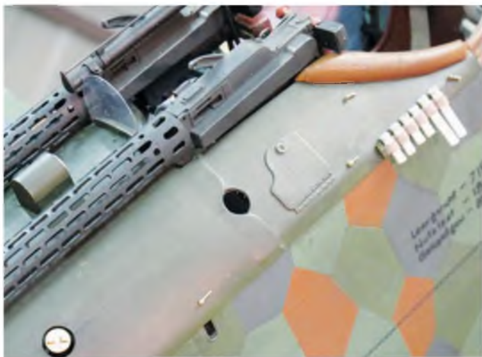
The external 'clutter' so common to aircraft of this era - including those Fokker nuts and flare cartridges.
