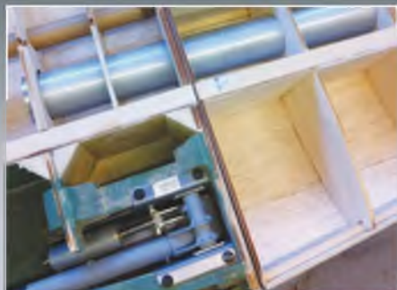
Rapid progress of the structure sees retracts, and wing joining tubes installed.
