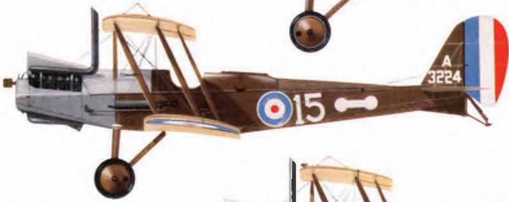
R.E.8, B5106 of No. 59 Sqn. R.A.F., Vert Galand, May 1918. Fitted with deep sump cowling and navigation lights
