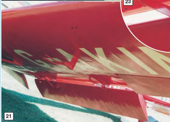
19 & 20: The wing flaps are fabric covered as seen here, revealing the rib positions. 21 & 22: Wing flaps viewed from the wing underside, showing the two hinges. 23: Close-up of one of the wing flap hinges. 24: Another view of the main undercarriage, also showing the underside of the engine cowl.
