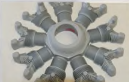
The resin cast dummy engine will hide the Zenoha G80 engine.
