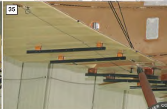
30, 31 & 32: General views showing the arrangement of bracing wires. 33: Aileron control cable runs externally from the fuselage, along the wing underside before feeding into the outer wing. 34: Another view of the fuselage centre section from the wing underside, showing the wing cut-outs to facilitate downward clear vision. 35: Bomb racks on the lower wing underside - four per wing panel. Note also, again, the aileron control run along the wing panel underside. 36: Detail of the main undercarriage rear strut mounting point. Note also the aileron control crank linked to its control cable. 37: Detail of the main undercarriage front strut mounting point. 38: Front profile of the main wheel. 39: A full view of the main undercarriage. 40: Mainwheel and axle close-up.
