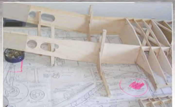
Like Graham Smith's original, Peter Shaw elected to build the wing as a one-piece structure. Here, the mainspar centre section is prepared, prior to laying down the left hand wing panel.
