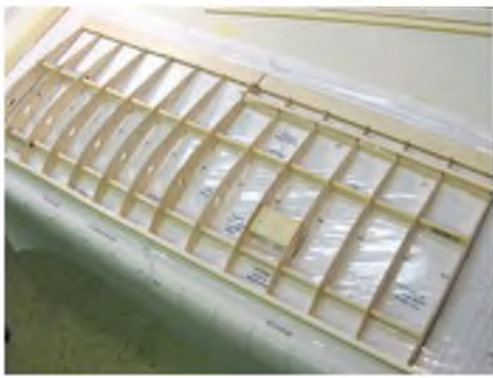
The hardest part about building these under camber wings is probably sliding the ribs onto the spars before pinning it all down to the board.
