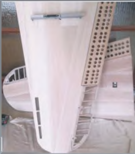
Wing outer panels structure completed and ready for finishing.
