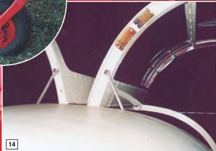
11-13: The cockpit/passenger cabin is a prominent feature of the Myles Messenger, so needs much attention. These views show the individual glazed panels. 14: Detail of the hinges of the cockpit hatches that hinge upwards. 15: The tailwheel unit. 16 & 17: Two views of the engine cowling showing panel lines and air intakes. 18: Profile of the propeller spinner.
