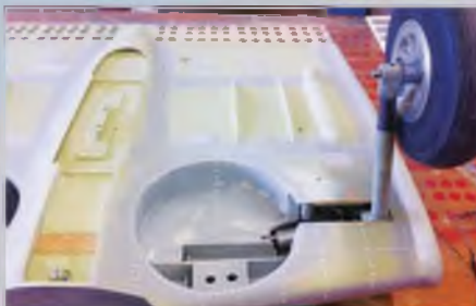
Application of rivets by use of glue droplets commences on the wings.
