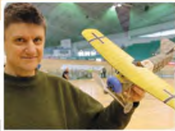
ABOVE: Peter Fardell's new Fokker E.V 20.5" span, weighs 40 grams. RIGHT: Peter's Fokker E.V was made from the Aerowekes kit. 2 loops of 1/8" rubber for power.
