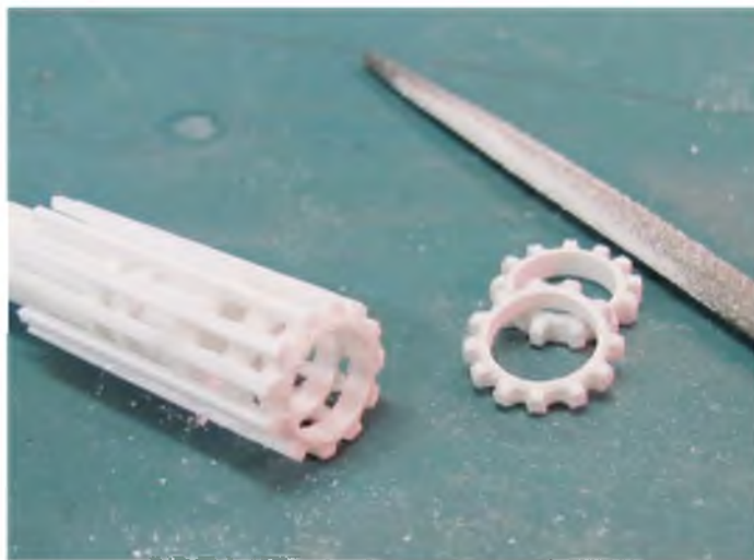
How the castellated nuts are made as a strip and cut off as required. Definitely easier than trying to make each one separately.
