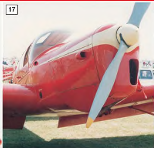
11-13: The cockpit/passenger cabin is a prominent feature of the Myles Messenger, so needs much attention. These views show the individual glazed panels. 14: Detail of the hinges of the cockpit hatches that hinge upwards. 15: The tailwheel unit. 16 & 17: Two views of the engine cowling showing panel lines and air intakes. 18: Profile of the propeller spinner.
