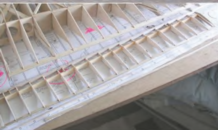
Close-up of one of the flaps, which, like the full size, will be fabric covered - the rib spacing needs to be as per full size.
