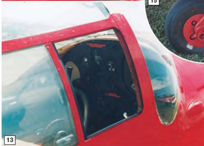
11-13: The cockpit/passenger cabin is a prominent feature of the Myles Messenger, so needs much attention. These views show the individual glazed panels. 14: Detail of the hinges of the cockpit hatches that hinge upwards. 15: The tailwheel unit. 16 & 17: Two views of the engine cowling showing panel lines and air intakes. 18: Profile of the propeller spinner.
