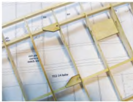
The servo plate fits into the rib slots and strut mounts glue to both rib and spar.
