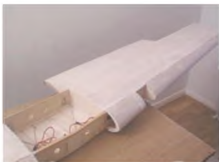
ABOVE LEFT: The left wing panel with plywood leading edge rolled around the wing ribs and fully skinned.
