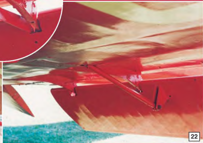
19 & 20: The wing flaps are fabric covered as seen here, revealing the rib positions. 21 & 22: Wing flaps viewed from the wing underside, showing the two hinges. 23: Close-up of one of the wing flap hinges. 24: Another view of the main undercarriage, also showing the underside of the engine cowl.
